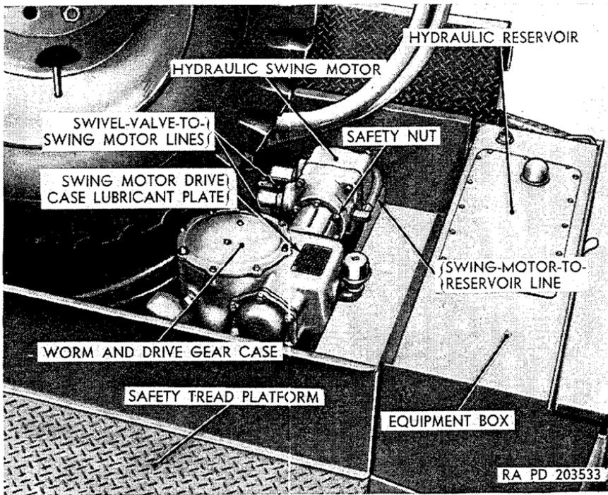
Figure 85. Crane hydraulic swing motor (M246).
