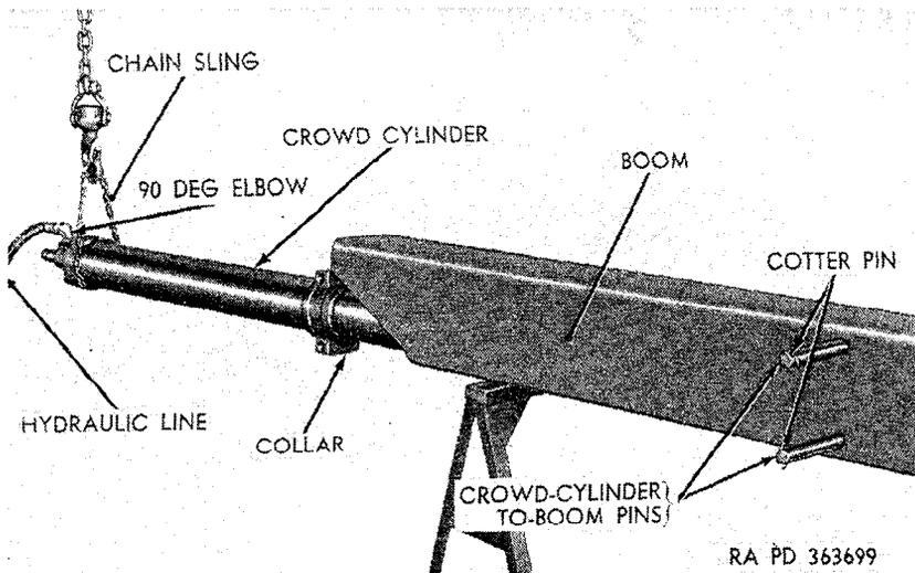
Figure 306. Removing boom crowd cylinder from boom M62 and M246.
