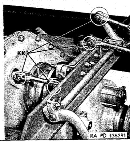
Figure 110. Localized lubrication points (BB-KK).
