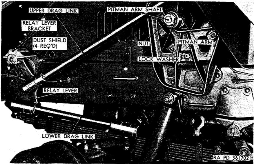
Figure 261. Steering linkage installed on vehicle under left front fender.
