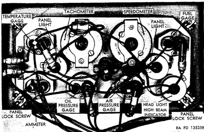
Figure 189. View of back side of instrument cluster.
