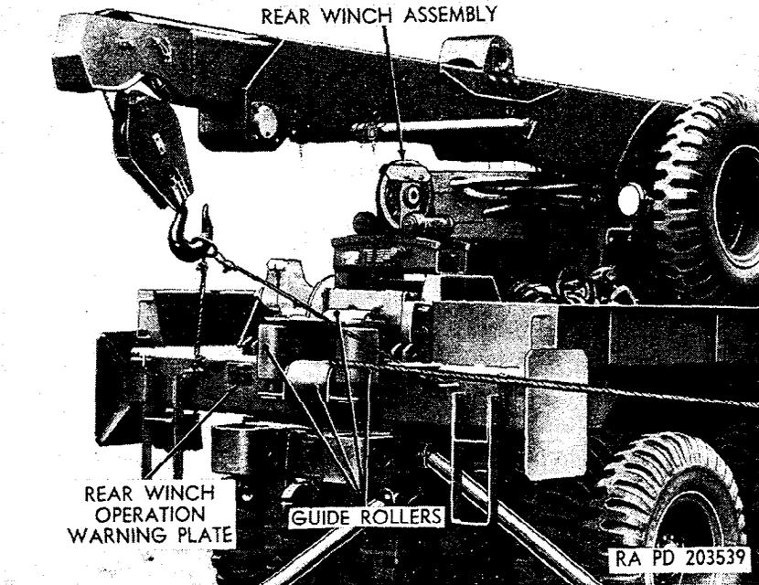
Figure 74. Right rear view of rear winch mounted on vehicle.
