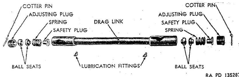
Figure 268. Drag link assembly—exploded view.
