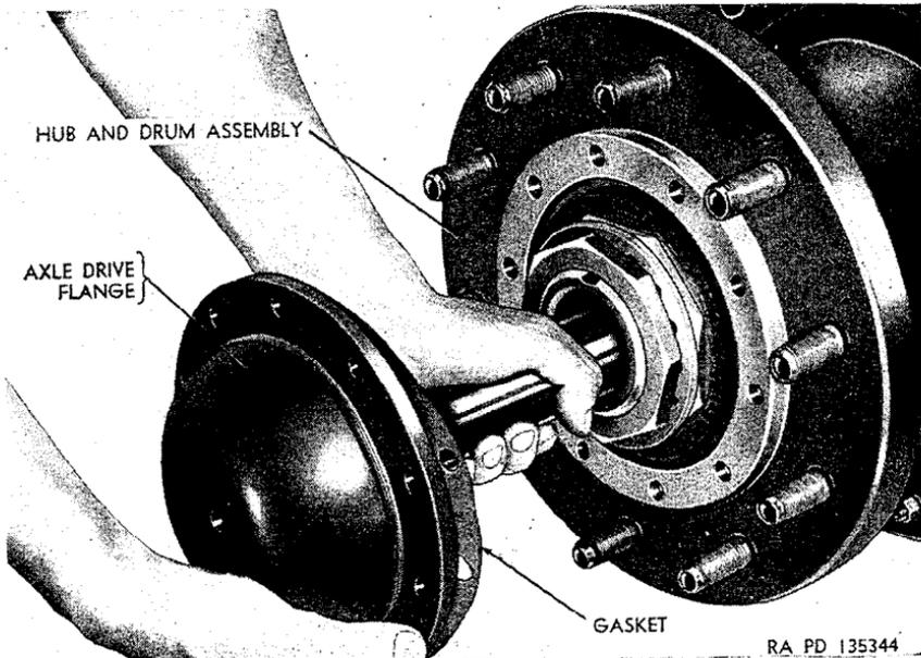
Figure 229. Removing rear axle shaft.
