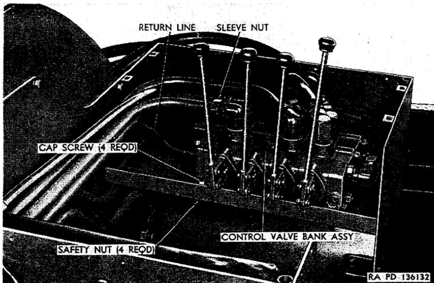
Figure 292. Rear view of operator's compartment and control valve bank assembly with cover removed M62.
