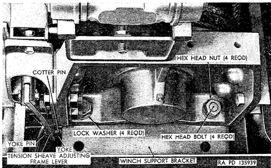
Figure 279. Top view of right end of rear winch—installed.
