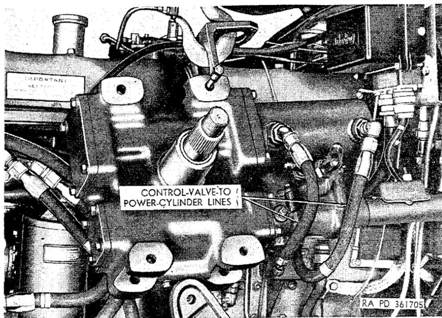
Figure 266. Removing steering gear.
