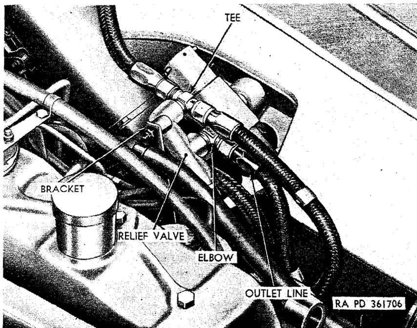
Figure 267. Top right view of relief valve installed.
