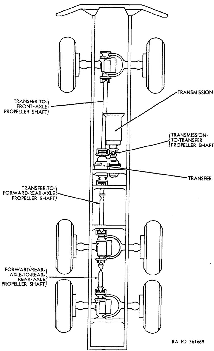
Figure 213. Diagram of axle driving propeller shafts.
