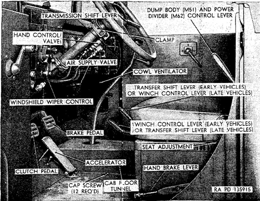
Figure 67. Driver's compartment—left side view.
