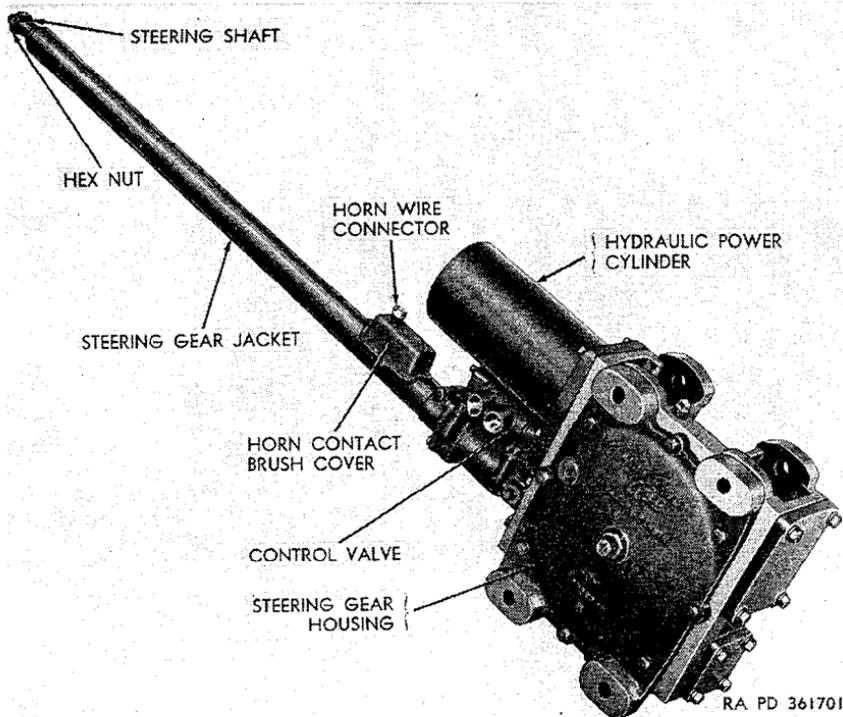
Figure 260. Right side view of steering gear removed from vehicle.
