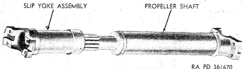
Figure 214. Propeller shaft assembly.
