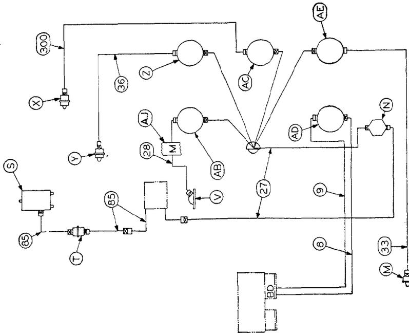
Figure 190. Diagram of gage and sending unit electrical circuits.
