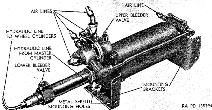
Figure 238. Air-hydraulic cylinder.
