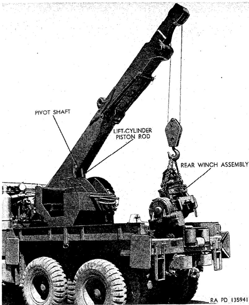
Figure 280. Removing rear winch assembly using wrecker crane.
