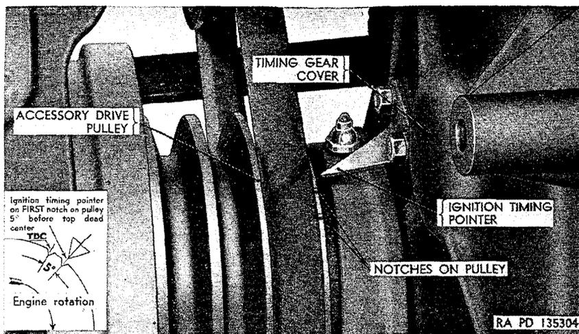
Figure 128. Ignition timing indicator.
