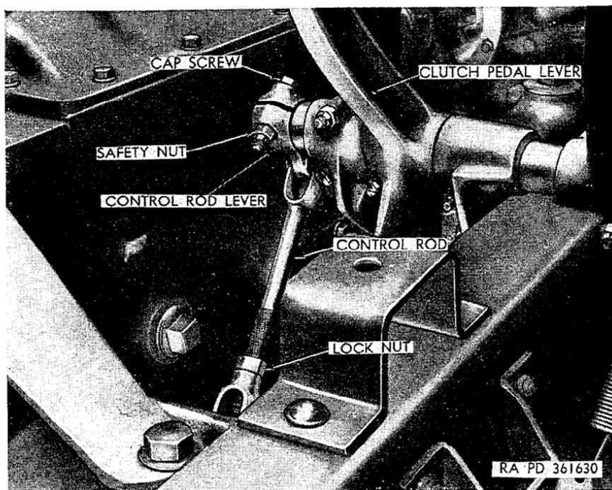
Figure 143. Left front view of clutch pedal lever and control rod.
