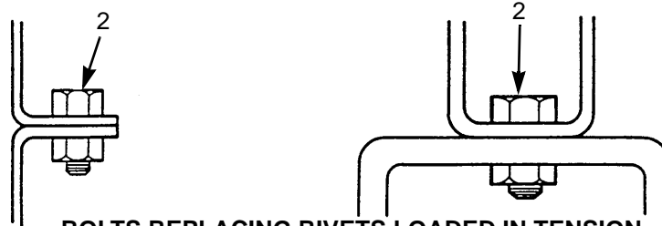
BOLTS REPLACING RIVETS LOADED IN TENSION
