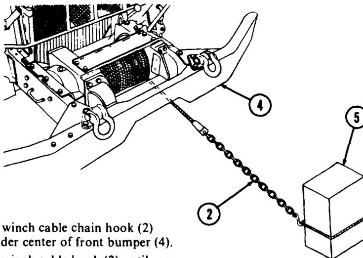
(6) Pull winch cable chain hook (2) down and under center of front bumper (4).
