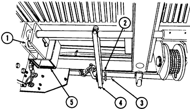
(a) Remove locking pin (3) and push handle (4) down to pull latch (1) from side rack posts (5).
