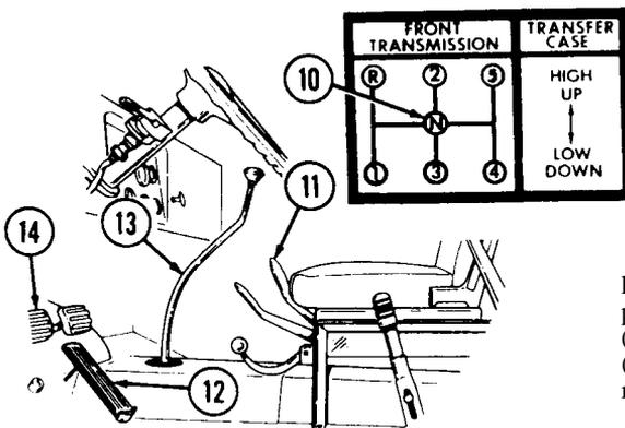
(1) Depress clutch pedal (14). Lift hinged locking plate on floorboard and place winch control lever (11) in "L" (low) position. Make sure gearshift lever (13) is in "N" (neutral) position (10) and release clutch pedal (14).
