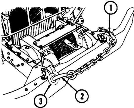
(5) Unhook winch cable chain hook (2) from right lifting shackle (3) and pass hook through left lifting shackle (1).
