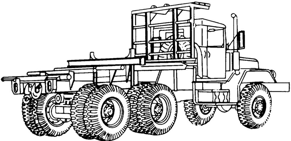
**5-TON, 6X6, BOLSTER LOGGING TRUCK W/W (M815)
