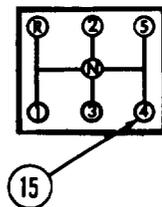
(d) Move gearshift lever (10) to "4" (fourth) gear (15).
