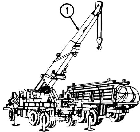
(1) Use crane (1) to unload class 60 bridge sections.
