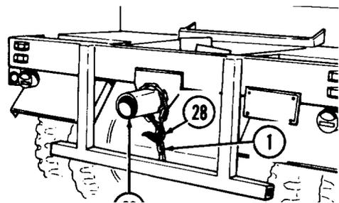
(12) Unhook winch cable chain hook (28) from cable chain (1) and free chain from fifth wheel (23).
