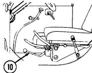
9 Airbrake hand control lever is used to control braking on a towed vehicle or semitrailer independently. When moved down, applies brakes; when moved up, releases brakes.
