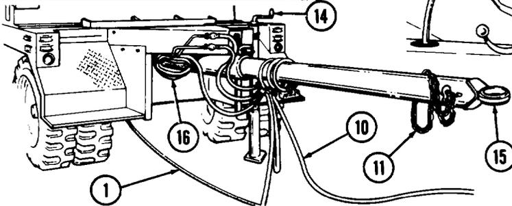
(4) Turn landing leg hand crank (14) clockwise until bolster trailer lunette (15) is free of bolster truck pintle (8).
