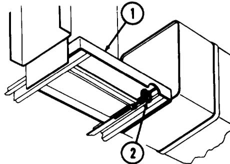
**b. Service.** Open draincock (2) after each day's operations and allow all moisture to escape. Close draincock (2) securely.
