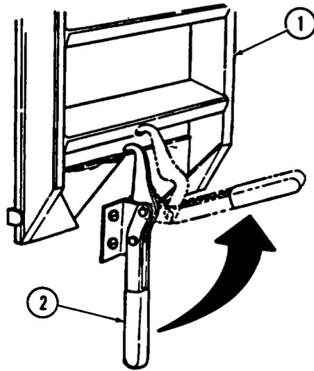
(b) Lift ladder (1) up and out to remove from rear door ladder mounting racks.
