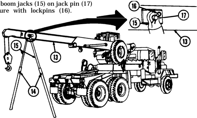
(r) Move hoist lever (11) to DOWN position and crowd lever (12) to EXTEND position to extend boom (13) all the way
