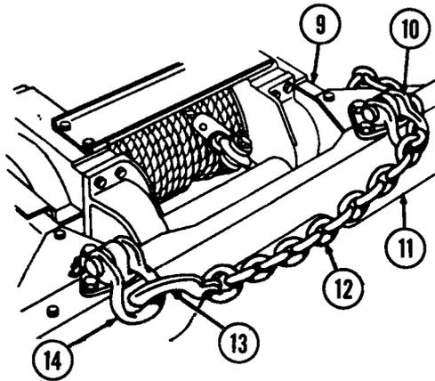
(2) On winches with level wind, pull cable chain (12) up through the space between the bumper (11) and winch on the left side. Wind cable chain around back of the level winding frame, then across the front so the chain hook (13) can be attached to the left side of the level winding frame.
