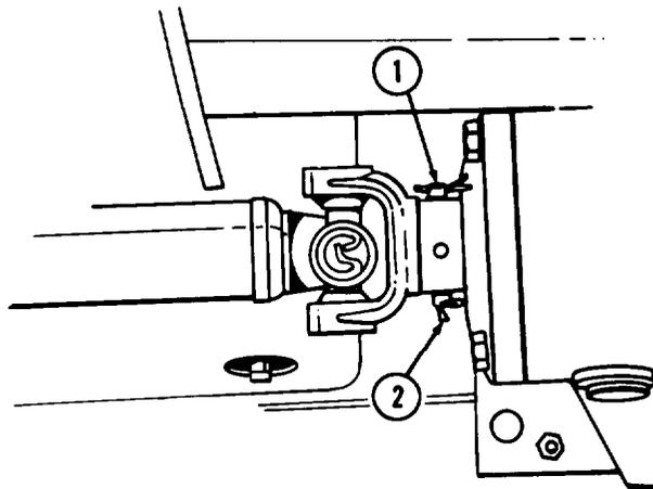
**a. General.** An aluminum shearpin (1) connects the universal joint yoke and front winch drive shaft. The shearpin (1) is designed to break whenever the winch is overloaded and is retained with cotter pins (2).
