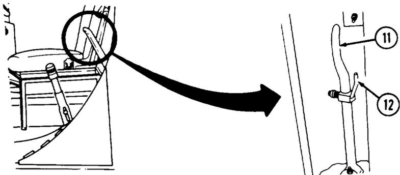
11 Power divider control lever is used to power hydraulic crane or rear winch.
