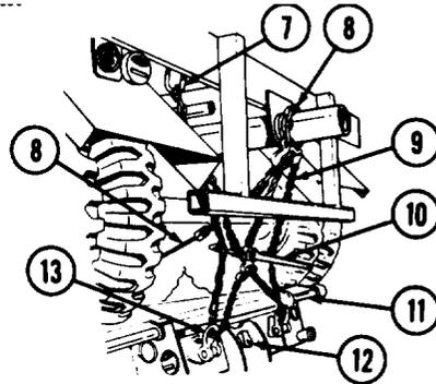
(5) Remove chain binder (10) and tiedown chain (9) at front of bolster trailer (4).
