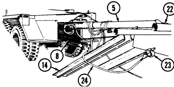
(6) Remove air hoses (24) from stowed position and between dual wheels of bolster trailer (4) and position along sides of bolster truck.
