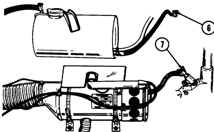
(2) Make certain both coolant shutof valves (6) and (7) are open (turned counterclockwise).
