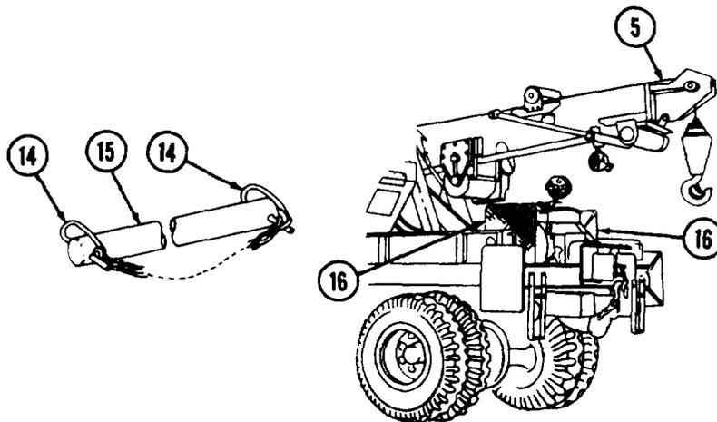
(a) Remove base plates (16) from rear winch
