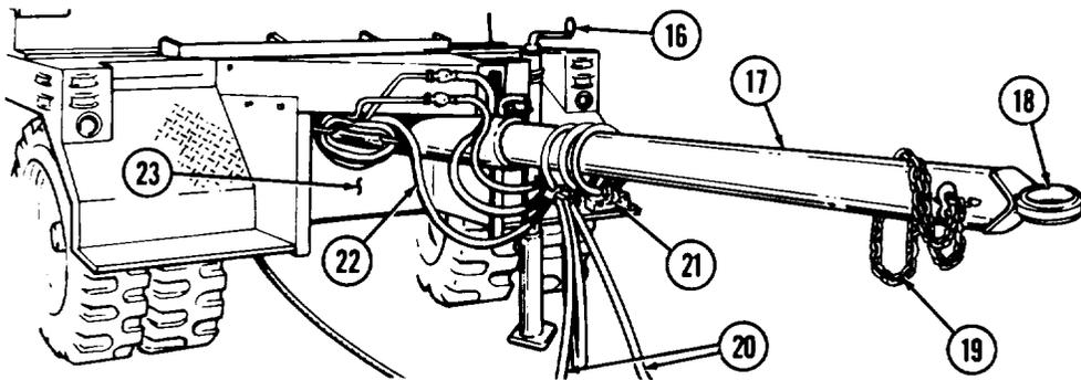
(19) Install intervehicular electrical cable (22) and two air hoses (20) in the front three retaining rings (21) on reach (17). Install electrical cable (22) in electrical connector (25) above the bolster truck pintle.
