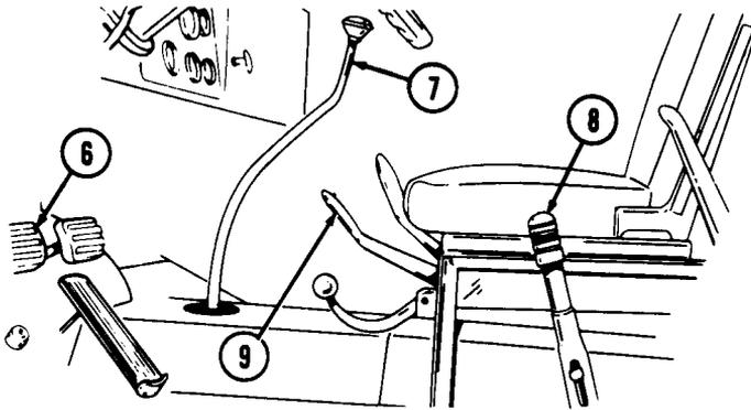
(5) Depress clutch pedal (6) of towed vehicle and place gearshift lever (7) and transfer lever (9) in neutral position. Release parking brake lever (8) of towed vehicle.
