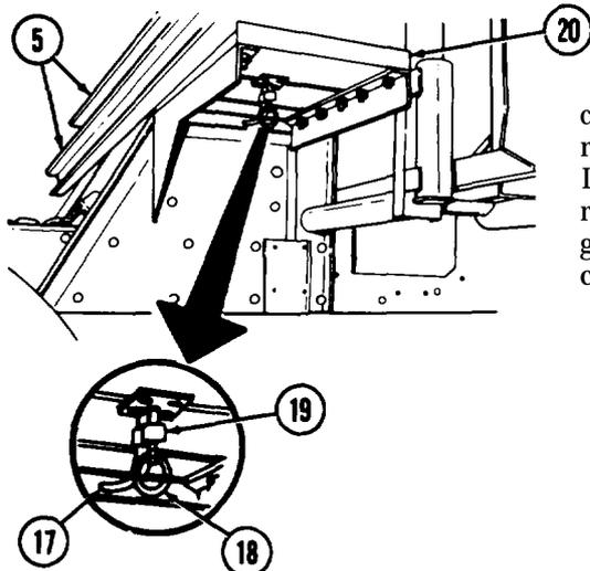
(26) Remove ramps (5) and place on catwalk (20) over midships winch. Secure ramps (5) in stowed position by pushing L-bolts (19) up through retaining slots in ramps (5), turning L-bolts (19) 90 degrees, grasping ring (18), and turning handle (17) clockwise to tighten.
