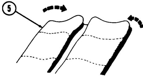
(6) Fold the side with three folds over the side with four folds.
