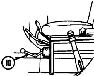
(g) Move transfer power takeoff lever (10) to disengage position.
