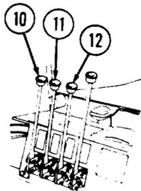
(p) Move boom lever (10) to DOWN position to lower boom (13) all the way.
