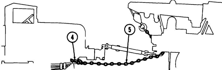
(3) Connect airbrake system of towing vehicle to intervehicular couplings located under front fenders of vehicle to be towed.
