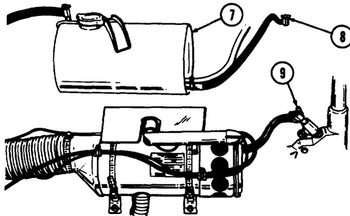
(1) Make sure coolant shutoff valves on engine water manifold (9) and engine oil cooler housing (8) are in fully opened (counterclockwise) position, and that shutoff valve in engine coolant heater box is in (counterclockwise) fully opened position.
