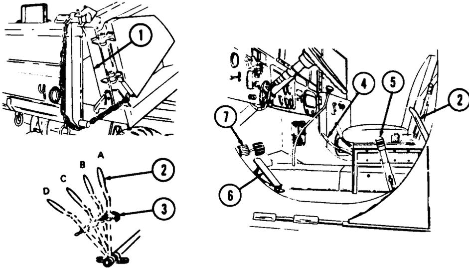
(14) When dump body is raised to desired height, move dump body control lever (2) back to position "C" to stop and hold dump body.
