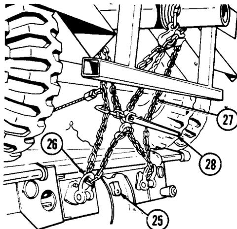
(20) Install bolster trailer lunette (18) on bolster truck pintle. Close pintle and install cotter pin to secure pintle in locked position. Install safety chain (19) attached to reach (17) near lunette (18) to towing shackles (26) of bolster truck.
