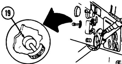
(g) Move hand throttle (19) to return engine speed to idle. Shut down engine (refer to paragraph 2-16).
