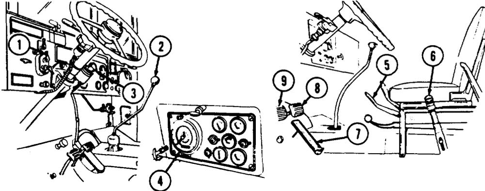
e. Depress service brake pedal (8), release parking brake lever (6), and release service brake pedal (8).
