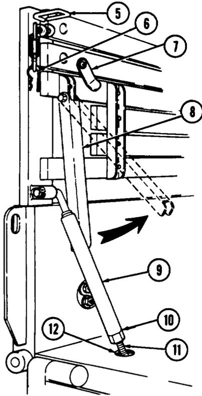
(3) On dropside trucks, install troop seat locking rods (9) in hole (12) near tailgate. Locking rod (9) can be shortened or lengthened. To adjust locking rod:
