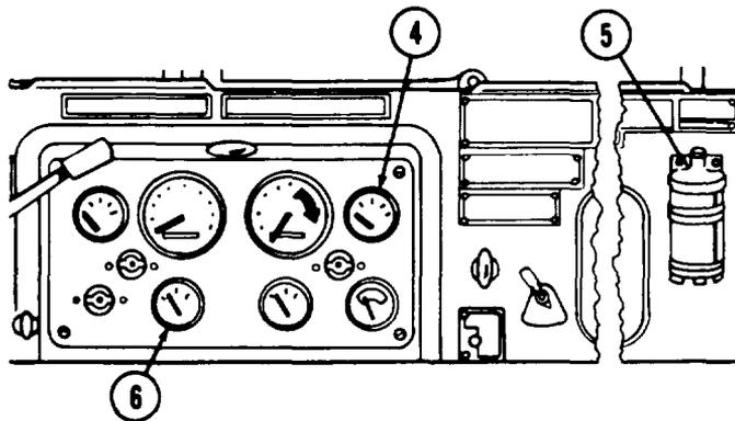
(3) Frequently check temperature gage (4) and oil pressure gage (6). Engine is overheating if one or more of the following conditions exist:
