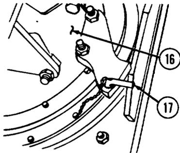
(e) Install pivot post lockpin (17) in crane pivot post (16).
