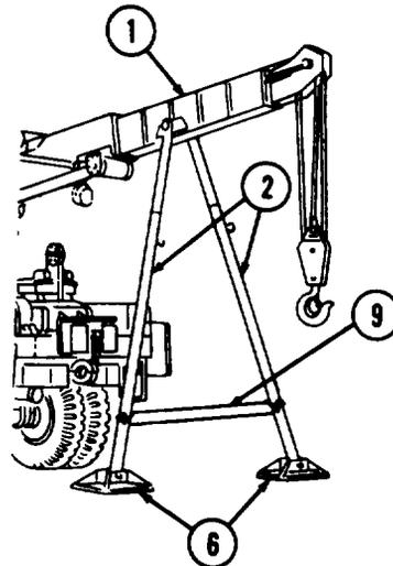
(g) Position base plates (6) to boom jacks (2) and secure with L-shaped pins (7) and lockpins (11).
