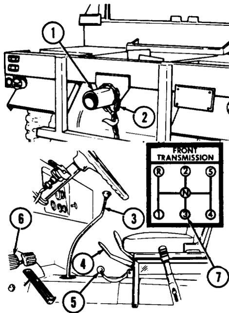
(16) Stop rewind as cable chain (2) nears midships winch by disengaging engine clutch (6) and shifting transfer power takeoff control lever (5) down to disengaged position. Place gearshift lever (3) in "N" (neutral) position and release clutch pedal (6). Attach winch cable (2) to fifth wheel base.
