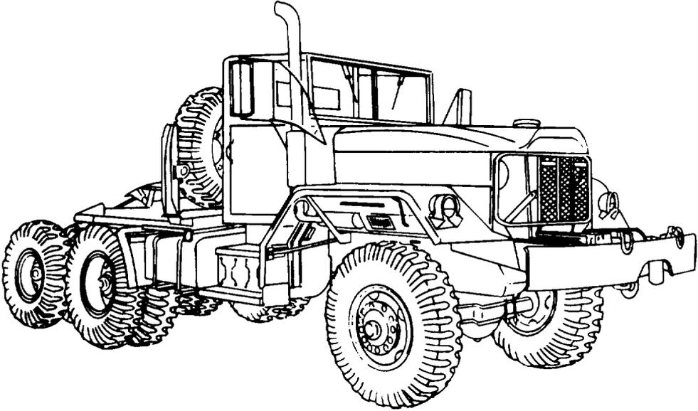
**5-TON, 6X6, TRACTOR TRUCK WO/W AND W/W (M818)
