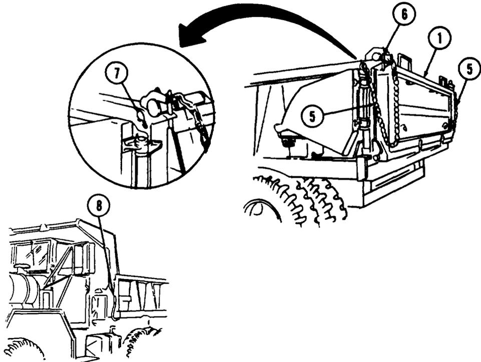
(c) Lock chains (5) in place by securing to locking slots (2).
