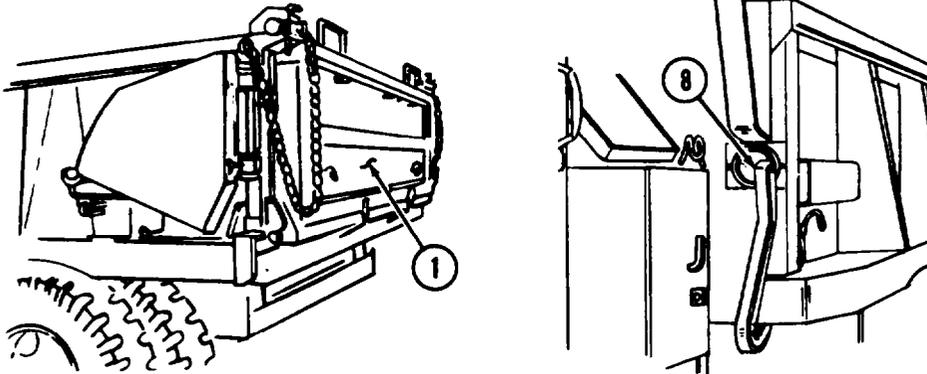
(25) Move control rod hand lever (8) up and back to lock tailgate(1) in closed position.
