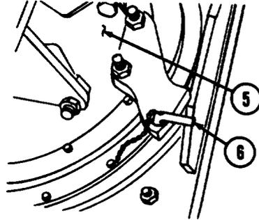
(b) Install pivot post lockpin (6) in pivot post (5).
