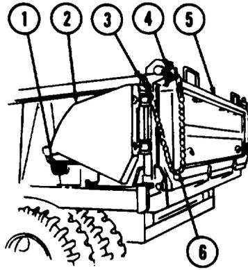
(3) To rig tailgate (5) to swing open at top for rocker-type operation, follow these procedures for both ends of tailgate (5).
