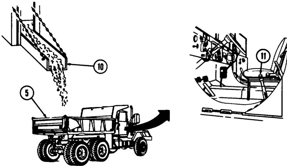
(a) Start engine (refer to paragraphs 2-12 and 2-13). Move truck so dump body is aligned directly under loading vehicle (10).
