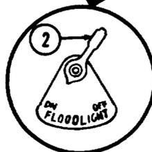
(11) For night operation, move main floodlight control switch (2) to ON position (if tactical situation permits).
