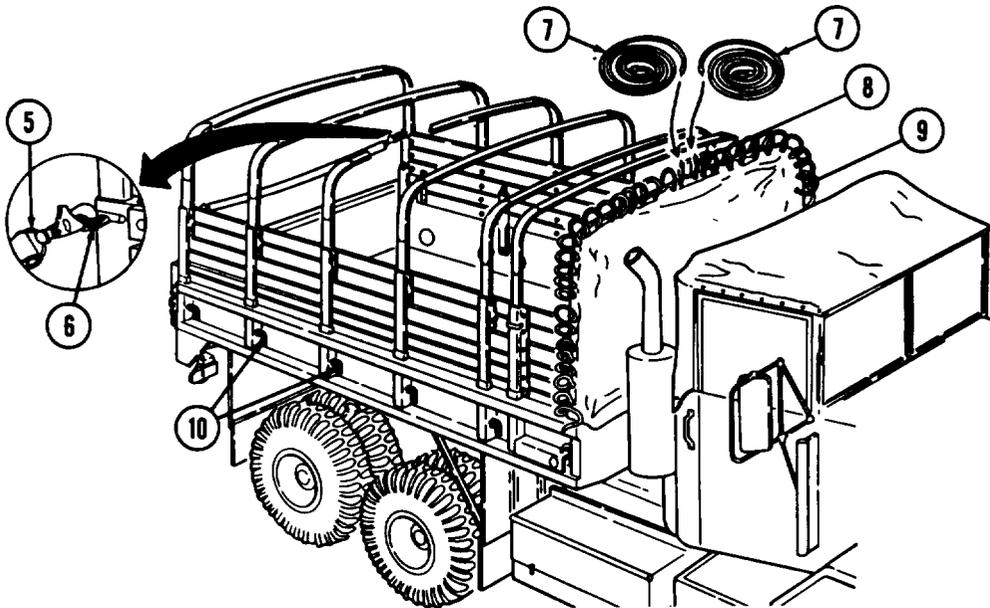
(4) Secure rope end on each side of vehicle to lashing hooks (10).
