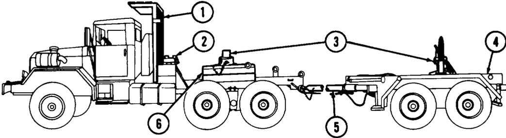
**a. General.** M815 bolster trucks are equipped with a cab protector (1), midships winch (2), bolster assembly (3), and fifth wheel assembly (6). M796 bolster trailer (4) has an adjustable reach (5) with safety chains. Truck and trailer combination is designed to haul utility poles, logs, or bridge sections. The trailer is carried on the truck when not in use. More information for trailer operation is contained in TM 9-2330-287-14.
