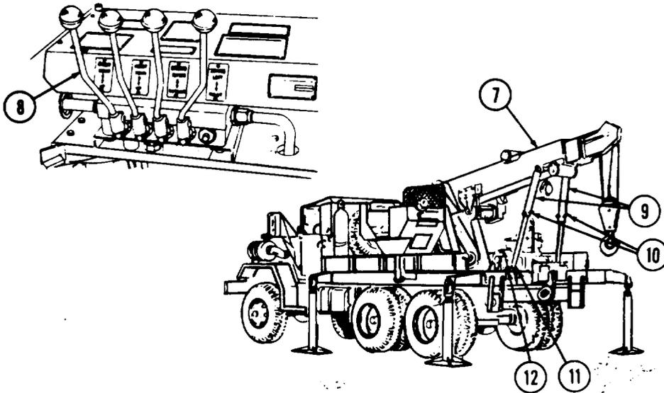
(s) Remove T-shaped pins ( 10 ) in braces (9). Raise or lower boom to remove pressure on pins.
