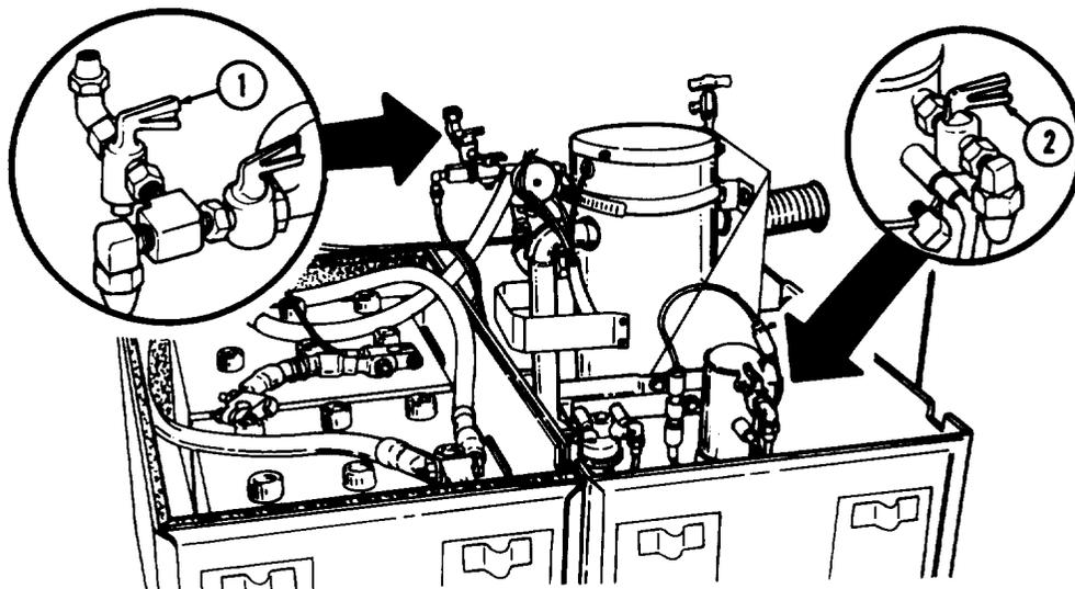
(3) Open fuel shutoff valve (1) for coolant heater by turning counterclockwise. Open valve (2) at coolant heater fuel pump in the same way.
