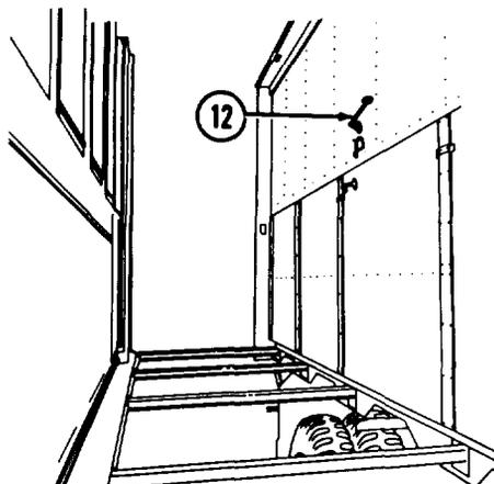
(8) Turn hinged roof lock handle (12) counterclockwise to release panel locks.
