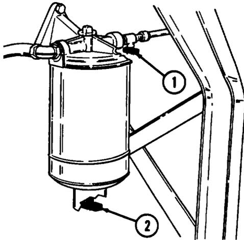
(c) Open draincock (2), at bottom of fuel filter/water separator, and allow approximately one pint (0.473 l) of liquid to drain off into a container.
