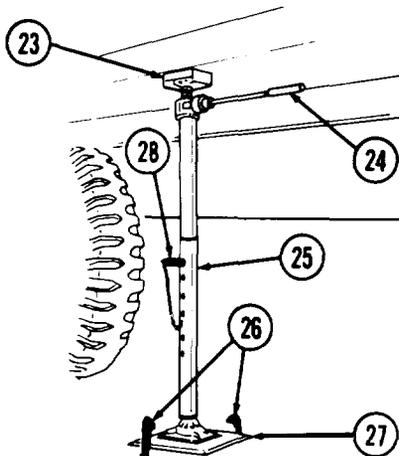
(22) Remove two jack spikes (26) from footpad (27) and install jack handle (24) in leveling jack (25). Rotate jack handle (24) clockwise until footpad (27) clears ground.
