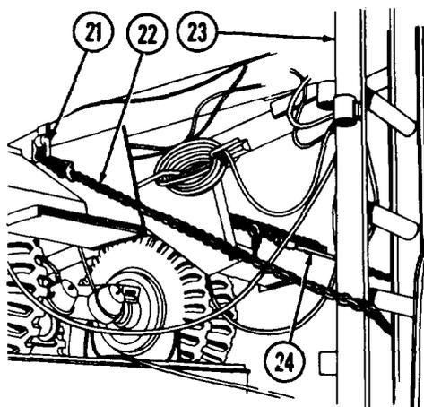
(27) Remove two tiedown chains (22) and two chain binders (24) from bolster trailer stowage compartment. Secure bolster trailer front to cab protector (23) with one tiedown chain (22) attached to front lifting shackles (21), then wrap chain (22) around cab protector (23). Tighten tiedown chain (22) with chain binder (24).
