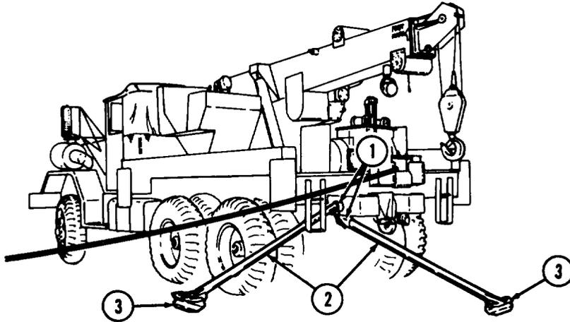
**(c)** For indirect pulls on left side, install chocks (2) in anchors (1) on left side frame. For right side pulls, install chocks in anchors on right side frame.
