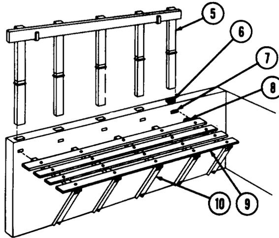
(1) Insert side racks (5) into slots (6) on dump body side walls.
