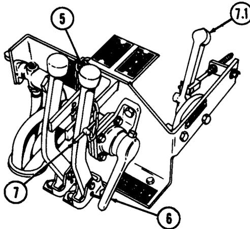
(3) Remove slack in winch cable chain (1) by moving winch shift lever (5) to WIND position.
