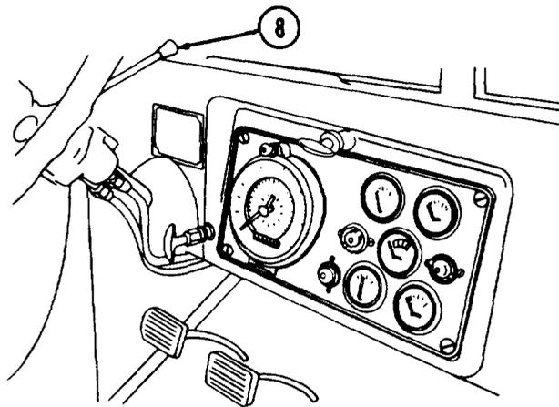
**(18)** Pull down on airbrake hand control lever (8) to check service airbrake system. Air should be heard passing through control valve.
