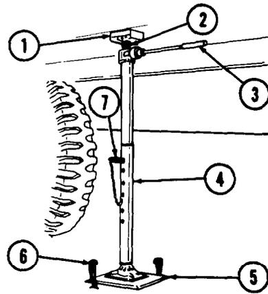
(3) Insert upper foot (2) of jack (4) into bracket (1). Install jack handle (3) and unscrew jack (4) until footpads (5) are in firm contact with ground. Anchor each jack footpad (5) with two jack spikes (6). Do not attempt to raise entire van off ground with leveling jacks.
