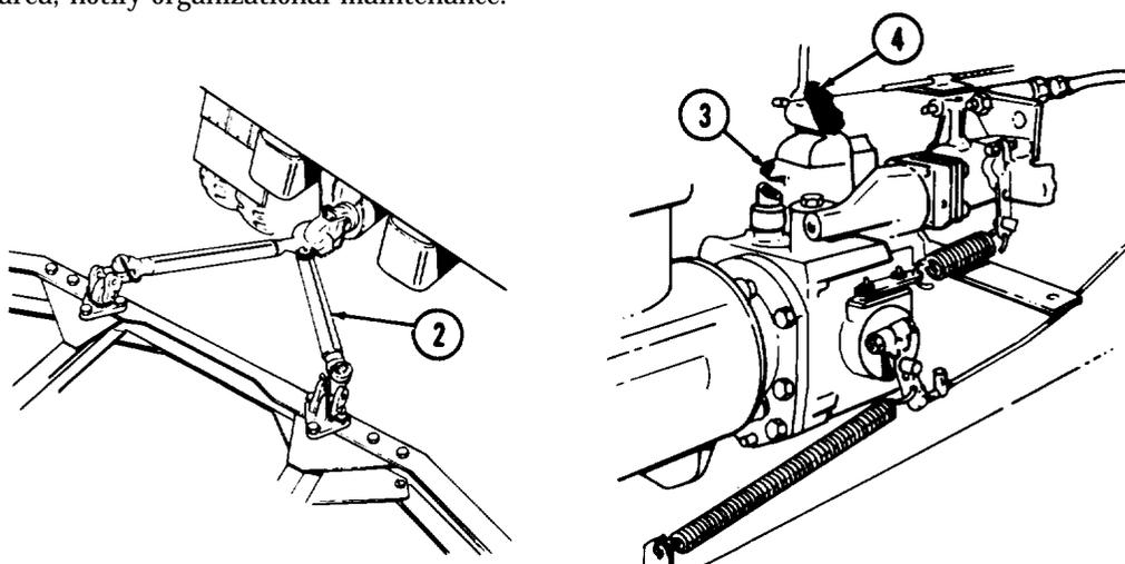
(15) Disconnect towbar (2) from towing and towed vehicles and stow.
