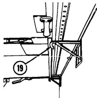
(10) Lift upon hinged roof panel (16) and turn swivel hooks (19) at right angles. Support hinged roof (16) on three swivel hooks (19).
