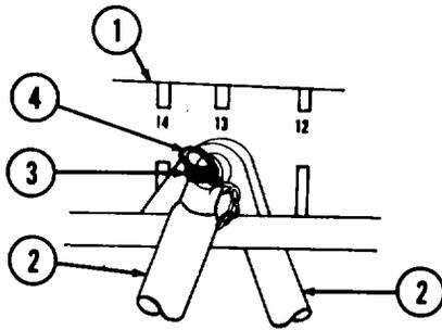
(e) Install boom jacks (2) on inner jack pin (3) and secure with lockpins (4). Lengthen or shorten boom jacks (2) by moving retaining pins (5) and lockpins, if needed.
