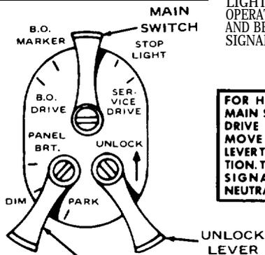
FOR HAZARD WARNING, MOVE MAIN SWITCH TO EITHER SERVICE DRIVE OR STOP LIGHT POSITION. MOVE TURN SIGNAL CONTROL LEVER TO HAZARD WARNING POSITION. TO DEACTIVATE, MOVE TURN SIGNAL CONTROL LEVER TO NEUTRAL POSITION.
