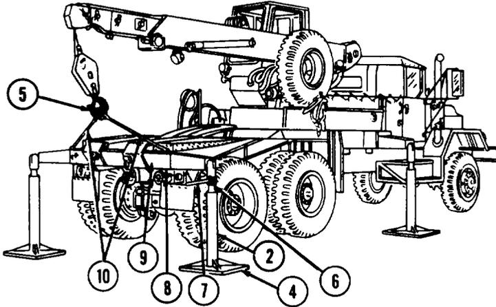
(b) Remove L-shaped pin (8), grasp outrigger base plate (4), and swing outrigger (2) down to touch ground.
