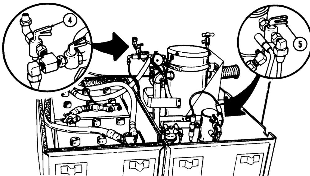
(1) Open fuel shutoff valves (4) and (5) by turning counterclockwise.
