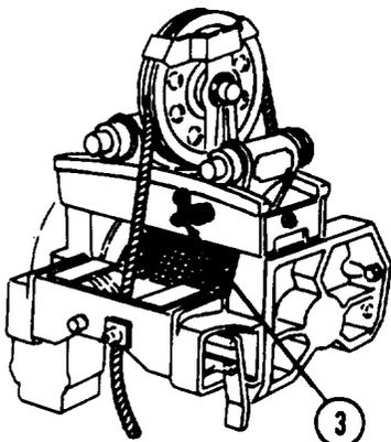
(13) Pull level wind knob (3), rotate 1/4 turn, and release.
