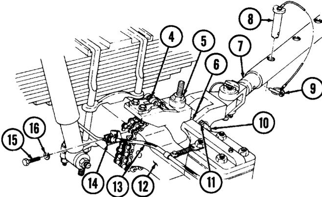
(f) Position clamp (6) against front axle (12) of disabled vehicle and wrap clamp chain (4) around axle and back up through clamp. Lock in place by turning tension adjusting nut (5) with wrench until securely tightened.
