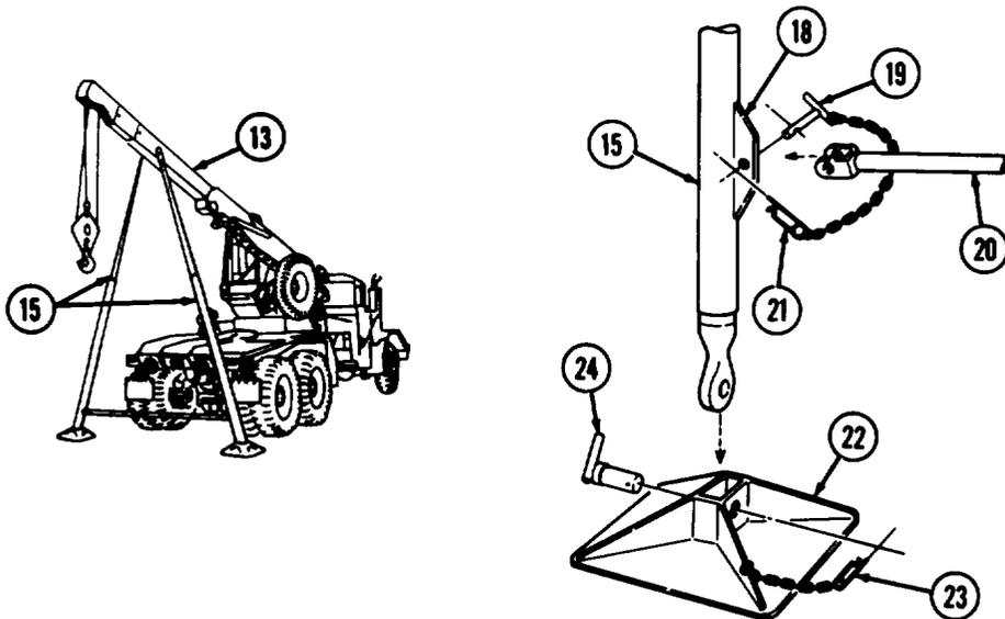
(t) Position base plates (22) on boom jacks (15) and secure with L-shaped pins (24) and lockpins (23).
