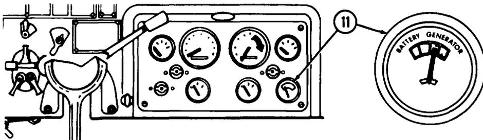
i. Observe battery-generator indicator (11) on slaved vehicle, If indicator (11) is not in green area, notify organizational maintenance.
