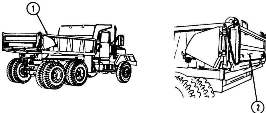
e. Unloading the Truck With Dump Body Down.
