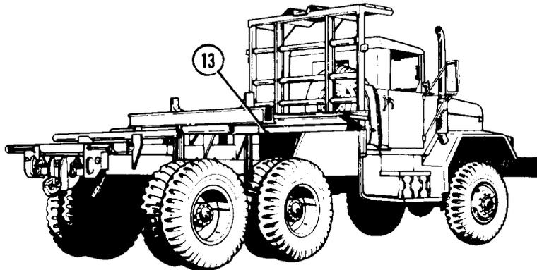
(2) The midships winch (13) and front winch can be used for loading and unloading. Controls for both winches are identical. Refer to paragraph 2-22 for front winch operation.
