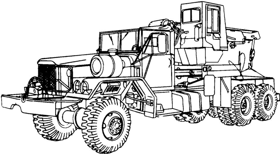
**5-TON, 6X6, TRACTOR WRECKER TRUCK W/W (M819)
