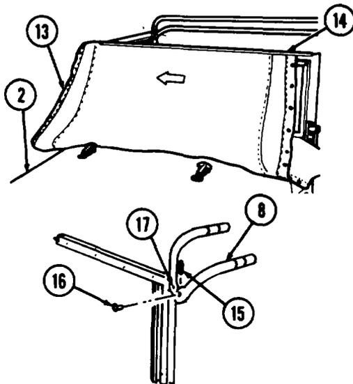
**i.** Pull cab top (13) towards rear of cab (12) over windshield (1), and crossbows (9) and (11). Place inner flap of cab top (13) between seats (10) and cab (12) wall.
