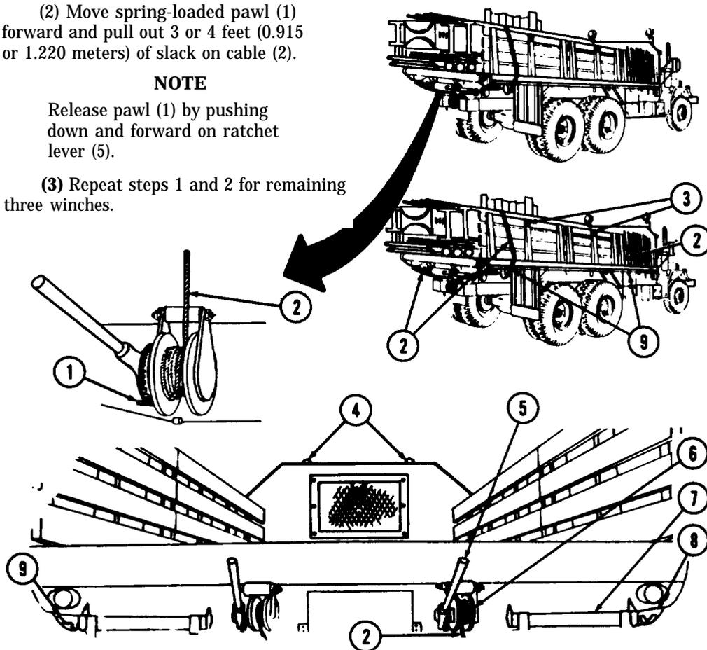
(4) Loosen and remove cables (2) from lashing hooks (10), lashing rings (3), and lashing rings (4).
