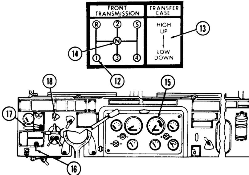
(7) Depress clutch pedal (11) of towed vehicle and place gearshift lever (6) in "1" (first) gear (12). Place transfer selector lever (8) up to HIGH position (13). Release parking brake lever (7) of towed vehicle.
