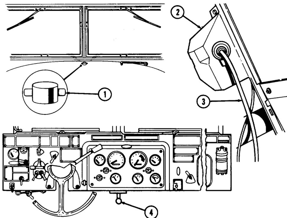
**a. General.** The windshield washer kit includes a hand pump (4) mounted under the instrument panel, a fluid reservoir (2) on right side of engine compartment, necessary tubing (3), and supports. A single nozzle (1) in front of windshield has two openings; one for each windshield section.
