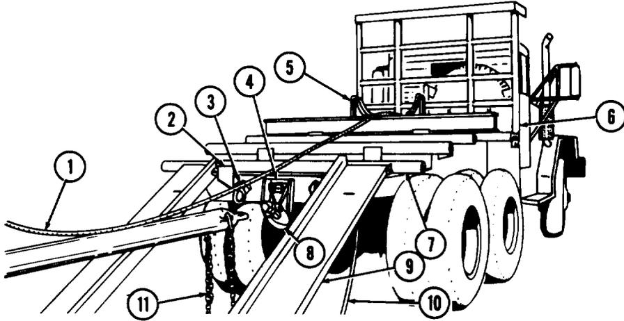
(1) Place bolster truck and trailer on level ground. Apply parking brake (13) and stop engine (refer to paragraph 2-16). Shorten reach as required [refer to c.(3) and c.(4) above].
