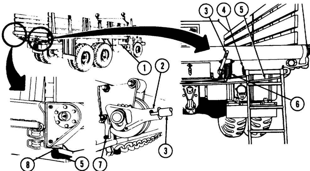
(1) Remove winch handle (3) from stowage compartment (1) and install in rear ratchet lever (2).
