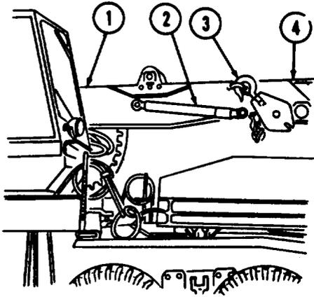
(a) When trailer is towed, stow shipper braces (2) on boom (1).
