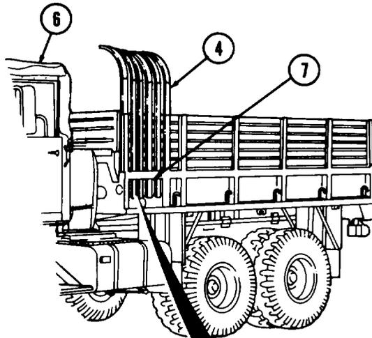
(16) Strap overhead crossbows (5) together and stow in storage area located under cargo body.
