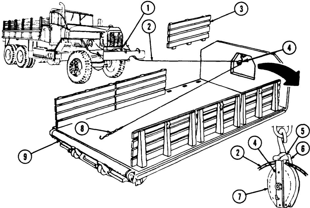
(7) Pull latch (5) down, swing bracket (6) to open position, and place winch cable (2) on sheave (7).
