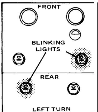
FOR TURN SIGNALS, MOVE MAIN SWITCH TO EITHER SERVICE DRIVE OR STOP LIGHT POSITION. MOVE TURN SIGNAL CONTROL LEVER UP FOR RIGHT TURN AND DOWN FOR LEFT TURN. MOVE TO NEUTRAL TO DEACTIVATE TURN SIGNALS.
