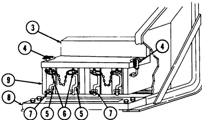
a. Unlatch two battery cover latches (4) and remove upper running board assembly (3).
