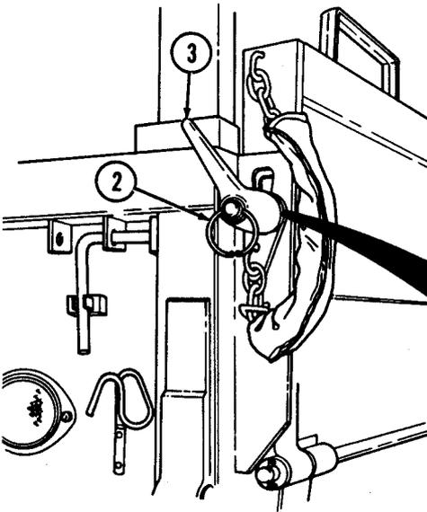
(3) On dropside trucks, turn locking handles (3) on sides of tailgate counterclockwise to loosen. Grasp ring (2) and twist to turn T-bolt (4) vertically up. Withdraw locking handle assembly. Do the same operation on the opposite end of tailgate.
