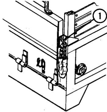
(1) Remove hooks (1) from retainer slots on both sides of tailgate.
