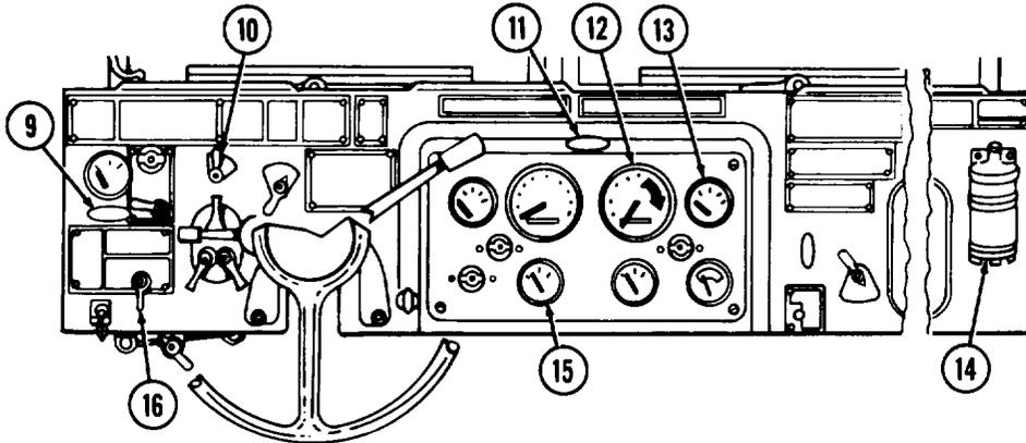
j. Place battery switch (10) in ON position,
