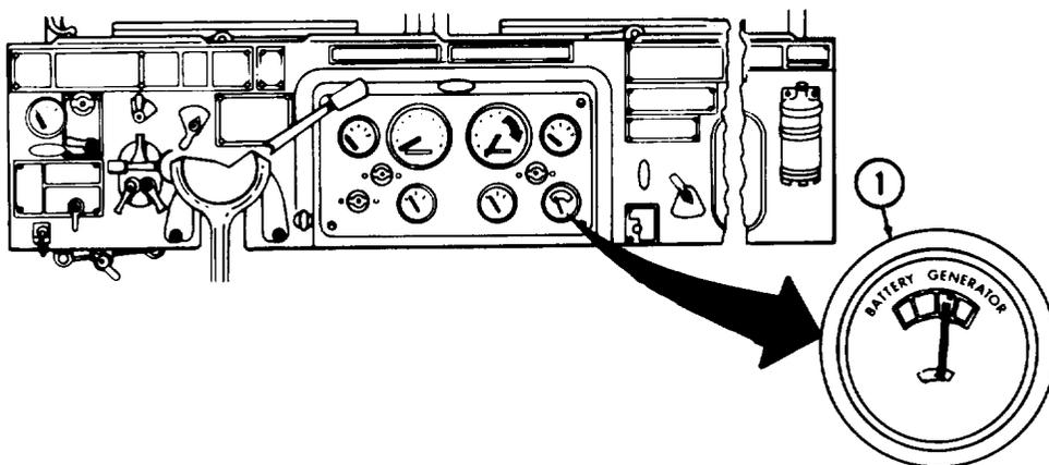
(14) Observe all instruments and allow engine to warm up. Check battery-generator indicator (1) to be sure alternator is producing current. If indicator (1) is in red or yellow area, notify organizational maintenance.
