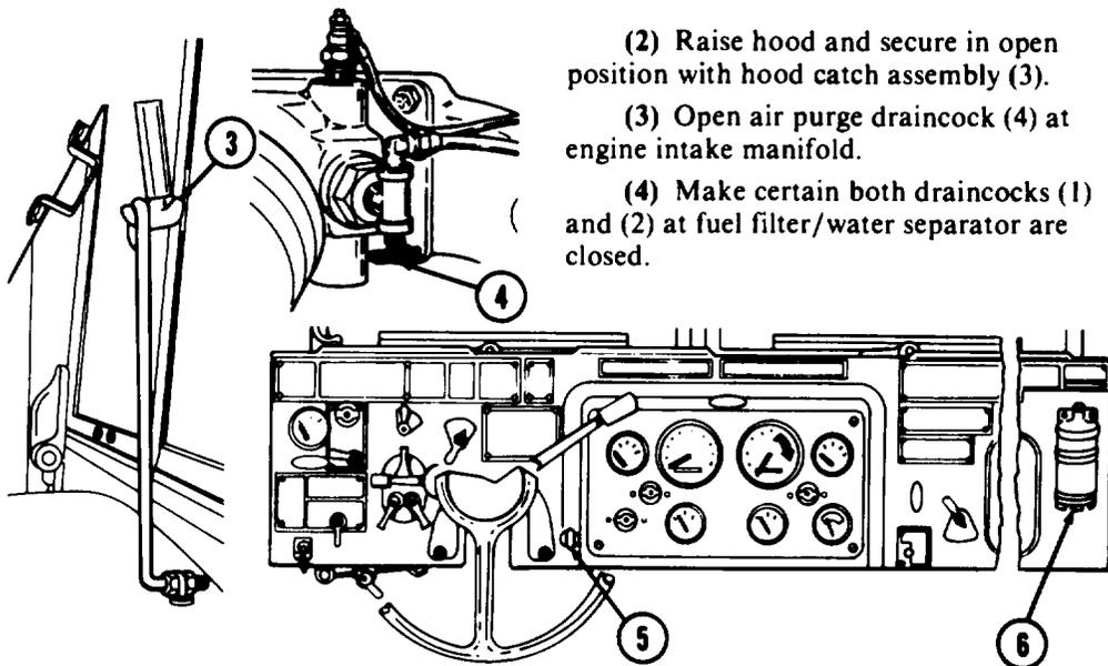
(2) Raise hood and secure in open position with hood catch assembly (3).
