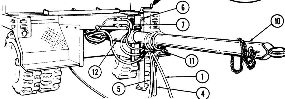
(3) Before extending or retracting trailer reach (10), disconnect brake air hoses (1) and (5) and electrical cable (4) from retaining rings (11) at rear of bolster truck.
