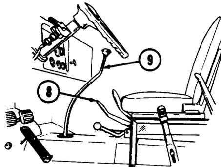
(2) Move gearshift lever (9) to "1" (first) gear (7).
