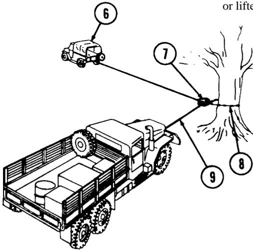
(8) If vehicle cannot be placed in direct line with load (6), attach snatch block (7) to winch cable (9) and secure with utility chain (8).
