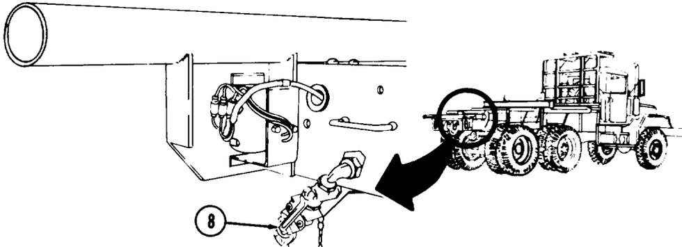
8 Air valve half couplings are used to connect air supply.
