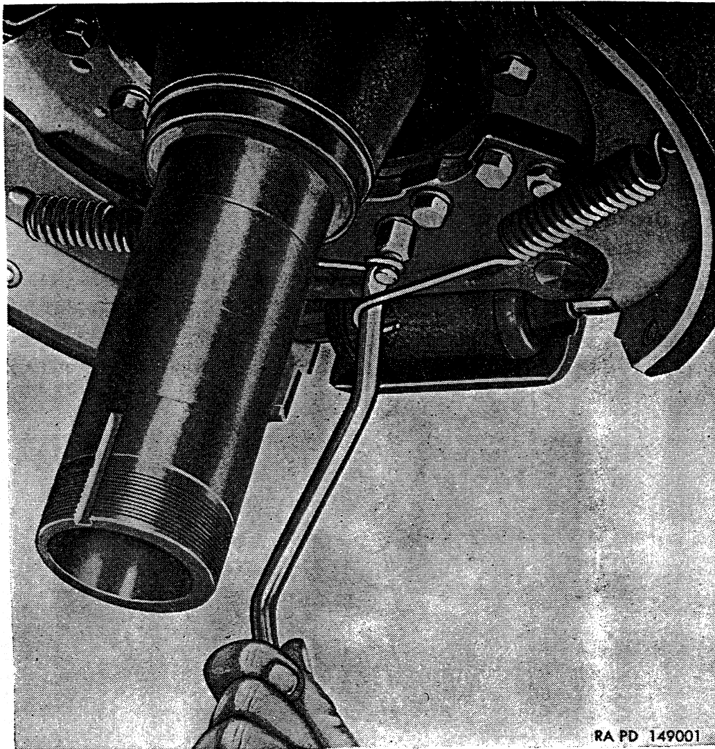
Figure 248. Installing brake shoe return springs, using remover and replacer B7950060.
