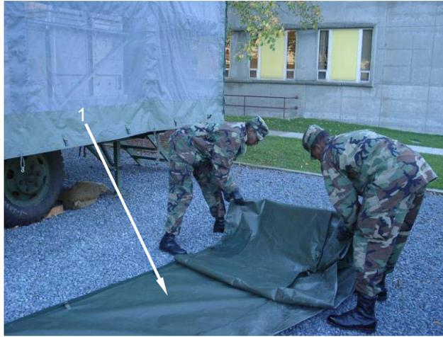
Remove side and end cover assemblies and screen assemblies (1), fold up and stow in cabinets (2).
