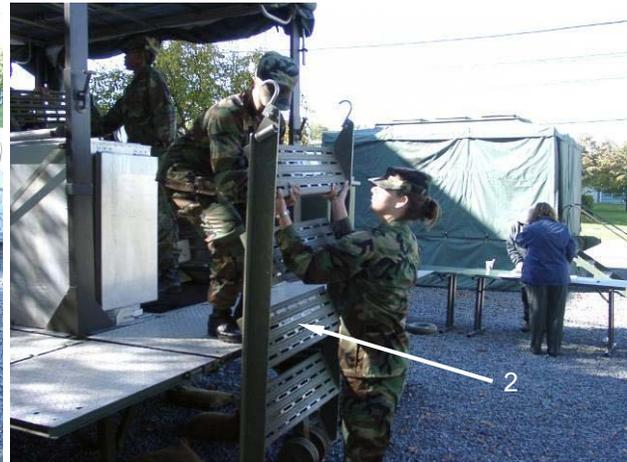
Install three ladders (1) and handrails (2) onto ramps at entry and exit. Engage the hooks (3) at the end of the ladder (1) into the holes (4) on the ramps (5). There are nine possible locations for the ladders (1). Install two handrails (2) on each ladder by engaging the ends of the handrails into the receptacles (6) in the ladder (1).
