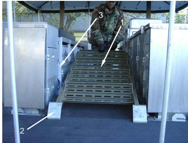
Slide ice chest (1) in temporarily so that it is flush with the end of the cabinets (2). Be sure that the handle of the ice chest does not interfere with the hole in the floor for the roof jack. Push the end of the ladder (3) so that it contacts the side of the ice chest (1). After positioning the ladder, remove the ice chest and set aside.
