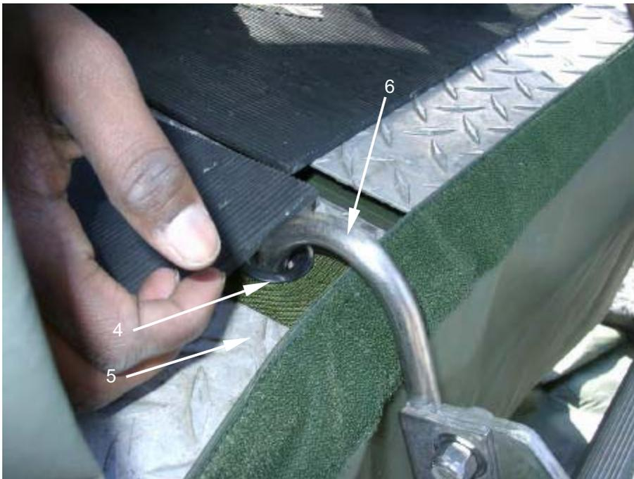
To install the left side section **(1)** of the cold weather skirt assembly, disengage all elastic cords with “S” hooks along the bottom of the side panels. Hold one end of the skirt in position to the left of the towing tongue in the front of the MKT. Engage the quick release clips **(2)** on the cold weather skirt to the side panels **(3)** of the MKT.
