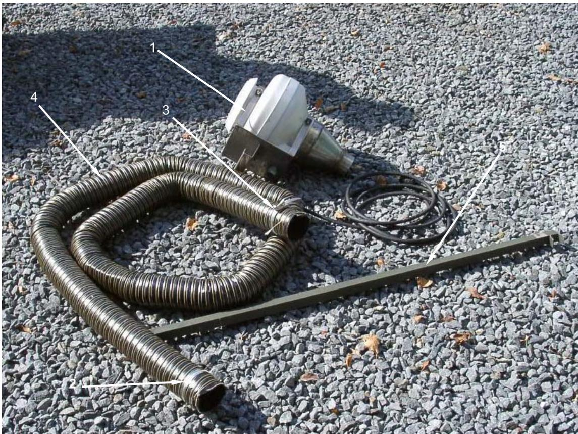
To install the exhaust fan assembly, first install the portable prop (1) on the upper MKT framework (2) by engaging the end of the prop with the tab shaped section (3) over the center frame member (4) between the first and second roof openings (5). Place the opposite end (6) of the prop over the lip (7) on the frame near the hand crank for the first roof opening. The prop (1) remains in place on the upper frame without the need for securing hardware.
