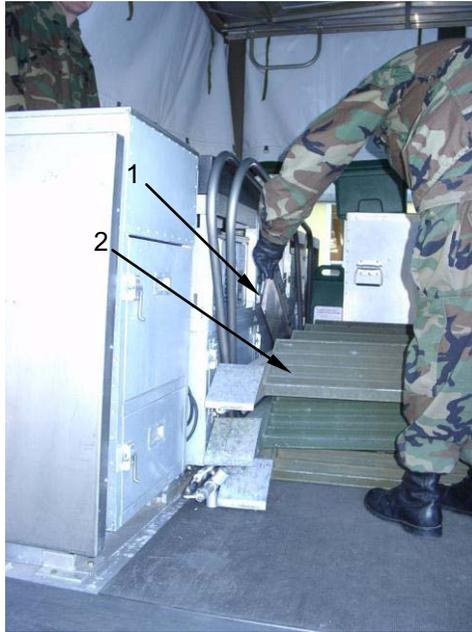
Stack five liquid dispensers (1) along the top of the burner rack (2) with the tops facing toward the center aisle.
