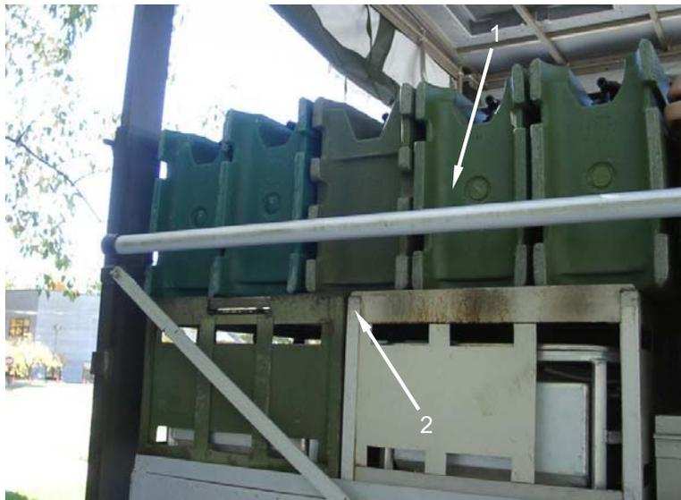
Place two insulated food containers (1), one cover facing up and the other with the cover facing down on top of the griddle (2). Place two liquid dispensers (3) on their side to the right of the two insulated food containers with the tops facing the center aisle. One of the cold weather skirts (4) will be placed on top of the insulated food containers and the liquid dispensers in a later step.
