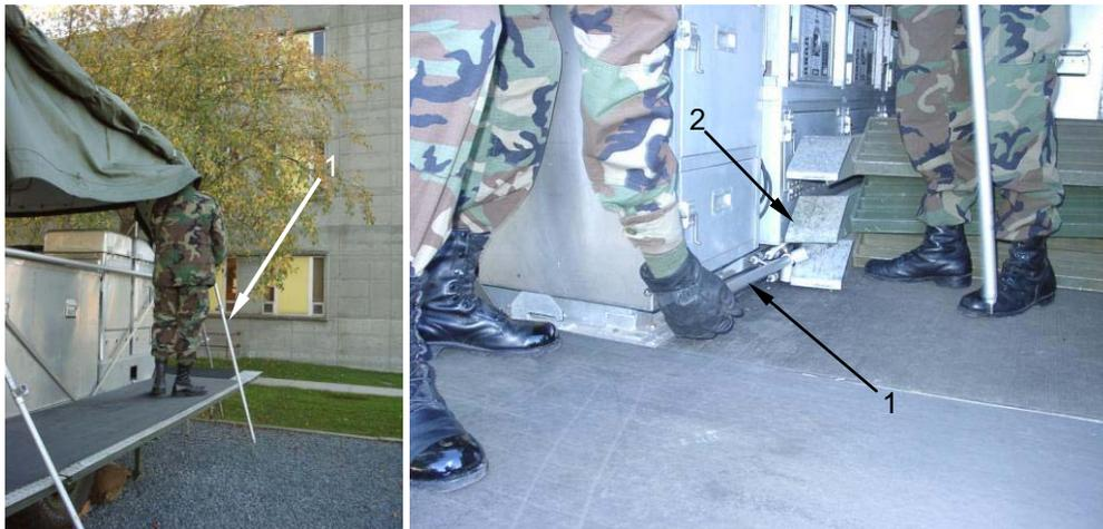
Stow ladder handrails (1) on the left and right side of the ladder (2) leaning against the fronts of the cabinets (3).
