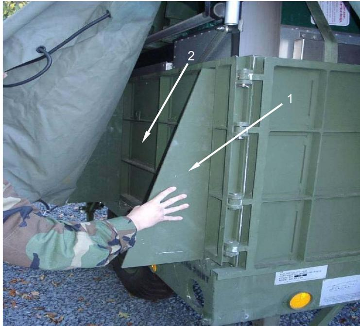
With one person at each corner holding side ramp so it will not fall, raise slide lock pins (1) to release corner ramps (2).
