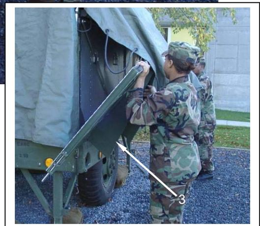
Retrieve the four corner struts (1) from their stowage location at the rear of the MKT. Install the corner ramp struts (1) in the two corner ramps (2). Insert one end of the strut (1) into the corner strut socket (3) on the bottom of the corner ramp assembly (2). Lower the corner ramp assembly until the other end of the strut (1) can be inserted into the socket (4) on the trailer frame. Repeat for the opposite side.
