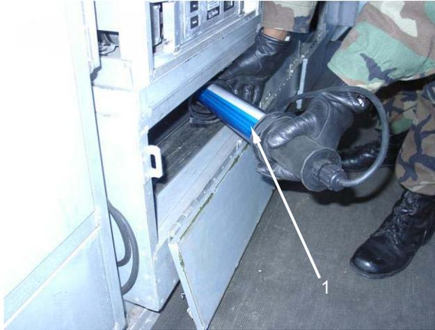
Loosen hose clamps and disconnect exhaust fan hose from heater weldment and from the hose adapter on the exhaust fan (1). Be sure to leave the heater weldment in place. Remove exhaust fan from roof and stow all components in storage area beneath burner racks (2).
