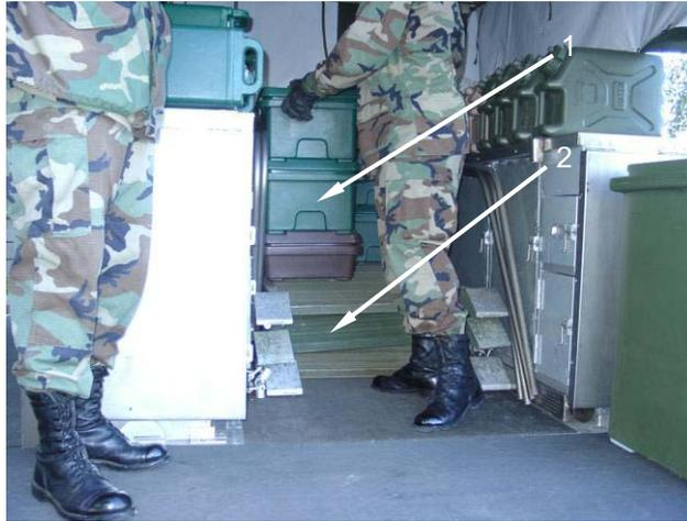
Move the ice chest (1) back into position at the end of the center aisle against the base of the ladders (2) and flush with the edge of the cabinets (3). Make sure that the handle (4) of the ice chest (1) is well behind the hole (5) used to stabilize the base of the roof jack so that the ice chest does not hinder the use of the roof jack in any way.
