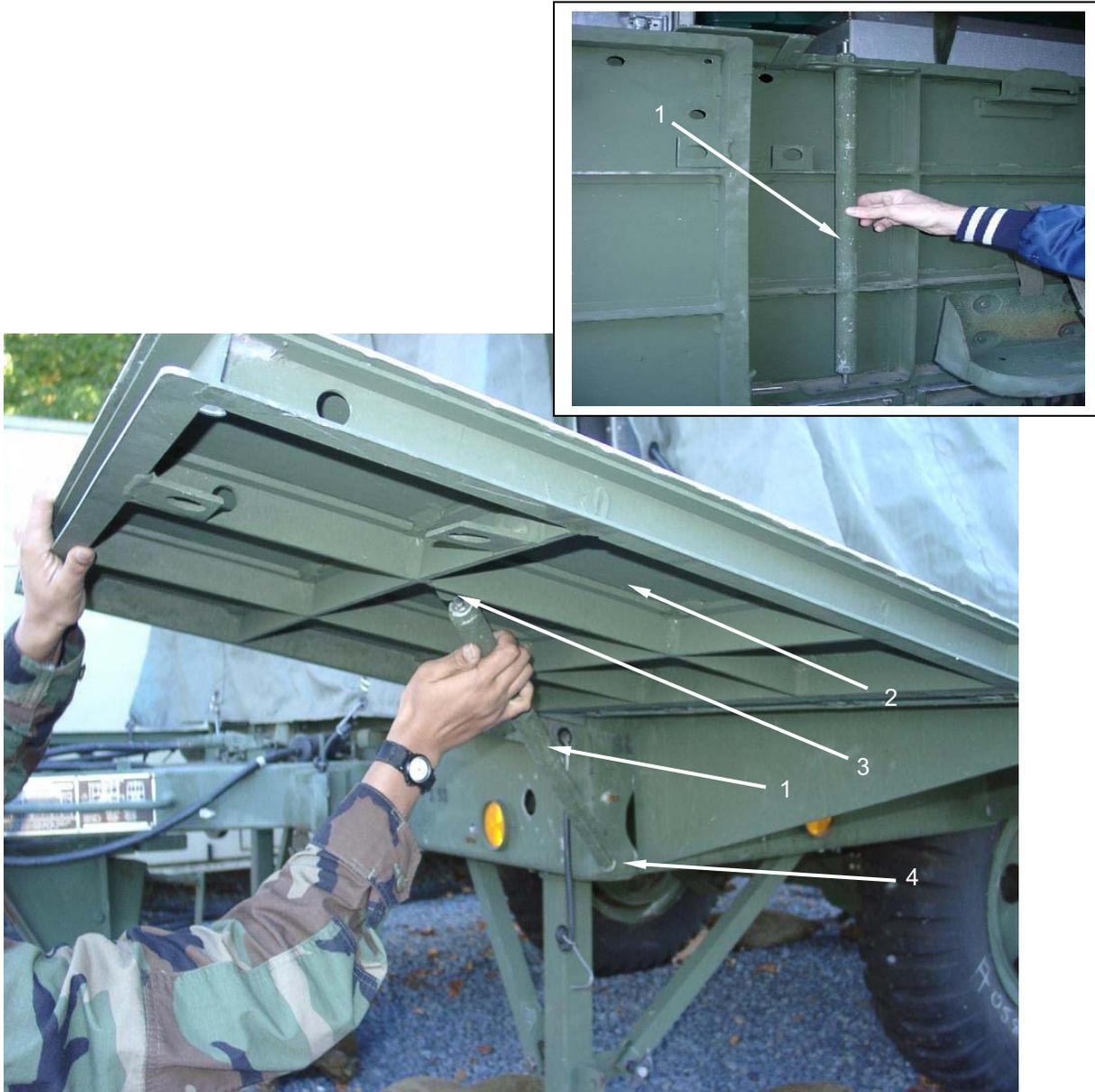
Release center aisle strap. Pull all four foldout braces (1) to right angles on end ramp (2). Check to ensure the four slide lock pins (3) are retracted. Lift eye bolt latch (or z-bar latch (4) – kitchen model MKT-85 serial no. 1494 and sub. MKT-90, MKT-95, and MKT-99) attached to corner post (5) at top of ramp.
