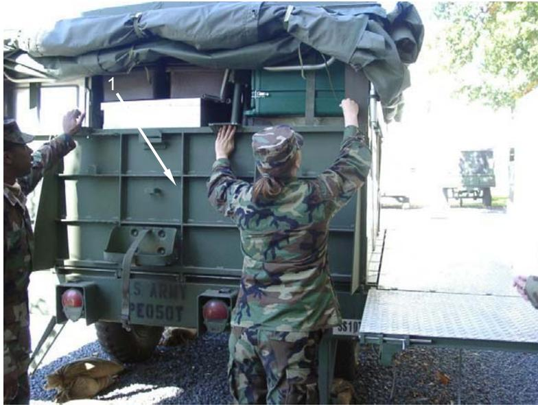
Secure front and rear end ramps (1) with eye bolt latches or z-bar (2). Fold in braces (3).
