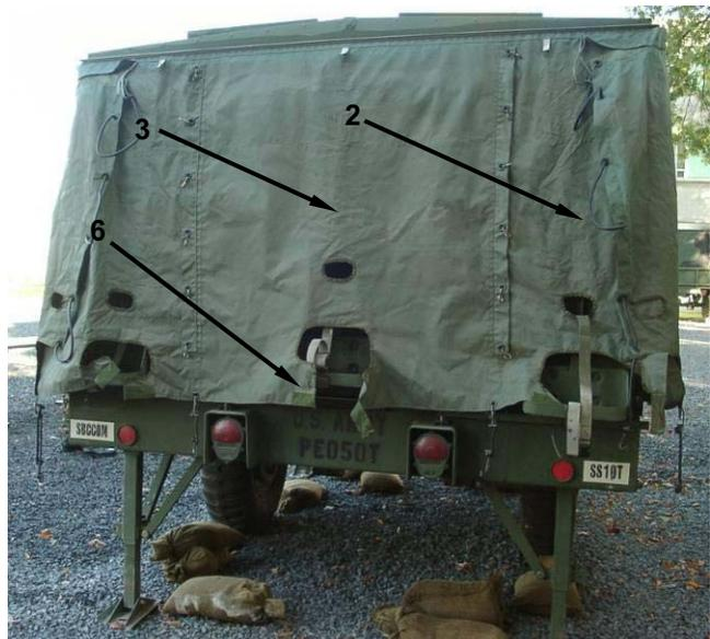
Move the travel covers aside and pull all braces (1) on side ramps (2) out at right angles to the ramp.
