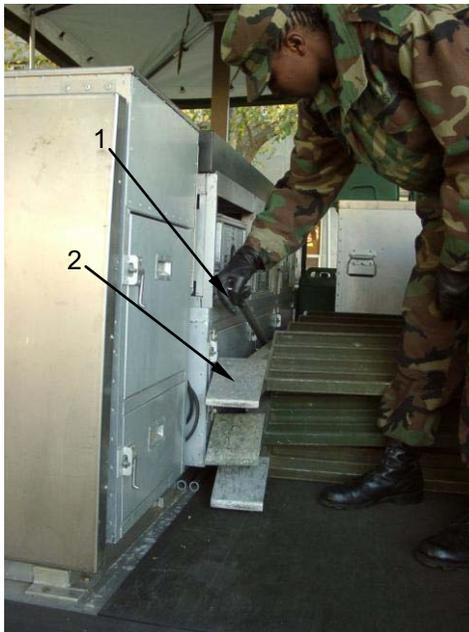
Remove roof canopy supports (1) and stow along the floor on the left and right side of the ladders (2).
