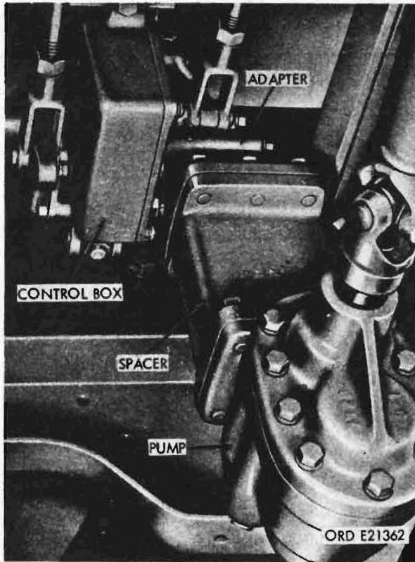
Figure 114. Hydraulic hoist pump and control box - viewed from below
