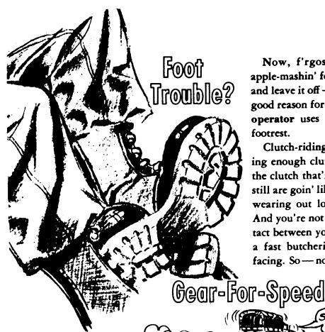
Now, f'rgoshsakes, get your big apple-mashin' foot off that clutch pedal and leave it off — until you've got some good reason for working the clutch. No operator uses the clutch pedal for a footrest.
