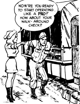
Leaks? Either lube or coolant? Check hoses, fittings, connections. Wet spots on ground?
