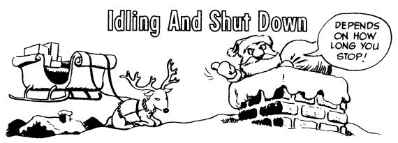
Keep your engine running—idle between 800 and 1000 RPM—for short stops. Figure a short stop is anything up to 30 minutes. You don't do your multifuel engine any favors by shutting down and starting up again all the time. It works better and lasts longer under steady operation.
