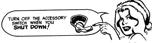
But remember that accessory switch when you shut down. Turn it off. Forgetting to turn off the accessory switch is one of the main causes of hydrostatic lock. Your in-tank fuel pump keeps running and pushing against fuel in the lines. This can push fuel past your manifold heater valves and on into your cylinders—a perfect setup for hydrostatic lock.
