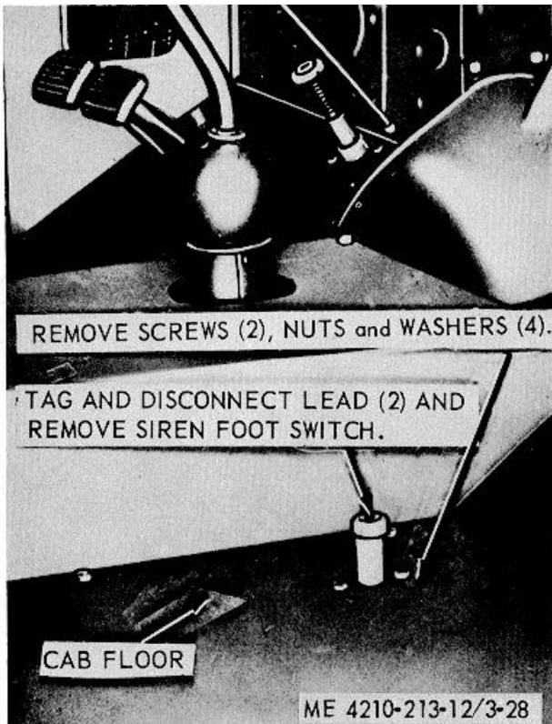
**Figure 3-28. Siren foot switch, removal and installation.**
