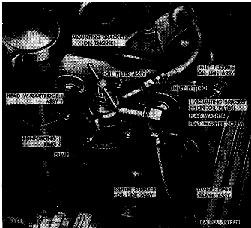
Figure 30. Oil filter assembly—installed.
