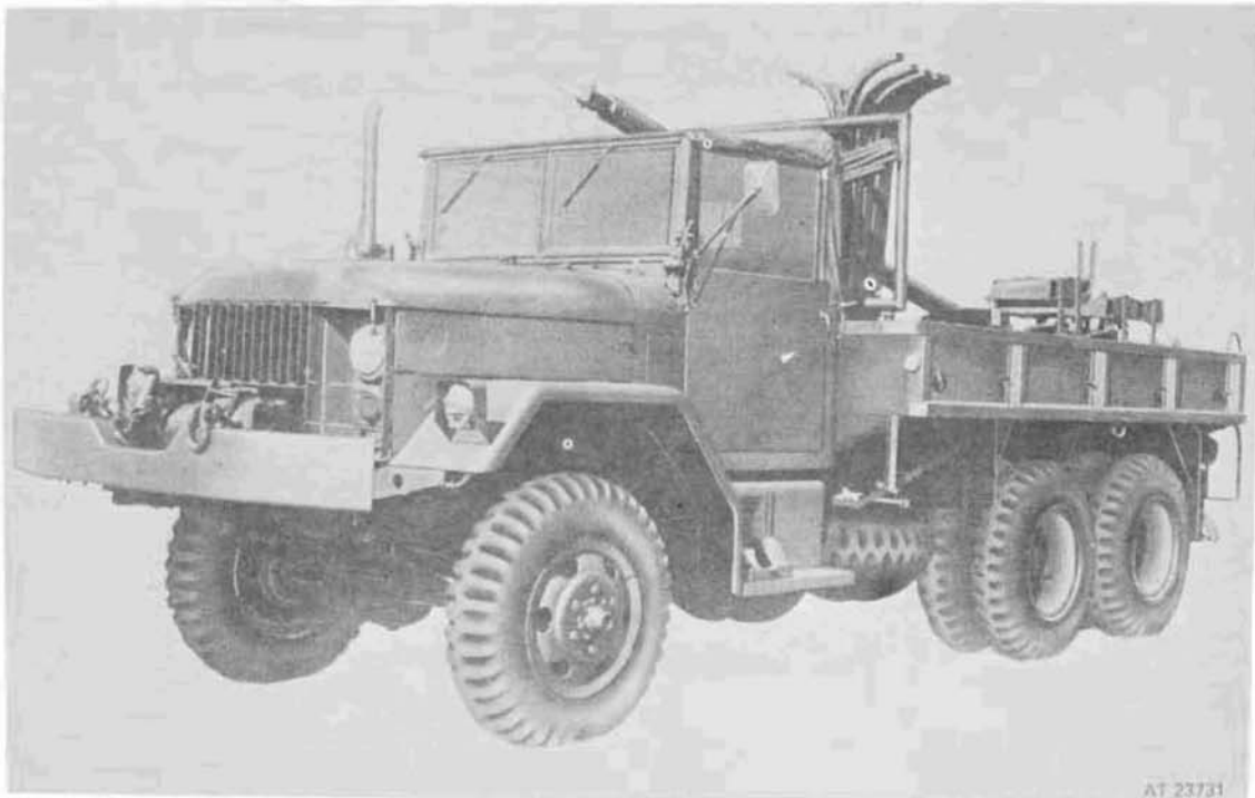
Figure 454. 2-1/2 ton, 6x6, M764 earth boring machine and pole- setter truck - left front view.
