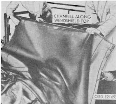
Figure 255. Installing cab top paulin
