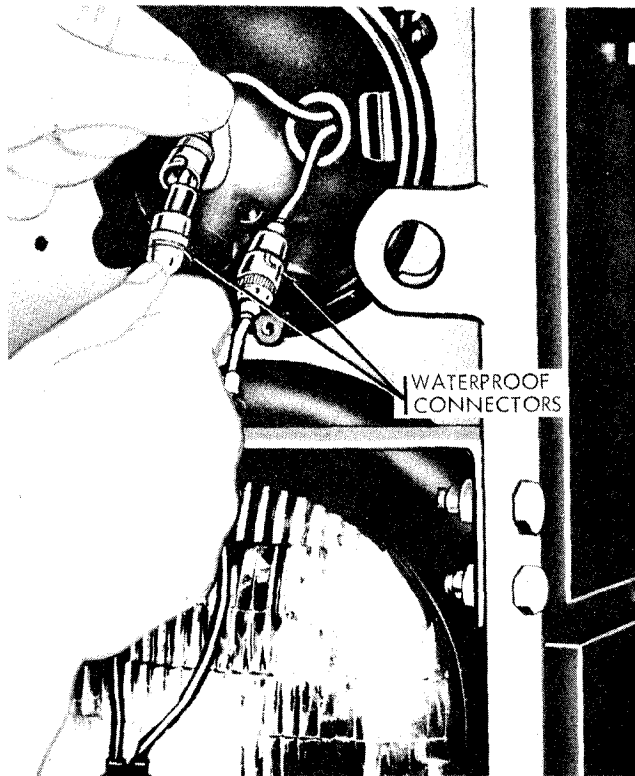
Figure 2-160. Removing blackout driving light sealed-beam lamp unit.
