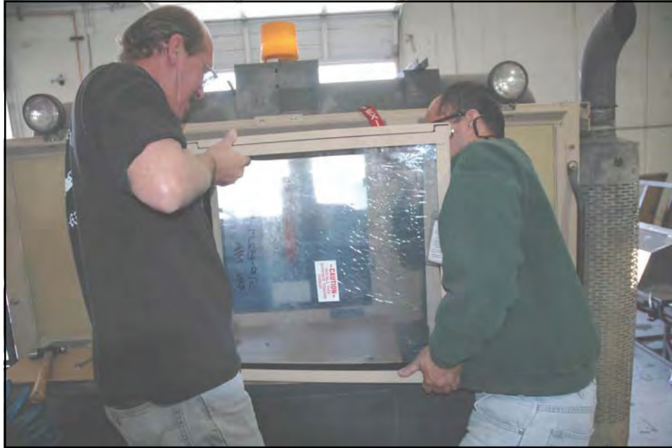
16. Lift the Window Assembly in place aligning the slots in the hinge with the holes in the Mounting Frame. *NOTE: THIS IS A TWO MAN LIFT
