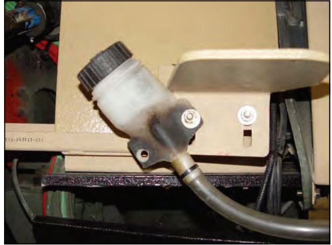
10.) Reinstall washer fluid box while installing hood support brackets
