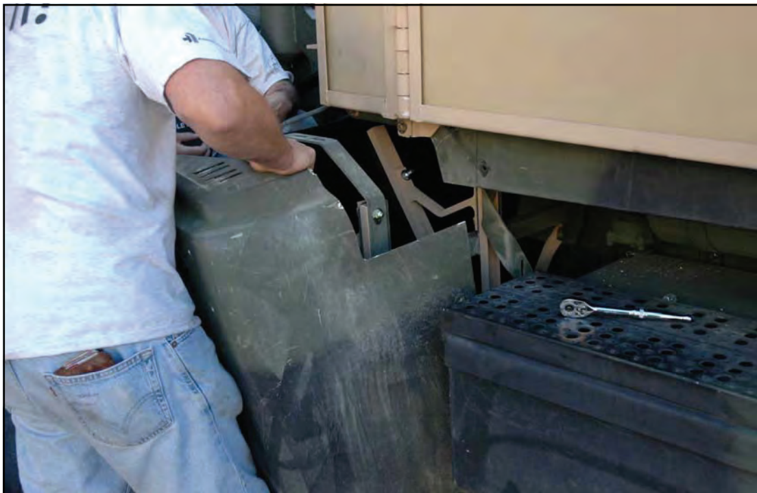
11.) Re-install original wheel well deflectors and ensure the wire from the side light has been connected. Note: fenders may need to be trimmed to make armor fit and will need to be trimmed to accommodate armor
