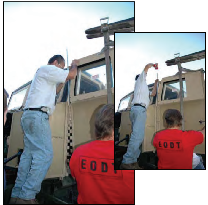
4.) Still using the forklift position hingbrackets on the door with brackets on the truck (at least three men are needed for this step)
