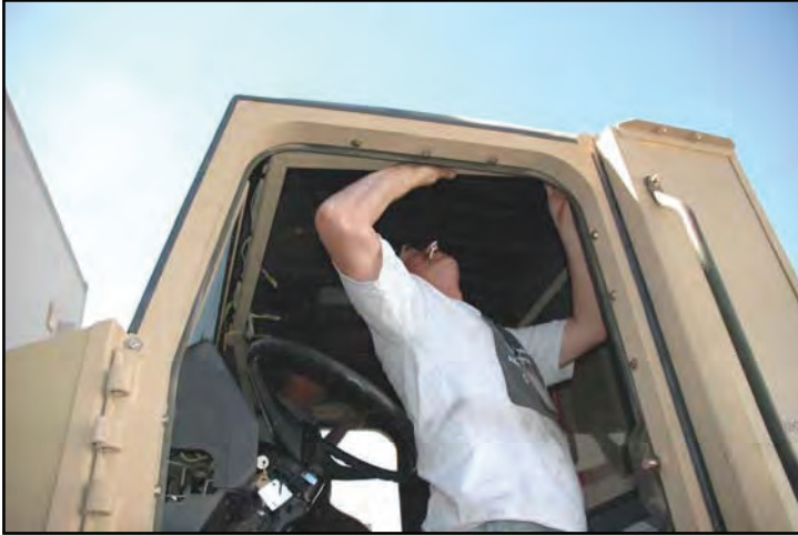
1.) Align roof frame with brackets installed earlier.
