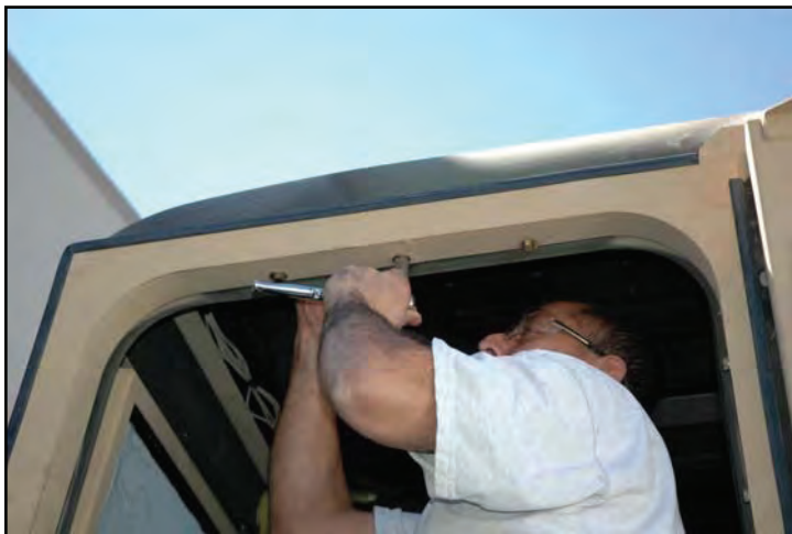
3.) Tighten bolts on frame of door.
