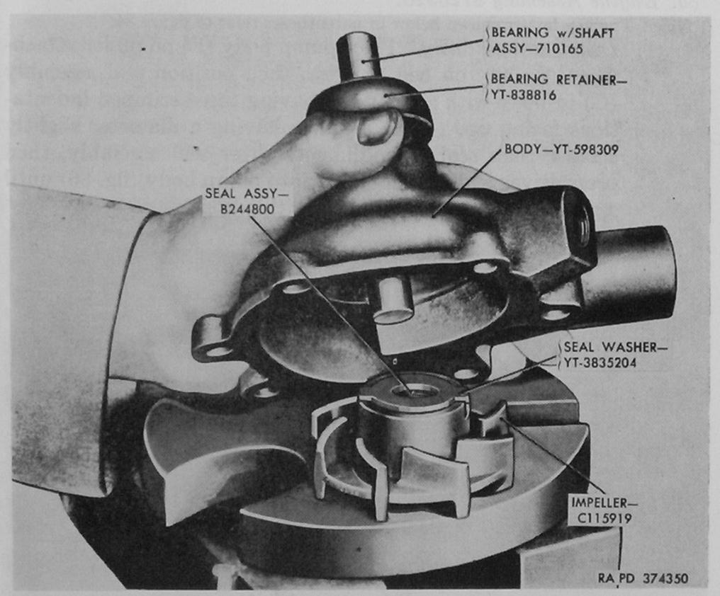
Figure 85. Positioning water pump body and bearing with shaft over impeller—engine assemblies 7411599 and 8329440.
