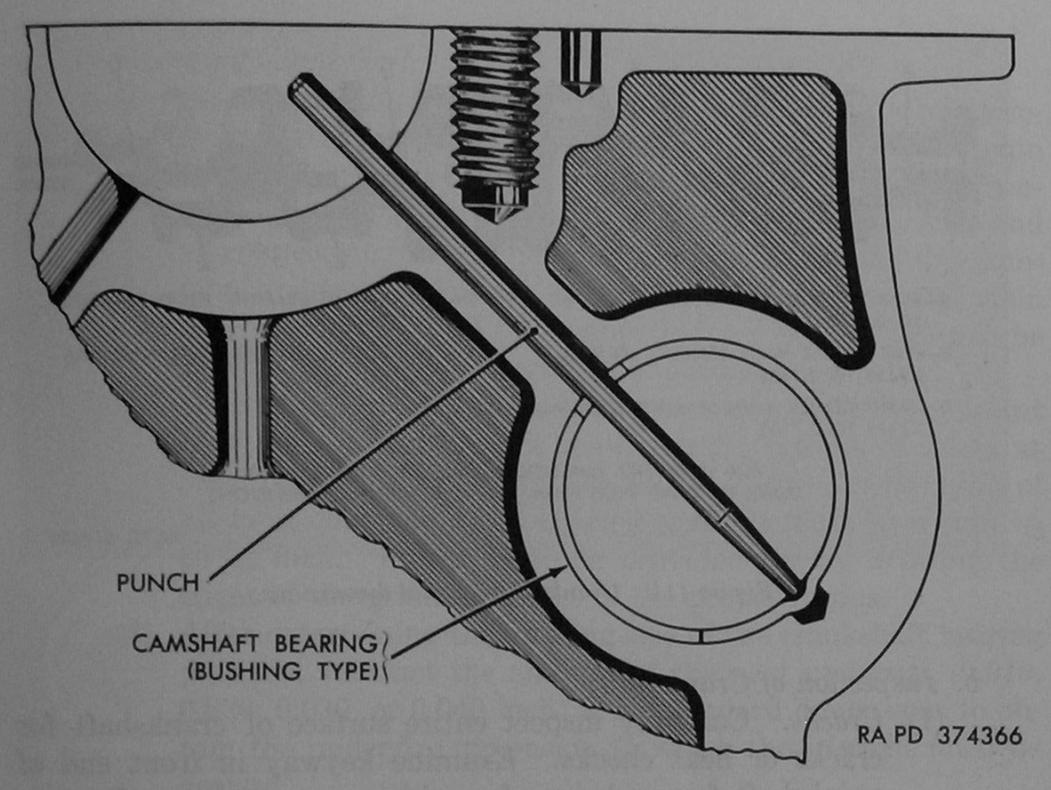
Figure 113. Locking camshaft bearings.
