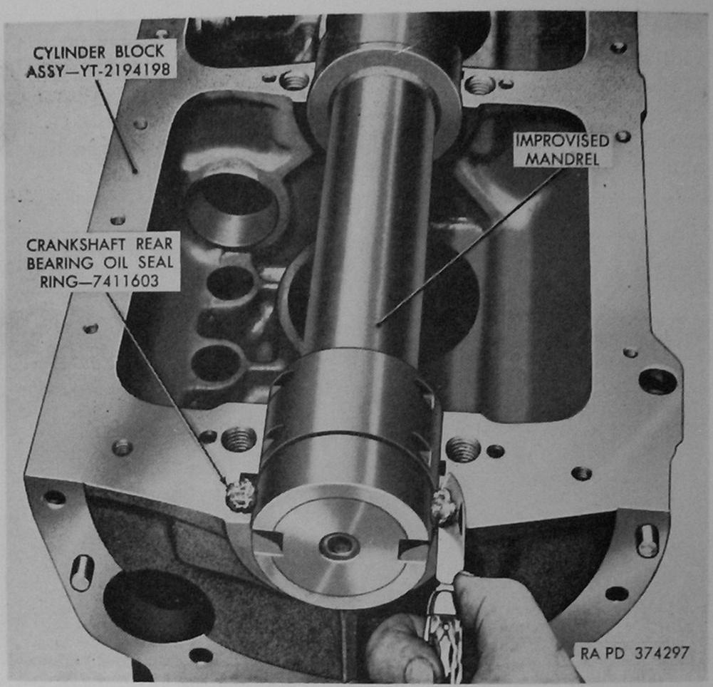
Figure 125. Installing crankshaft rear bearing oil seal ring using improvised mandrel.
