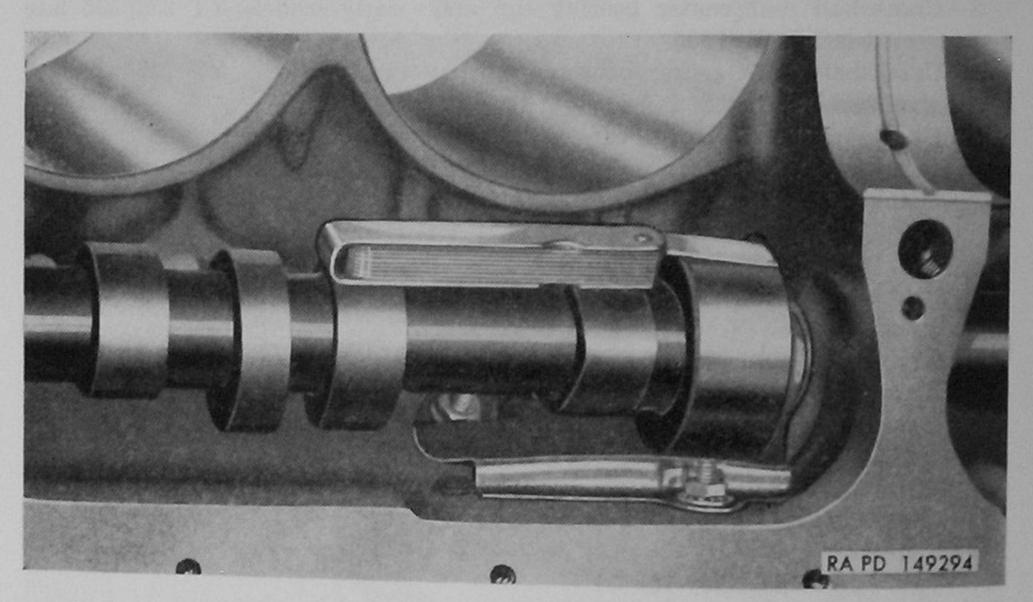
Figure 112. Checking camshaft bearing clearance with feeler (thickness) gage.
