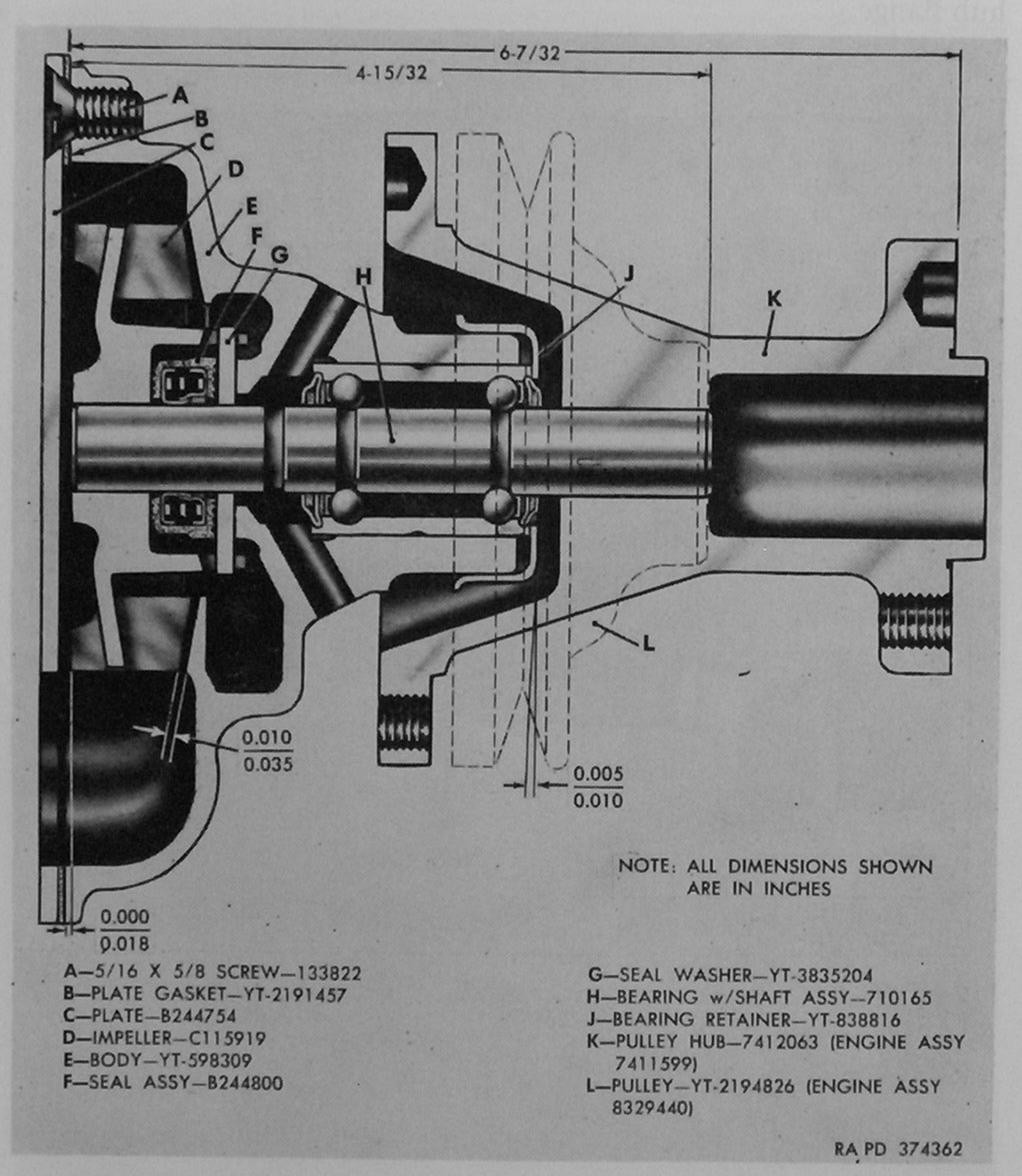
Figure 79. Water pump assembly—engine assemblies 7411599 and 8329440.
