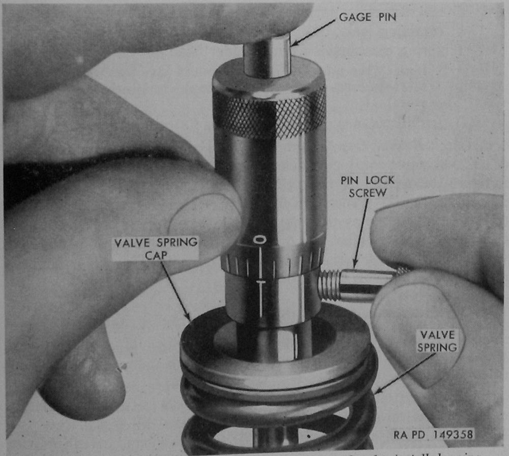
Figure 163. Checking valve rotator cap clearance with valve installed, using gage 7083104.
