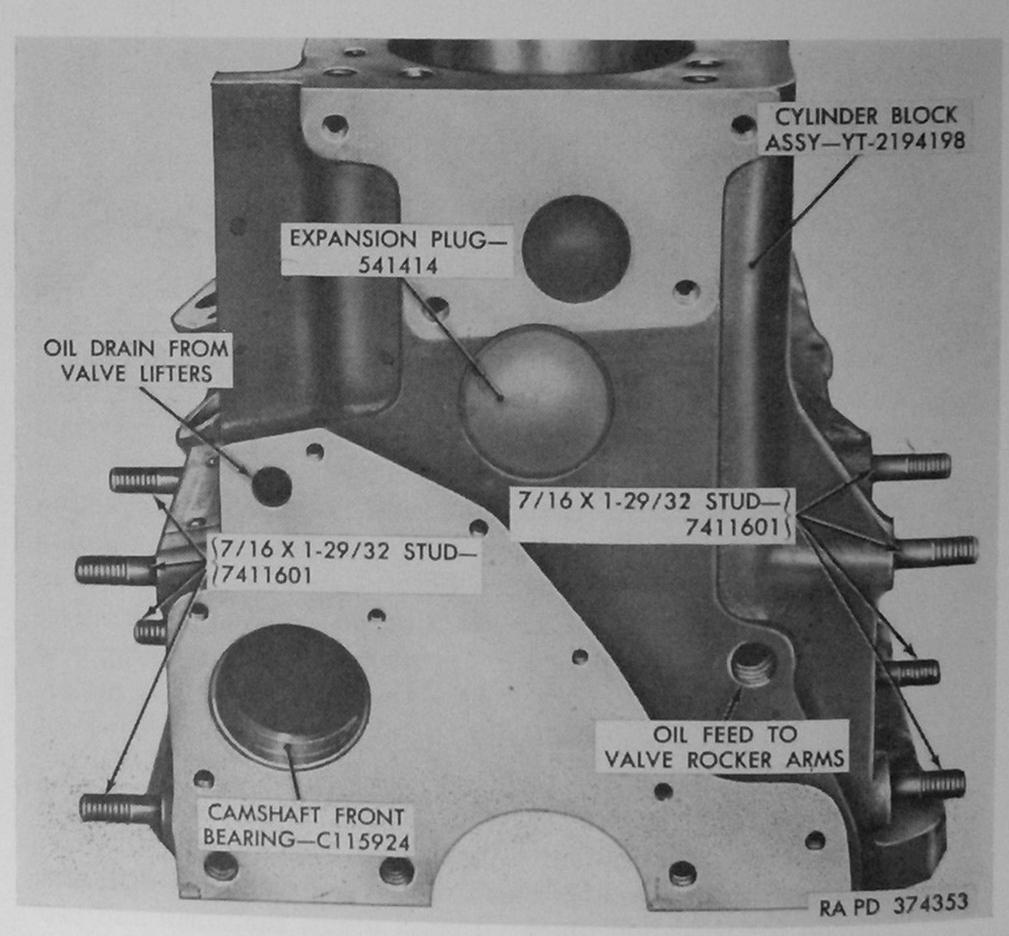
Figure 122. Front view of cylinder block assembly.
