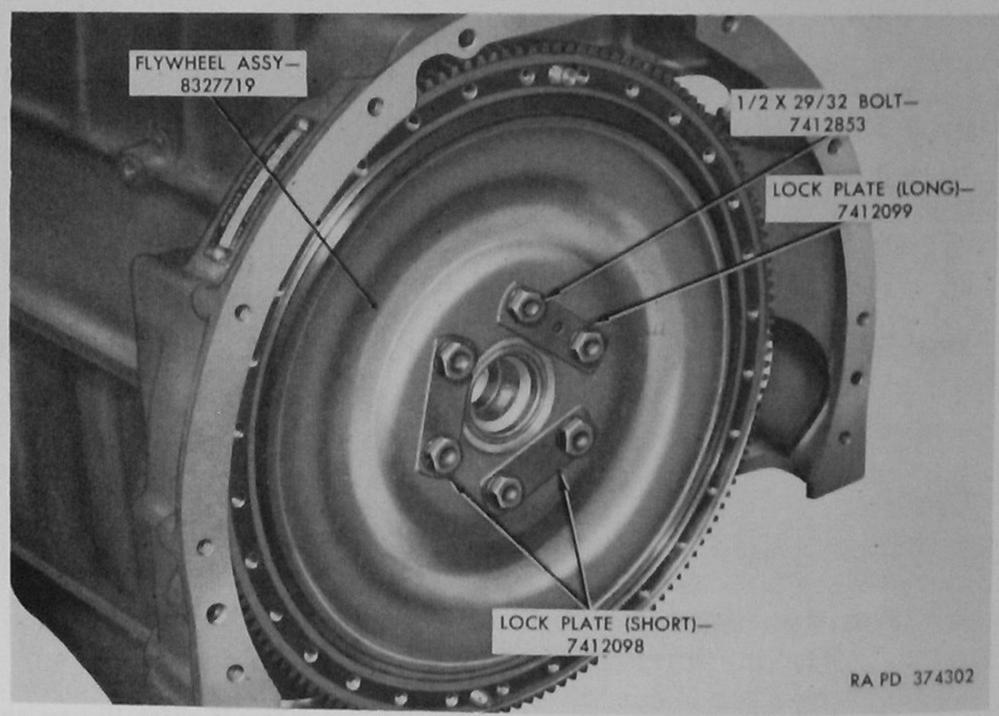
Figure 146. Flywheel installed—engine assemblies 7411599 and 8329440 shown.
