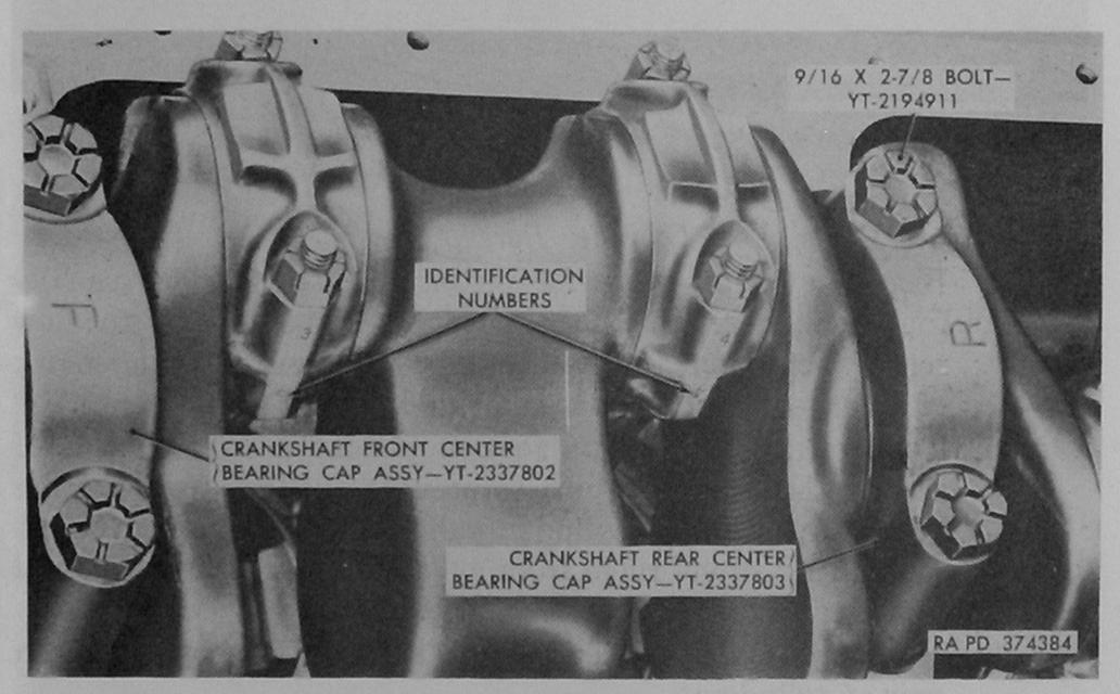
Figure 59. Identification markings on connecting rods and crankshaft bearing caps (late model engine shown).
