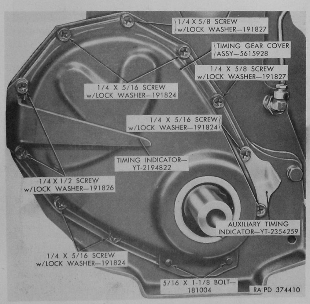
Figure 135. Timing gear cover and timing indicators installed—engine assembly 8329440.
