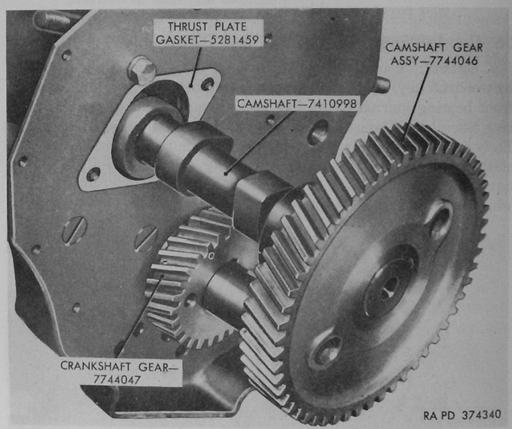
Figure 66. Camshaft and gear assembly partially removed (early engine assembly 7411599 shown).
