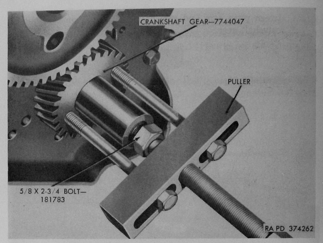
Figure 68. Removing crankshaft gear using puller 7950886.
