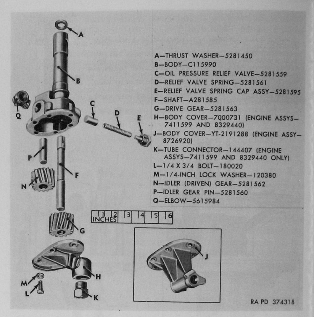
Figure 89. Oil pump components.
