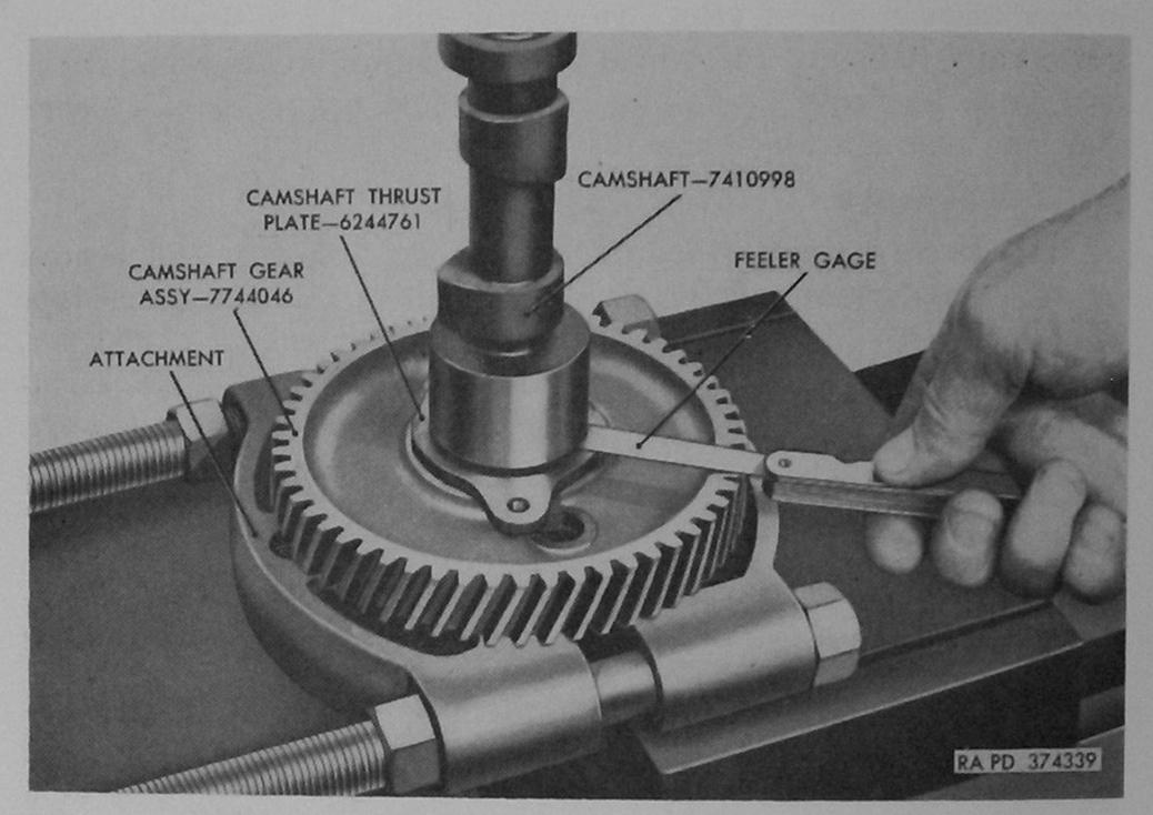
Figure 131. Installing camshaft gear assembly on camshaft—early engine assemblies 7411599 and 8329440.
