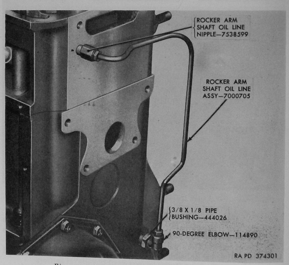
Figure 52. Rocker arm shaft oil line assembly installed.
