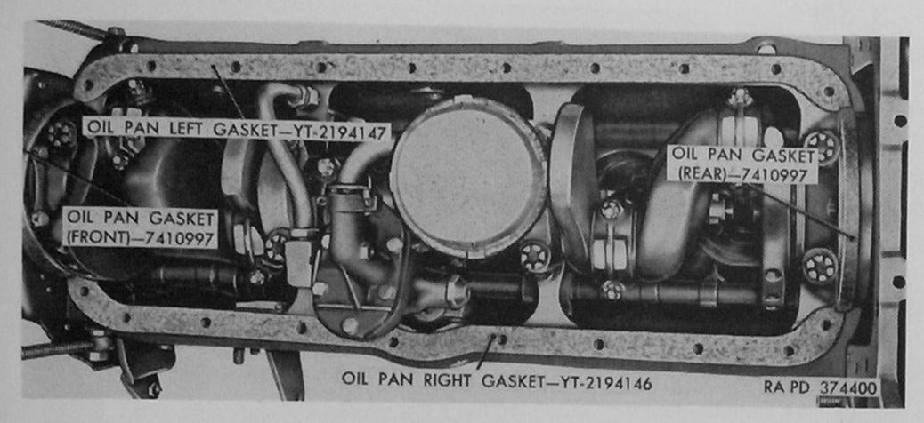
Figure 154. Engine oil pan gaskets installed—engine assembly 8726920 shown.
