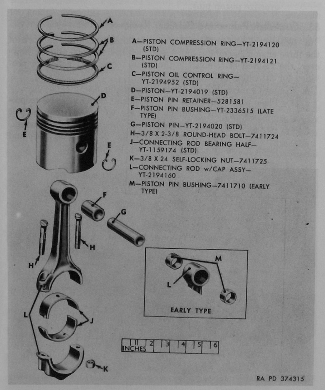
Figure 61. Connecting rod and piston components.
