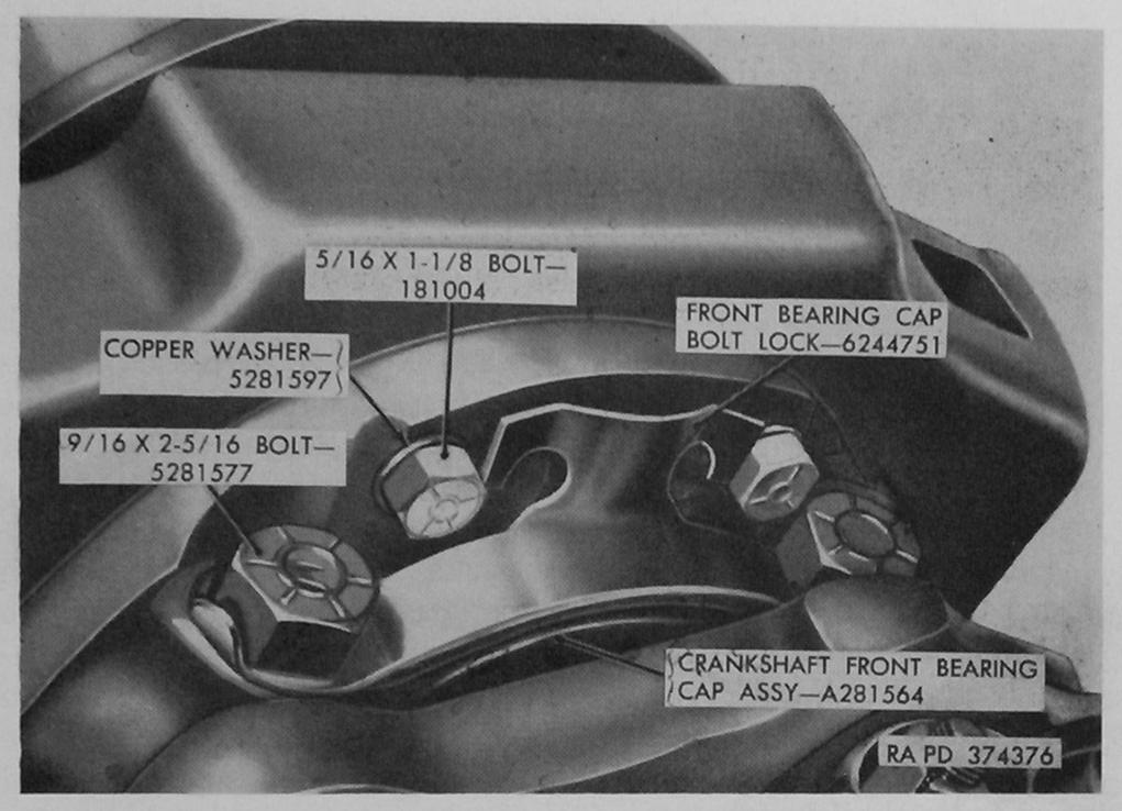
Figure 137. Crankshaft front bearing cap bolt lock—early engine assemblies 7411599 and 8329440.
