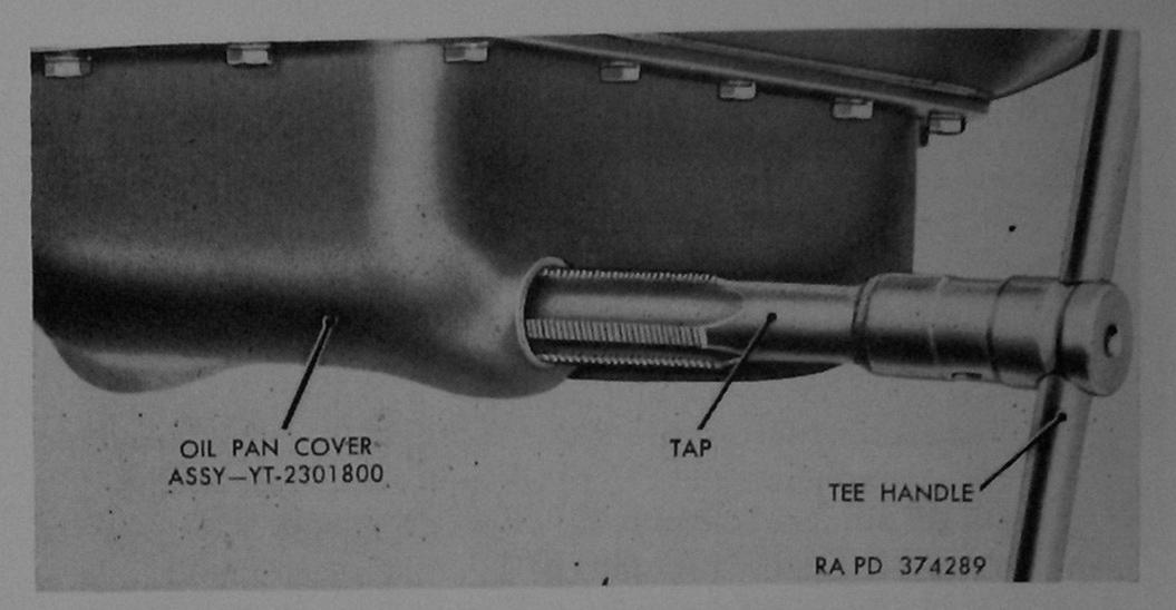
Figure 157. Using special tap 8720299 to clean up threads in oil pan drain plug hole
