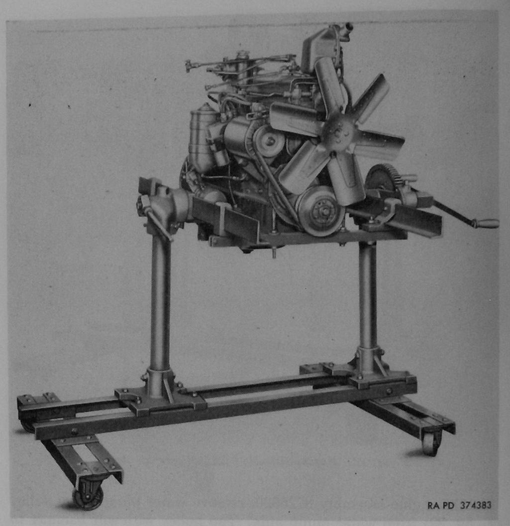
Figure 13. Engine assembly 8726920 in repair stand.
