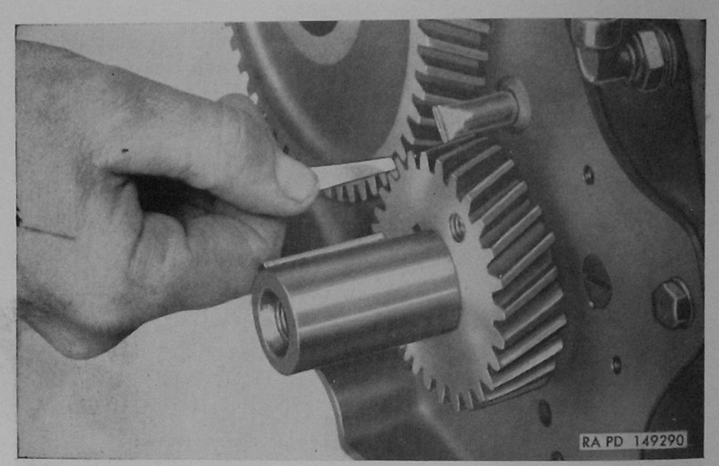
Figure 133. Checking timing gear backlash.
