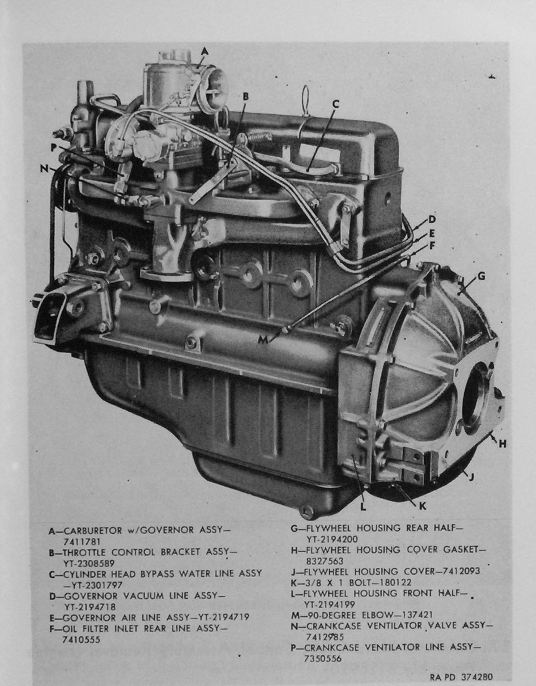
Figure 20. Engine assembly 8329440—left rear view.
