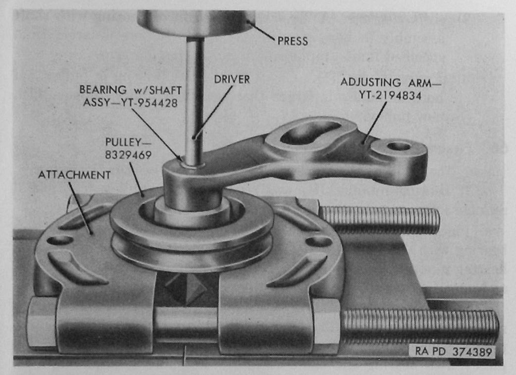
Figure 72. Pressing idler bearing with shat assembly from adjusting arm and pulley —engine assembly 8329440.
