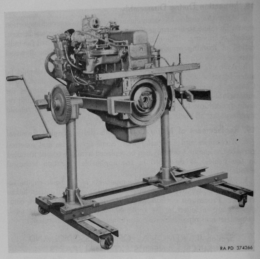
Figure 11. Engine assembly 7411599 in repair stand.
