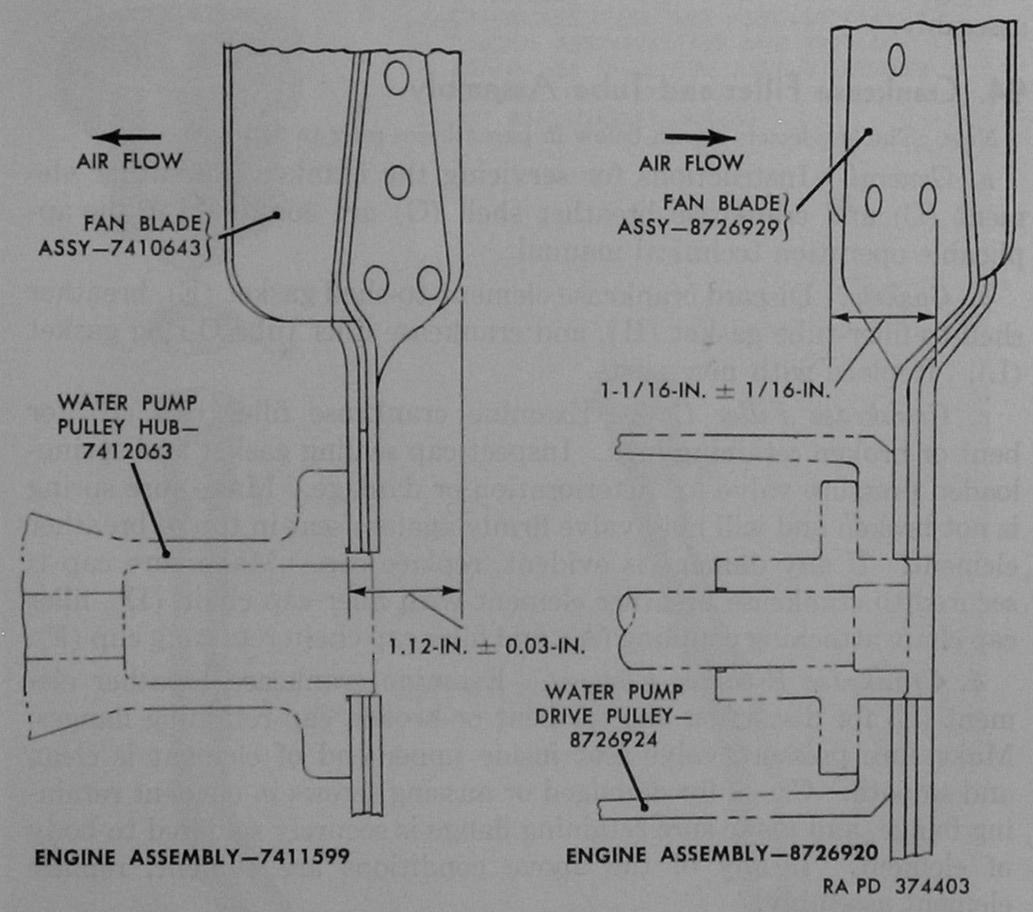
Figure 94. Fan blade alinement dimensions—engine assemblies 7411599 and 8726920.
