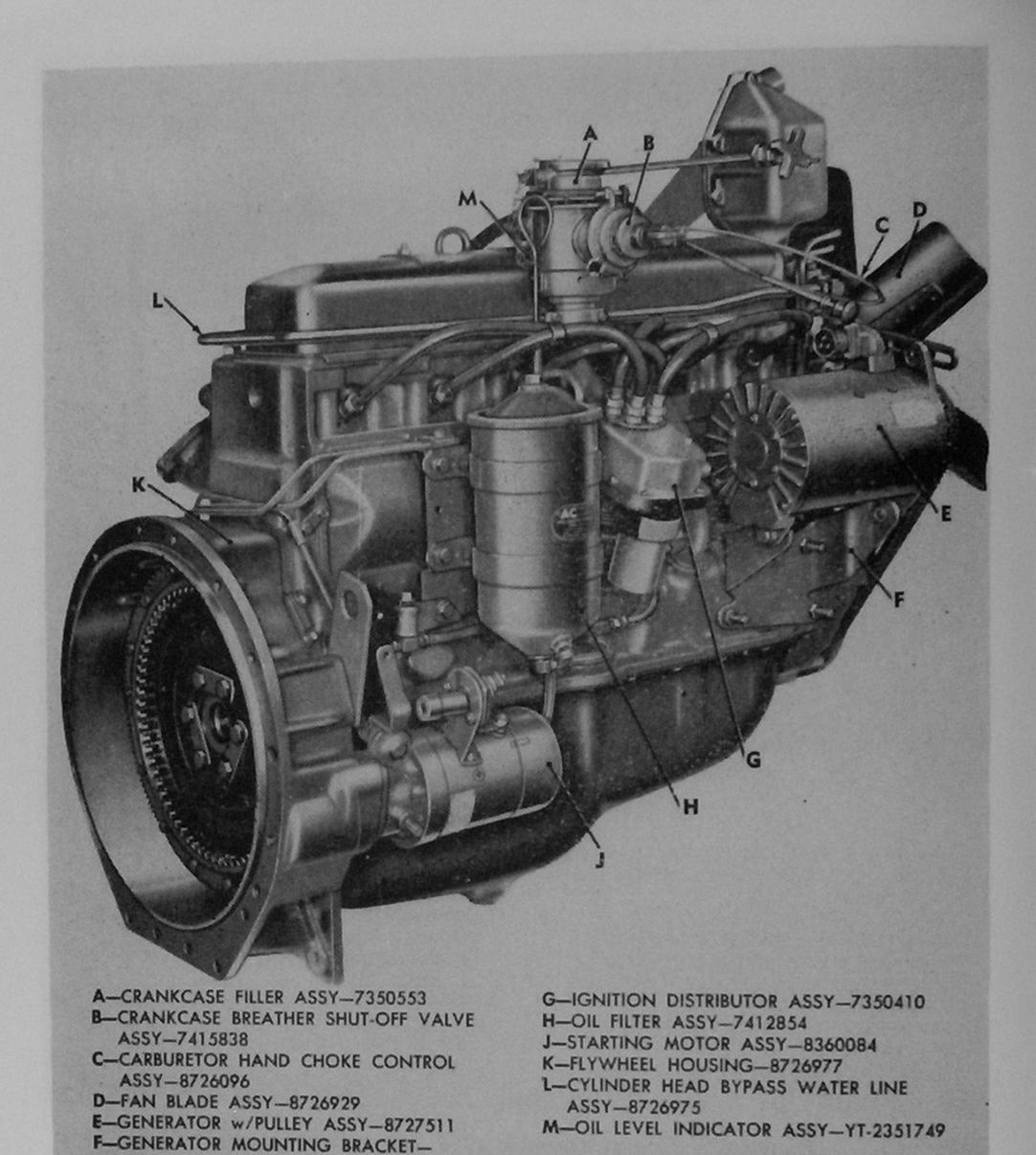
Figure 23. Engine assembly 8726920—right rear view.
