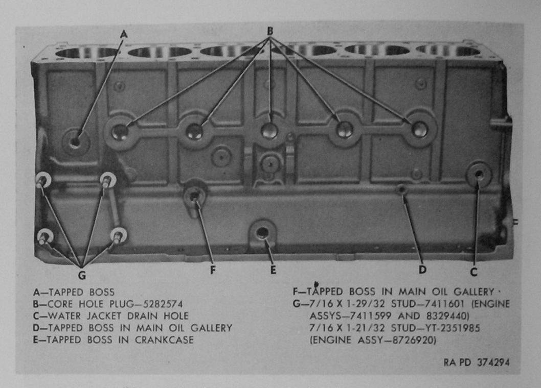
Figure 121. Left view of cylinder block assembly.
