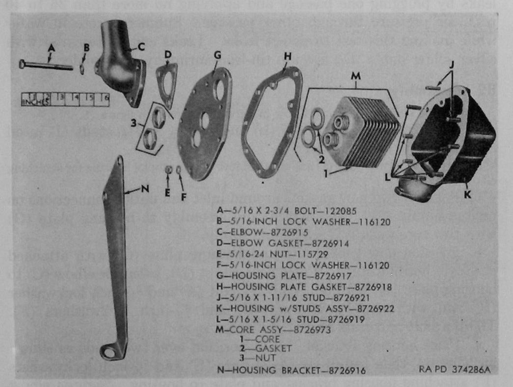
Figure 78. Engine oil cooler components—engine assembly 8726920.
