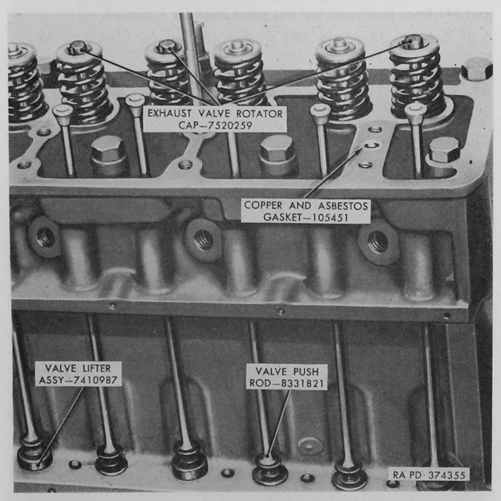
Figure 51. Push rods and lifters installed.
