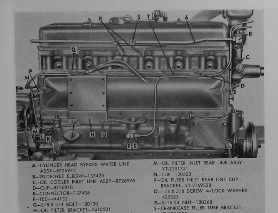
Figure 34. Right side of engine assembly 8726920 with oil filter, distributor, and generator removed.
