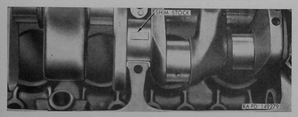
Figure 128. Use of shim stock to check bearing clearance.
