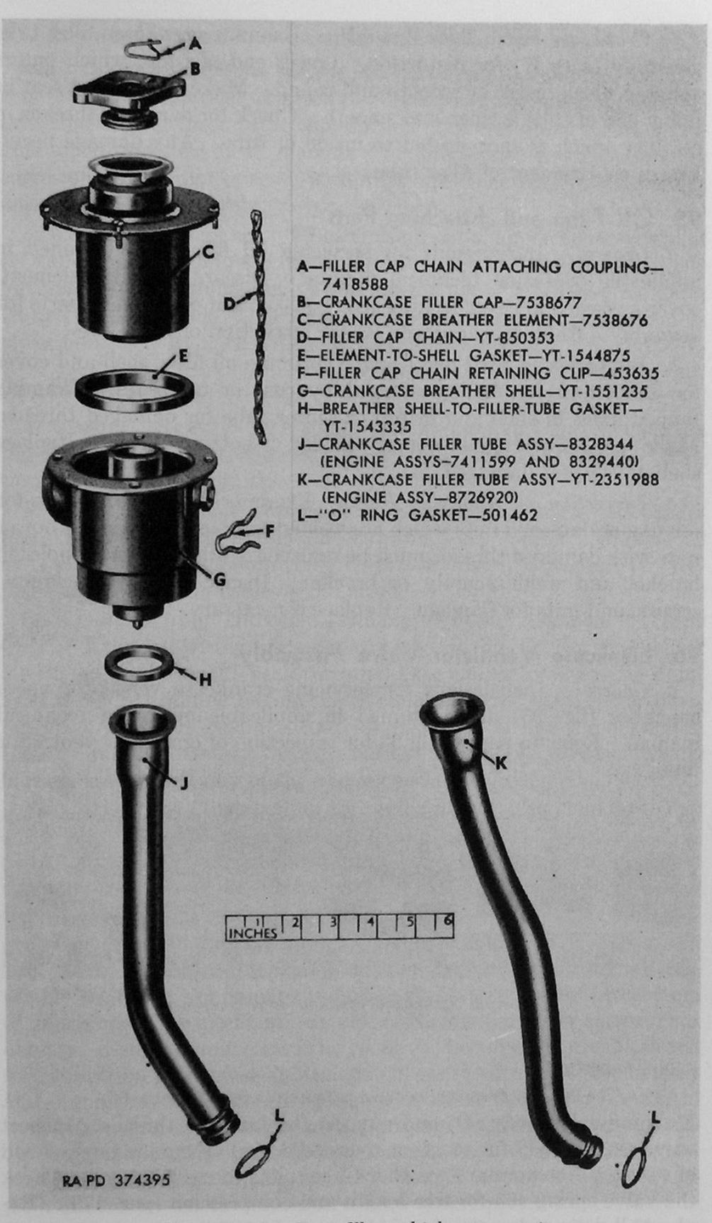
Figure 95. Crankcase filler and tube components.
