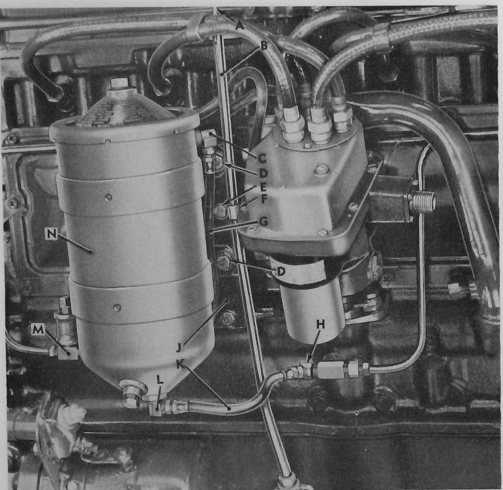
A-OIL LEVEL INDICATOR ASSY-YT-2301798 (ENGINE ASSY-8329440) YT-2351749 (ENGINE ASSY-8726920)
