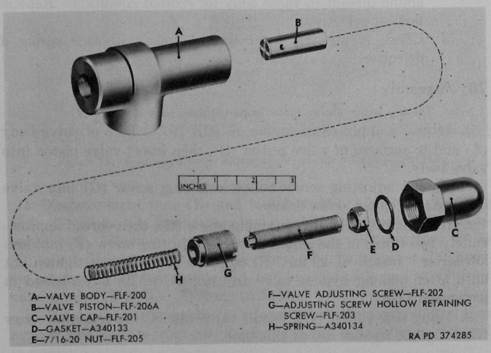
Figure 77. Engine oil bypass valve components—engine assembly 8726920.
