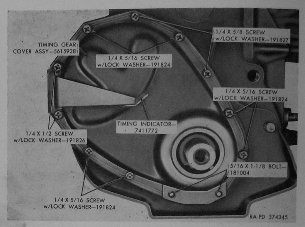
Figure 136. Timing gear cover and timing indicator installed—engine assemblies 7411599 and 8726920.
