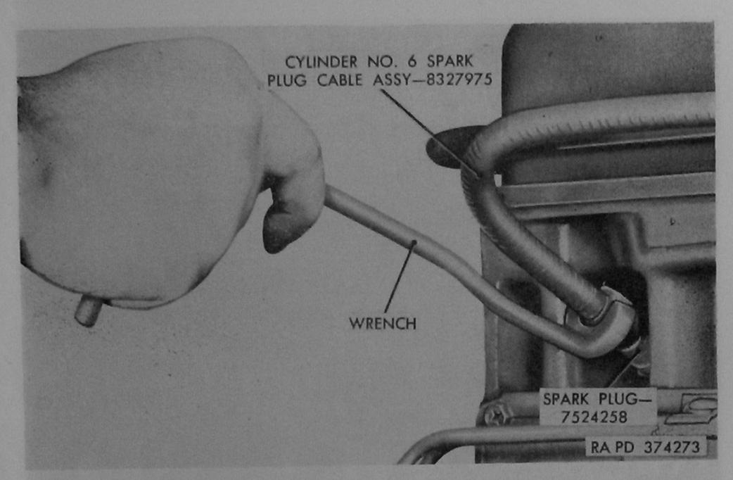
Figure 32. Disconnecting spark plug cable using wrench 7950895.
