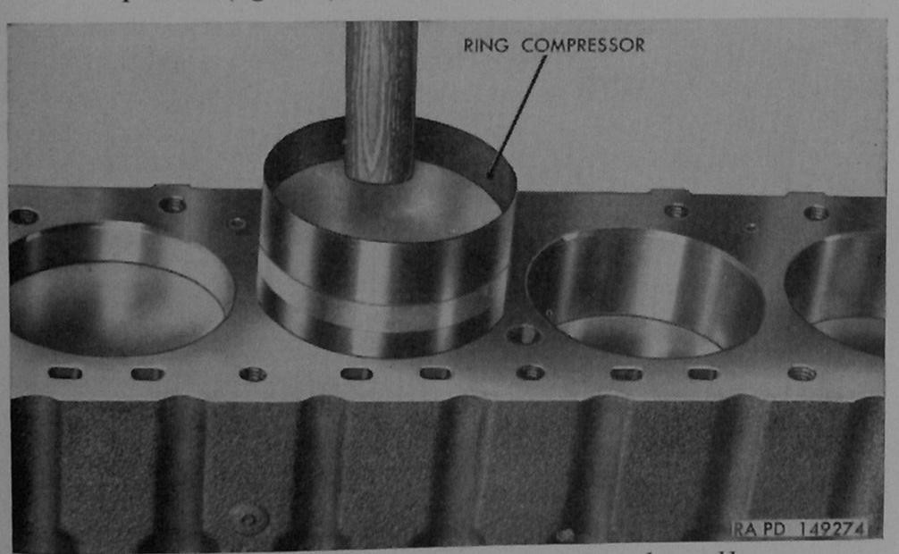
Figure 153. Installing piston and connecting rod assembly.
