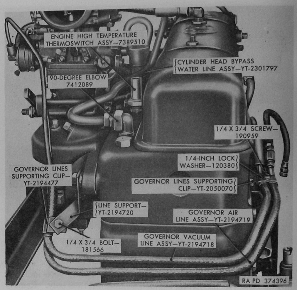
Figure 37. Location of governor line clips and cylinder head bypass water line—engine assembly 8329440.
