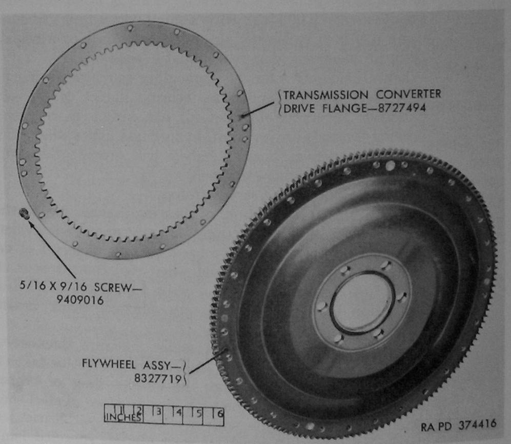
Figure 115. Engine flywheel and drive flange—engine assembly 8726920.
