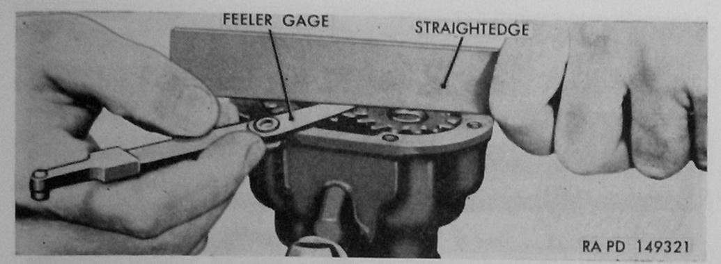
Figure 91. Checking oil pump gear to cover clearance.
