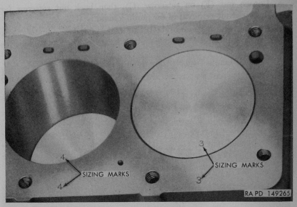
Figure 60. Sizing marks on pistons and cylinder bores.
