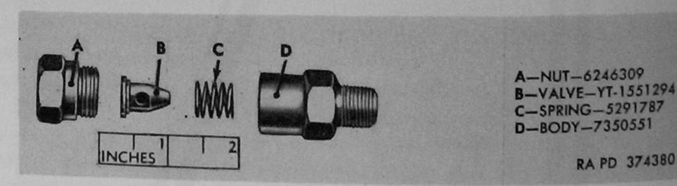
Figure 96. Crankcase ventilator valve components.
