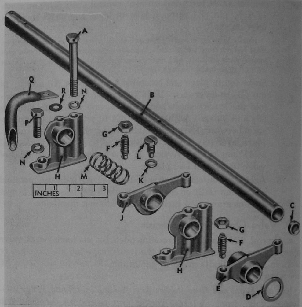
A-3/8 X 3-1/4 BOLT-189304 B-VALVE ROCKER ARM SHAFT-YT-2193774
