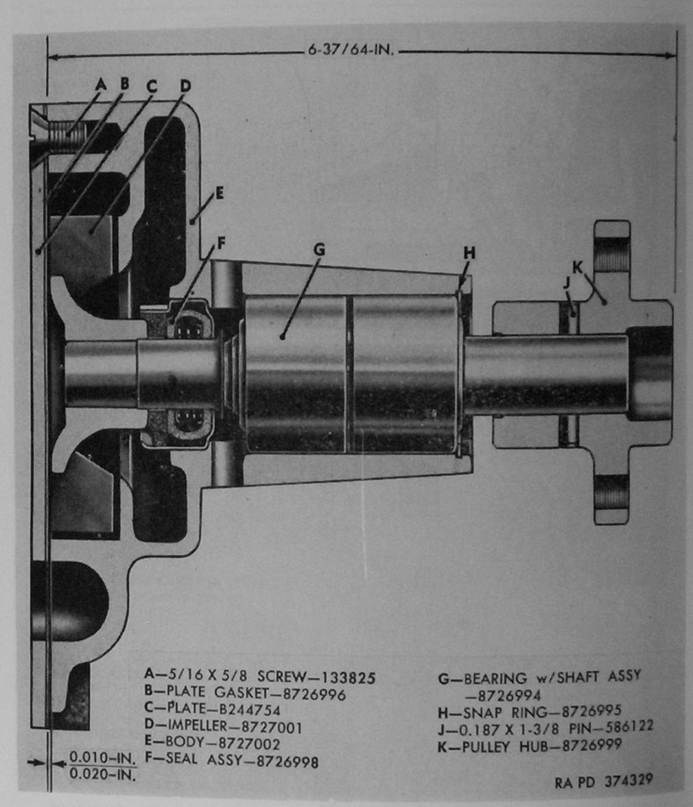
Figure 80. Water pump assembly—engine assembly 8726920.
