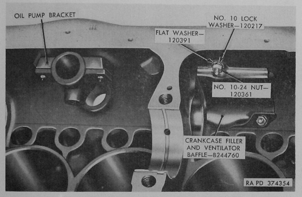
Figure 124. Crankcase filler and ventilator baffle installed on cylinder block.
