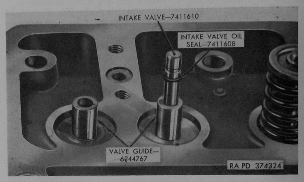
Figure 54. Oil seal in groove in intake valve stem.
