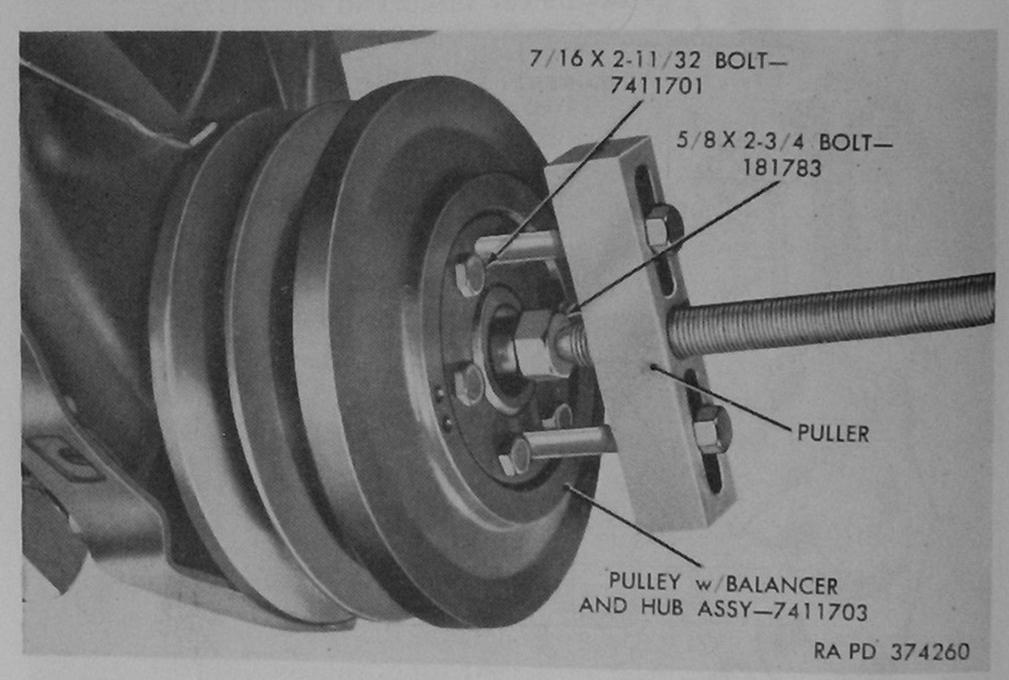
Figure 62. Removing crankshaft pulley and balancer assembly from crankshaft using puller 7950886 (engine assembly 7411599 shown).
