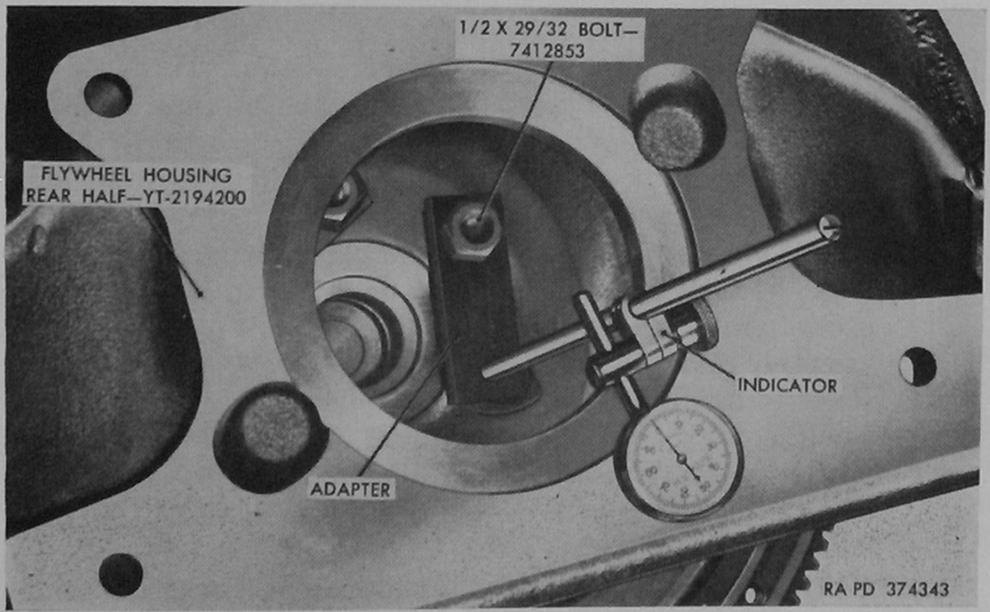
Figure 142. Checking squareness of rear face of flywheel housing rear half—engine assemblies 7411599 and 8329440.
