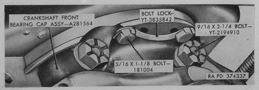
Figure 138. Timing gear cover bolts and bolt lock—late engine assemblies 7411599 and 8329440, and all engine assemblies 8726920.
