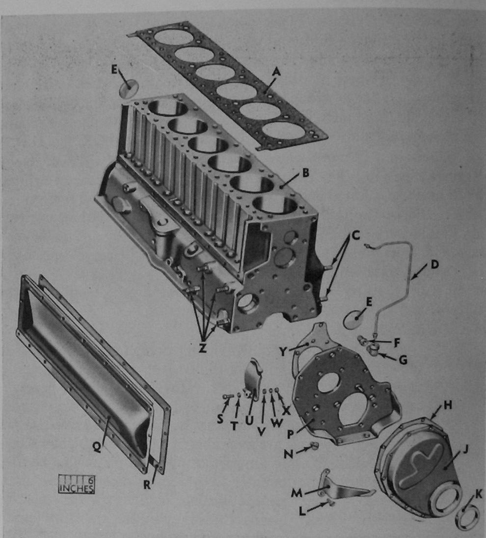
A-CYLINDER HEAD GASKET-7411605 B-CYLINDER BLOCK ASSY-YT-2194198 C-7/16 X 1-21/32 STUD-YT-2351985 D-ROCKER ARM SHAFT OIL LINE
