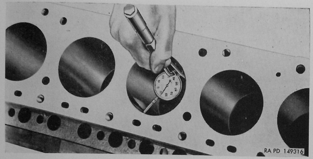
Figure 119. Checking cylinder bores with indicator.
