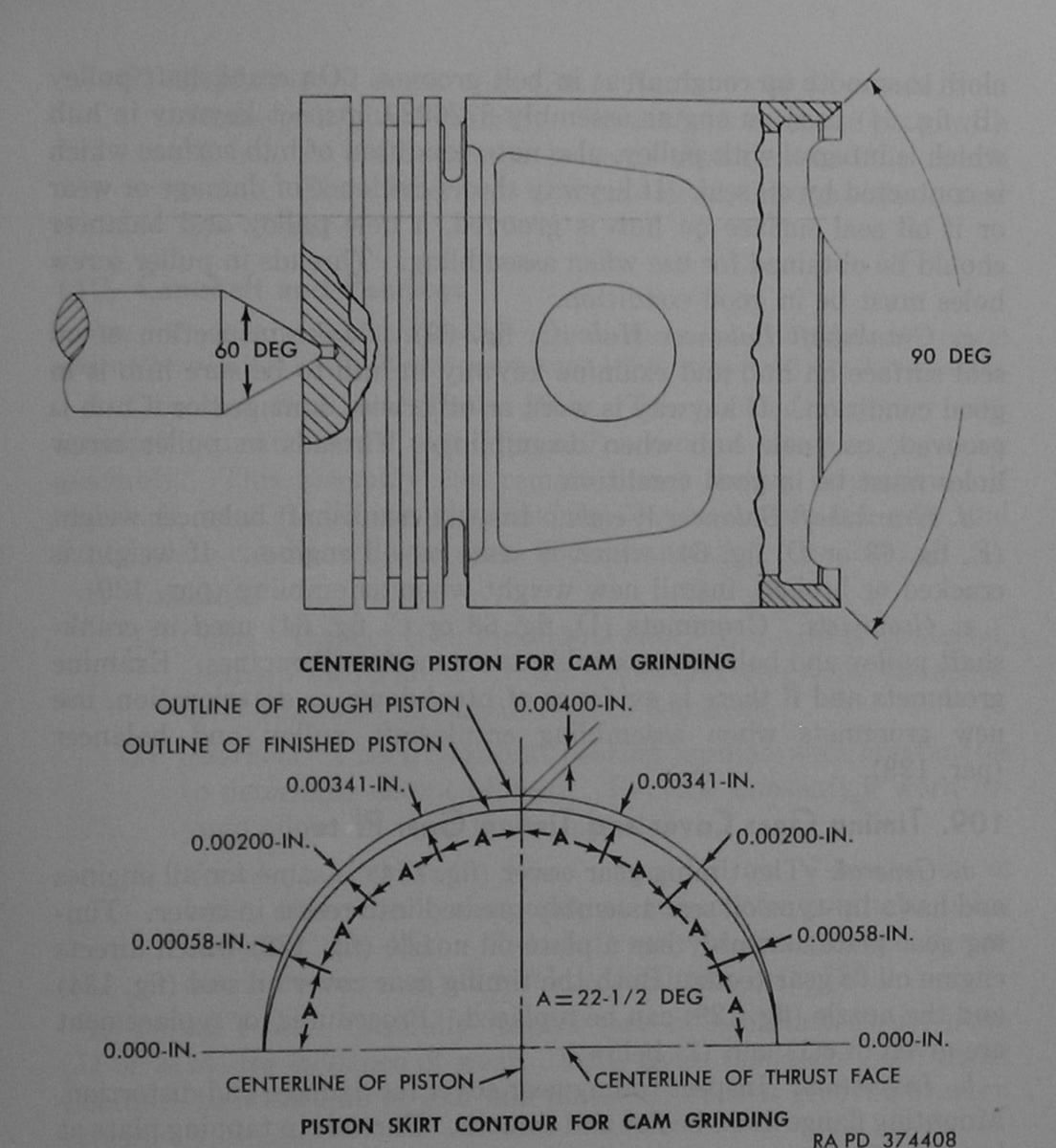
Figure 108. Piston centering and grinding of semifinished pistons.
