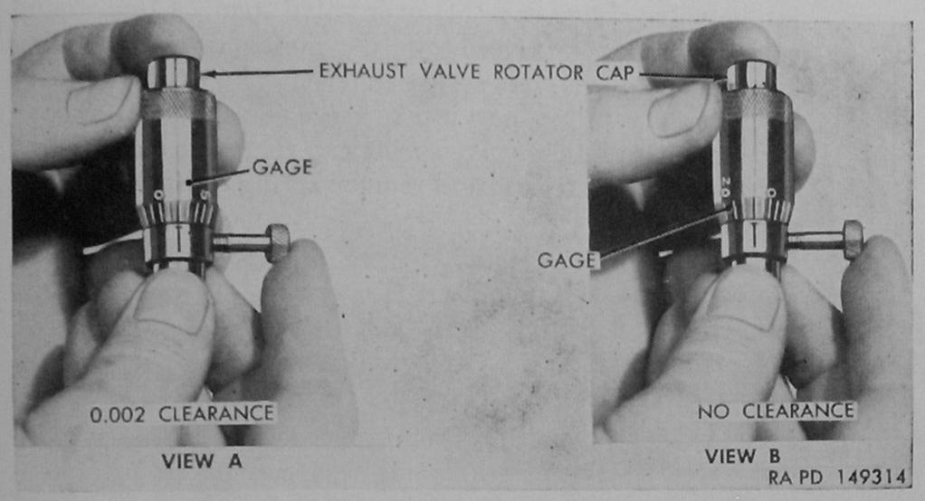
Figure 162. Using gage 7083104 to check valve rotator cap clearance.
