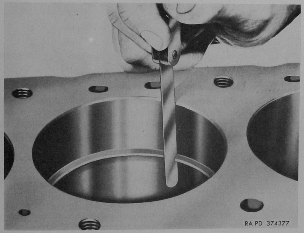
Figure 149. Checking piston ring gap.
