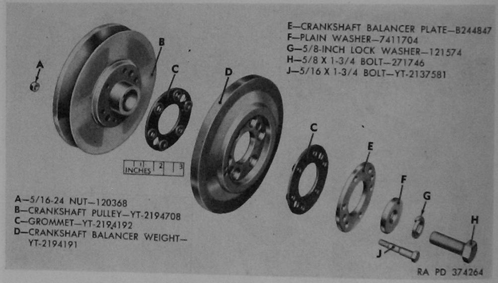
Figure 64. Crankshaft pulley and balancer components—engine assembly 8726920.
