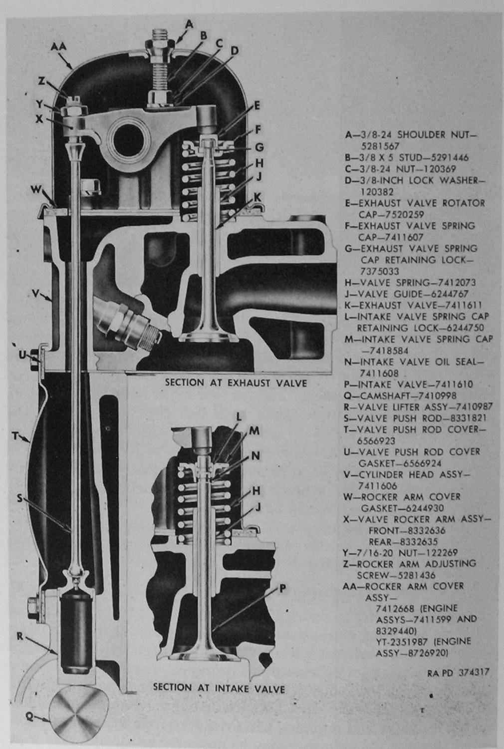
Figure 159. Sectional view of cylinder head and valve mechanism.
