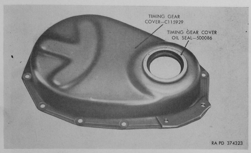
Figure 134. Timing gear cover with oil seal installed.
