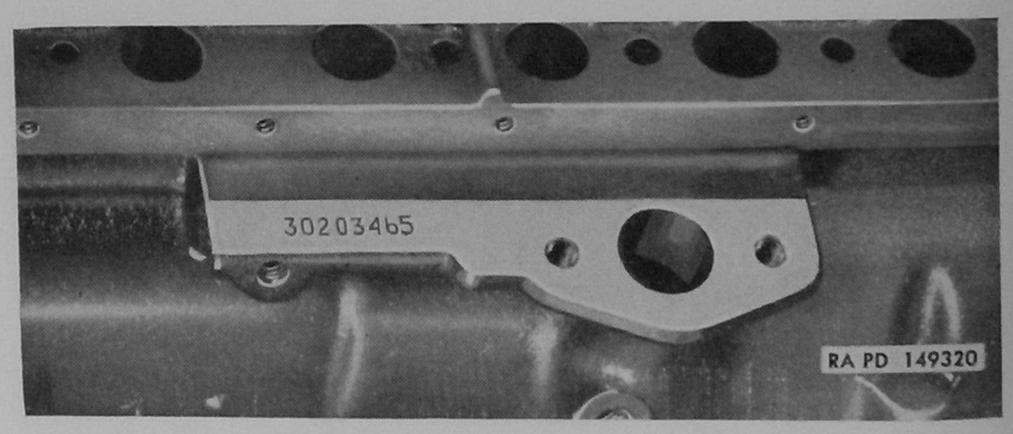
Figure 5. Location of engine serial number stamped on block.
