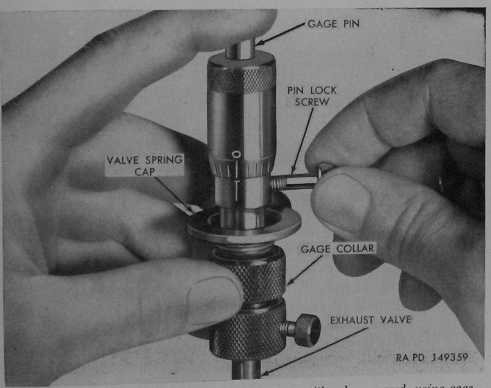
Figure 160. Checking valve rotator cap clearance with valve removed, using gage kit 7950601.
