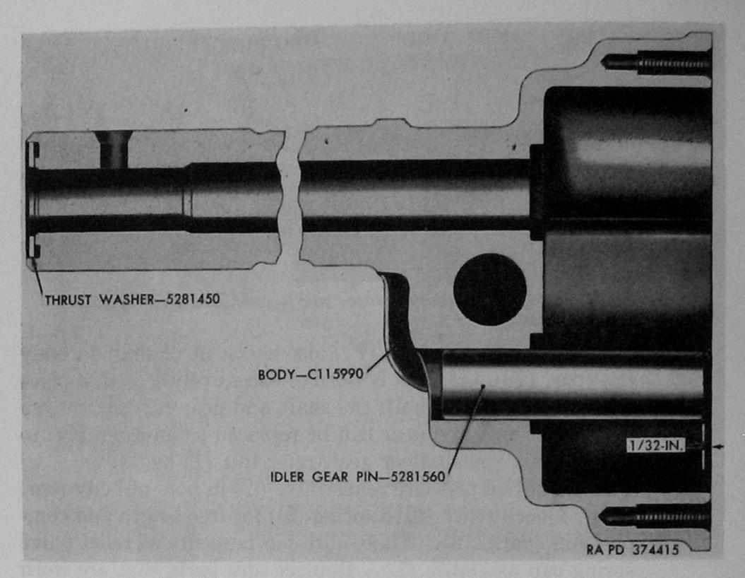
Figure 93. Oil pump body, idler gear pin, and thrust washer assembled.
