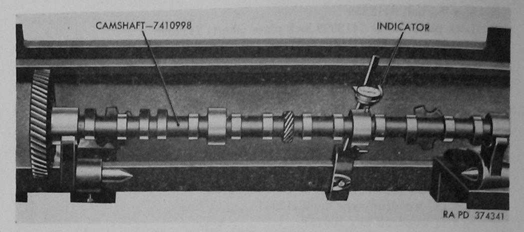
Figure 111. Checking camshaft for runout.
