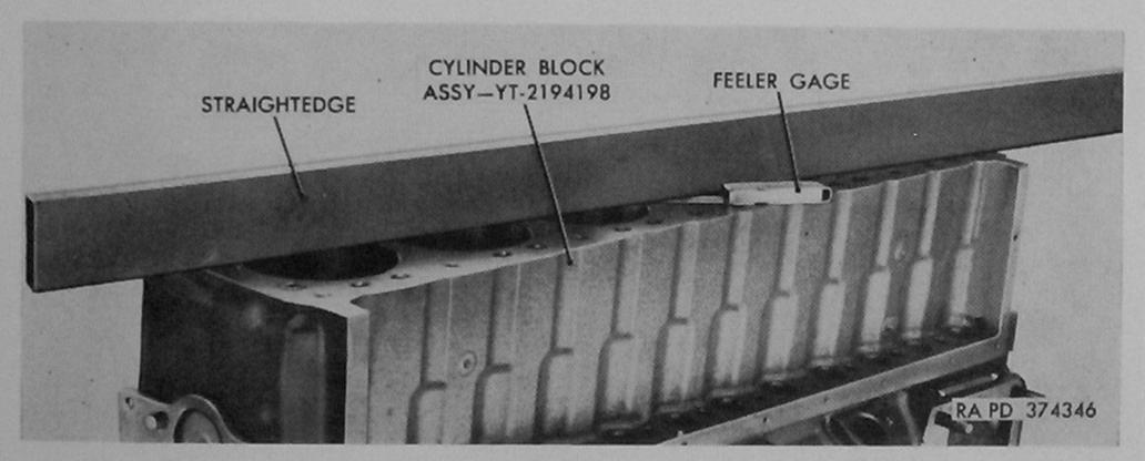
Figure 120. Checking flatness of top of cylinder block.
