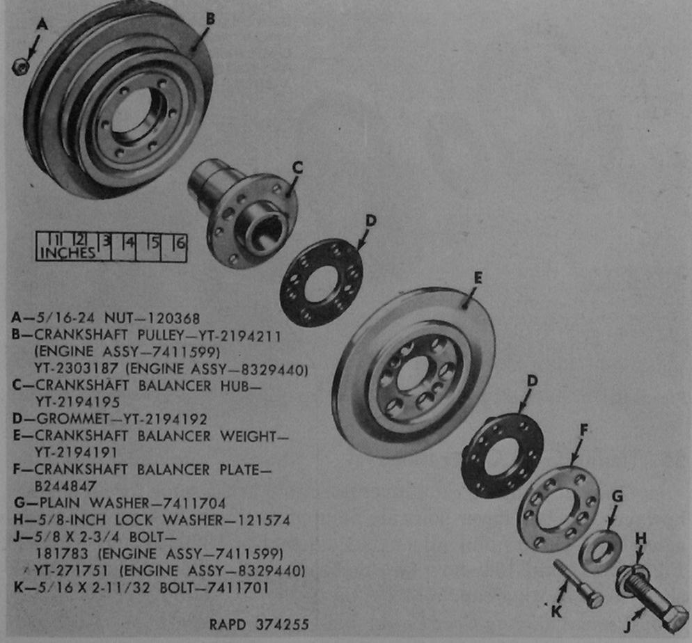
Figure 63. Crankshaft pulley and balancer components—engine assemblies 7411599 and 8329440.
