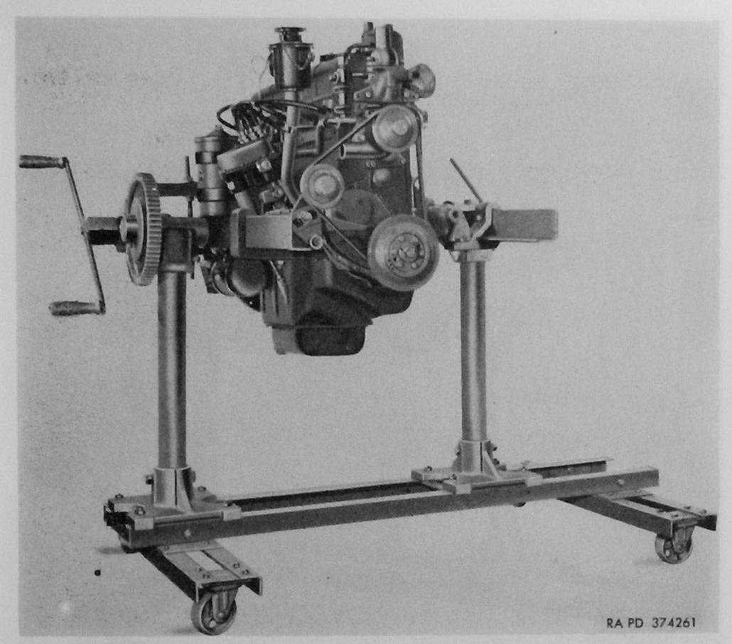
Figure 12. Engine assembly 8329440 in repair stand.
