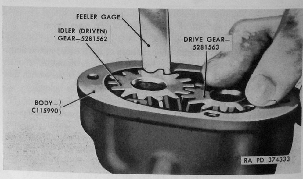
Figure 90. Checking oil pump gear to body clearance.
