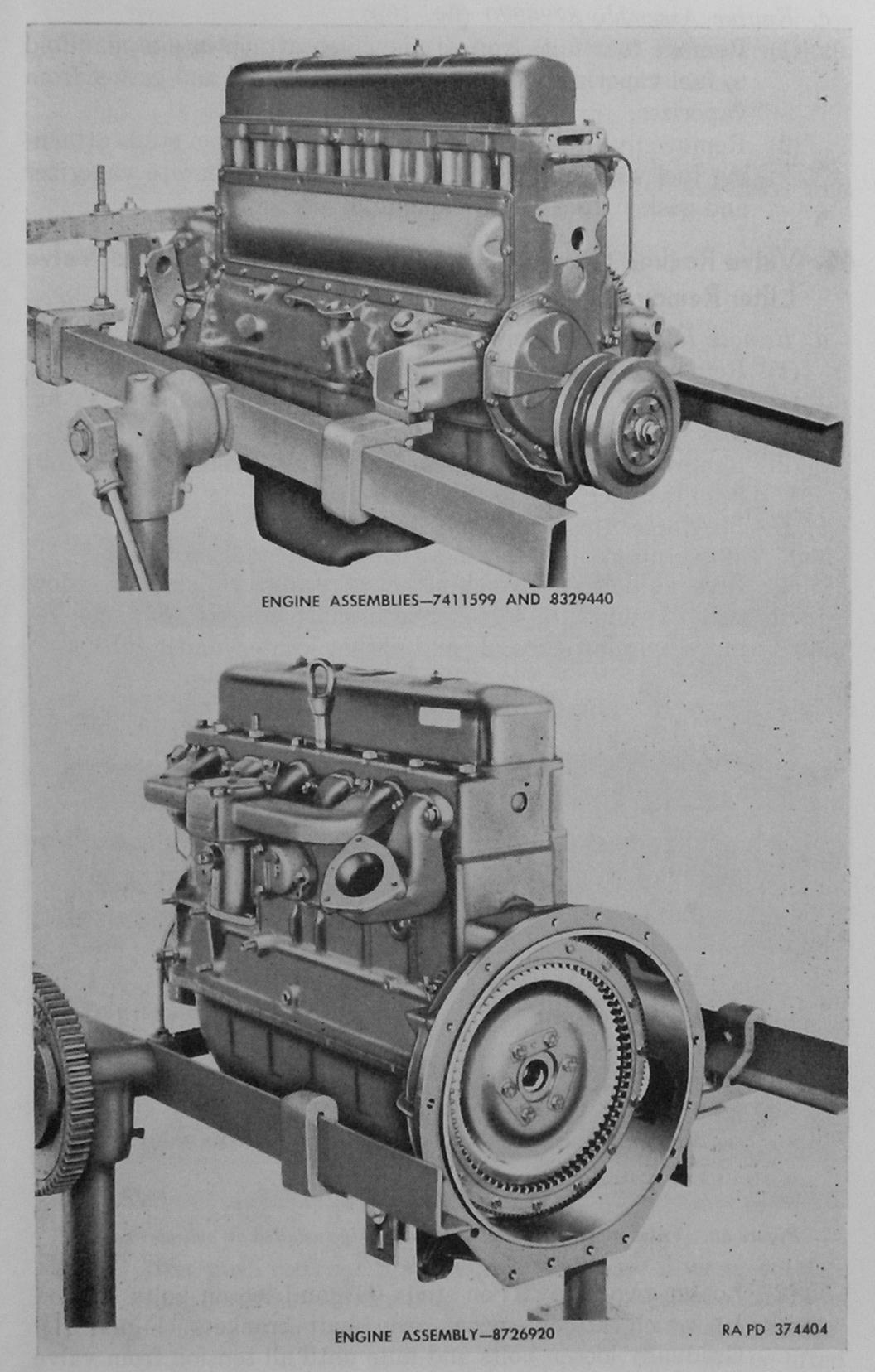
Figure 49. Stripped engine assemblies mounted in repair stand.
