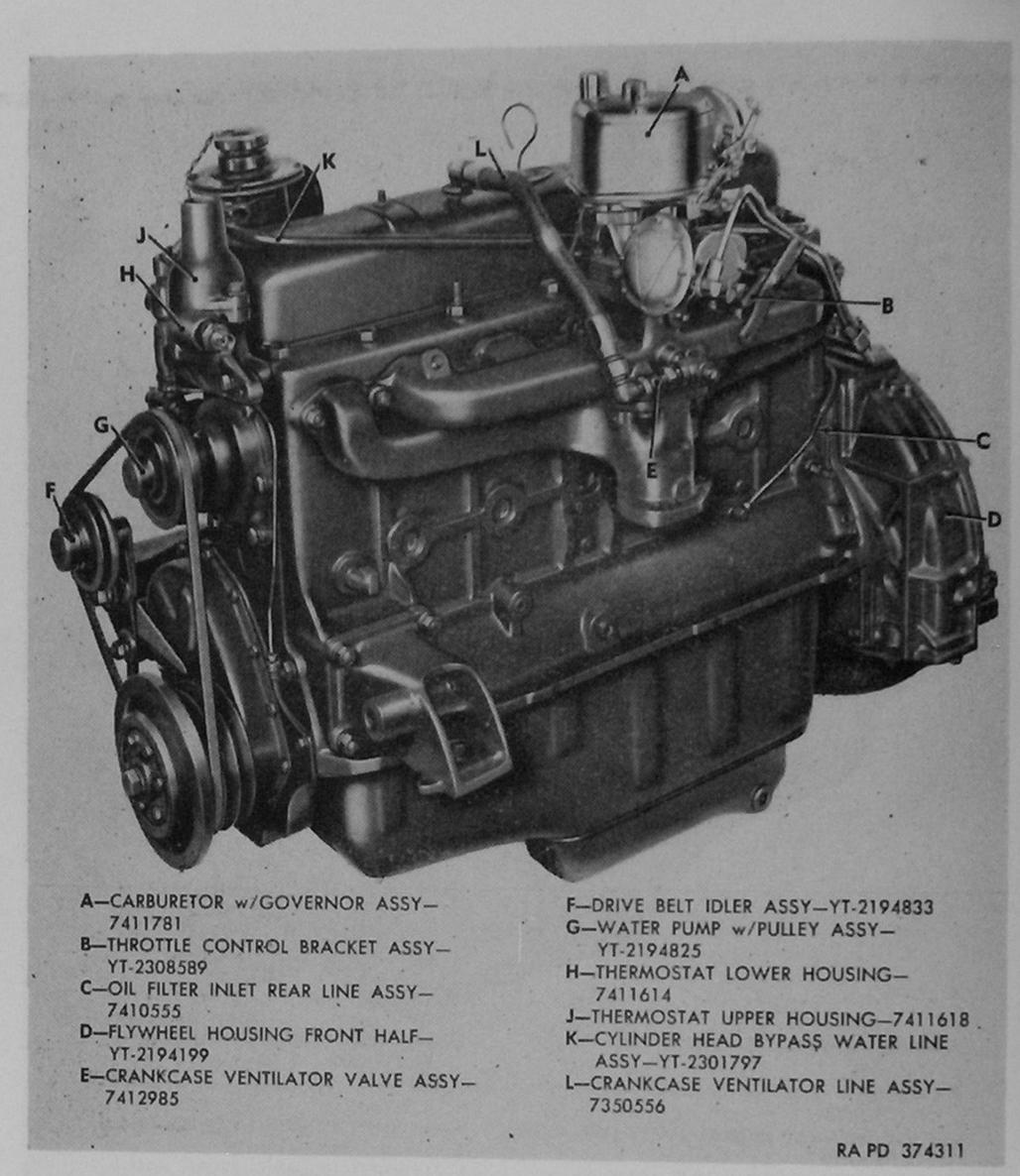
Figure 21. Engine assembly 8329440—left front view.
