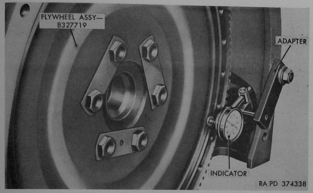
Figure 147. Checking flywheel runout-engine assemblies 7411599 and 8329440 shown.
