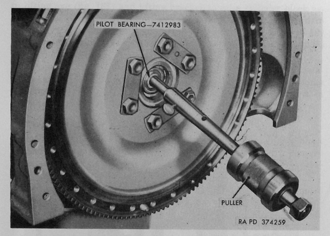
Figure 69. Removing pilot bearing assembly from crankshaft using puller 7077742.
