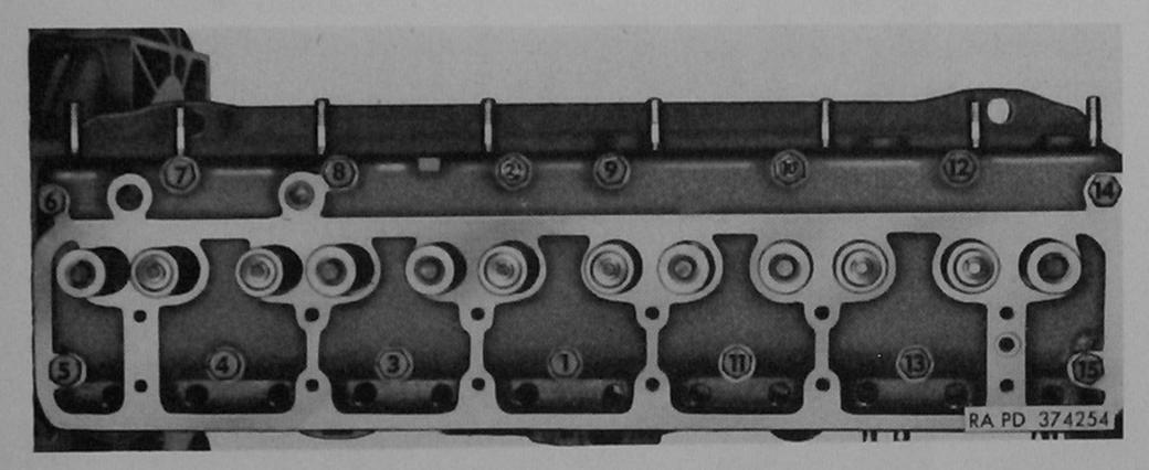
Figure 164. Cylinder head bolt tightening sequence.
