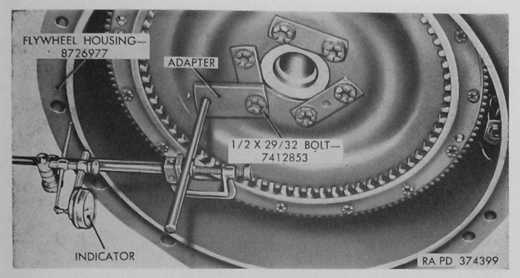
Figure 144. Checking pilot flange on flywheel housing—engine assembly 8726920
