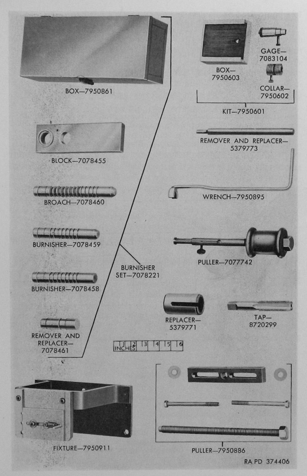
Figure 8. Special tools and equipment for field and depot maintenance.
