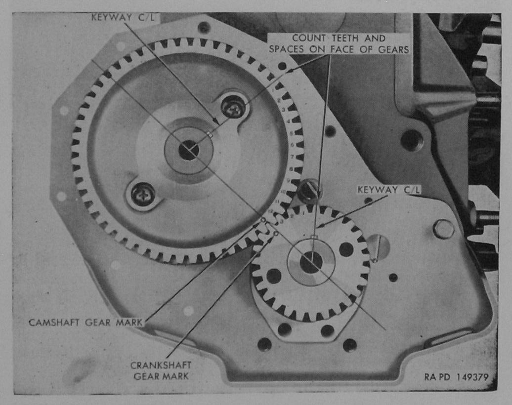
Figure 132. Location of timing marks on timing gears.
