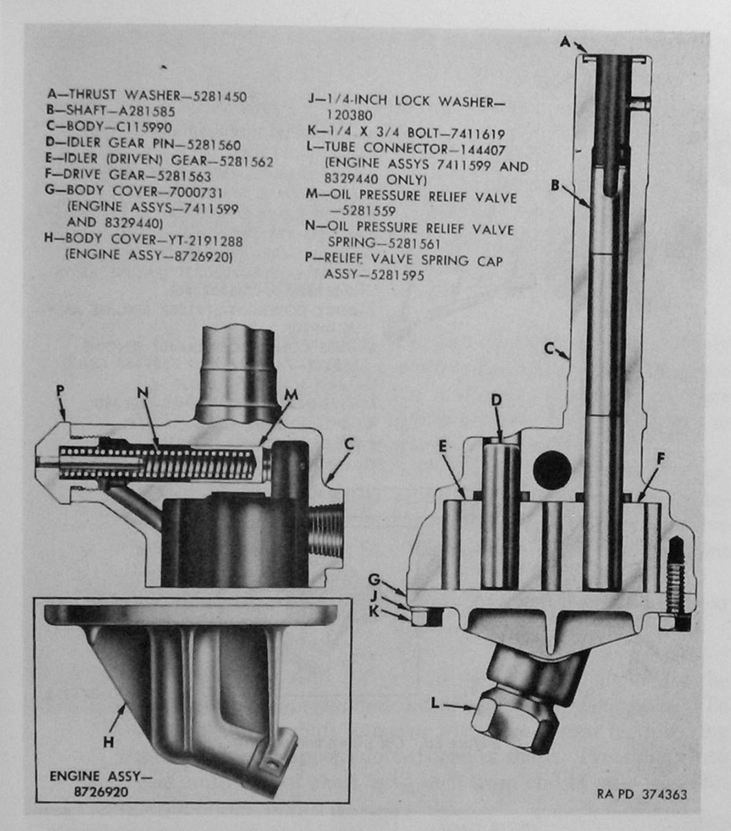
Figure 88. Oil pump assembly.
