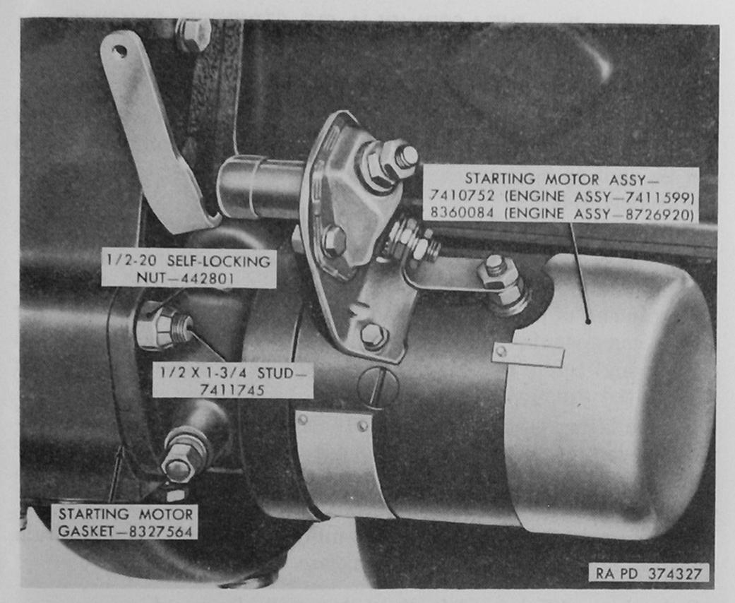
Figure 47. Starting motor ass.embly installed—engine assemblies 7411599 and 8726920
