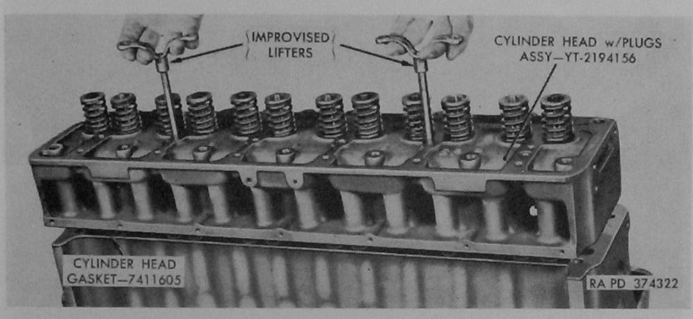
Figure 53. Removing cylinder head with plugs assembly, using improvised lifters.
