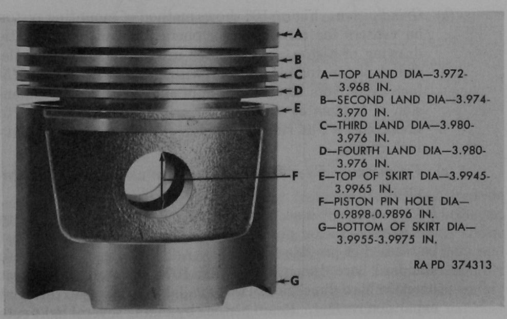
Figure 107. Standard piston dimensions.
