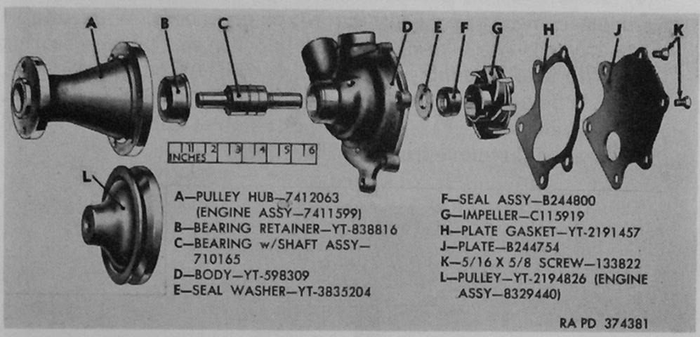
Figure 81. Water pump components—engine assemblies 7411599 and 8329440.
