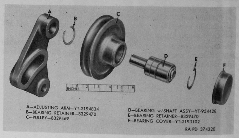
Figure 71. Drive belt idler assembly components—engine assembly 8329440.
