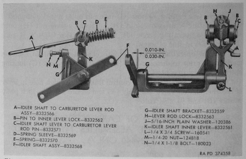
Figure 76. Carburetor throttle control bracket assembly—engine assembly 8329440 and late engine assembly 7411599.
