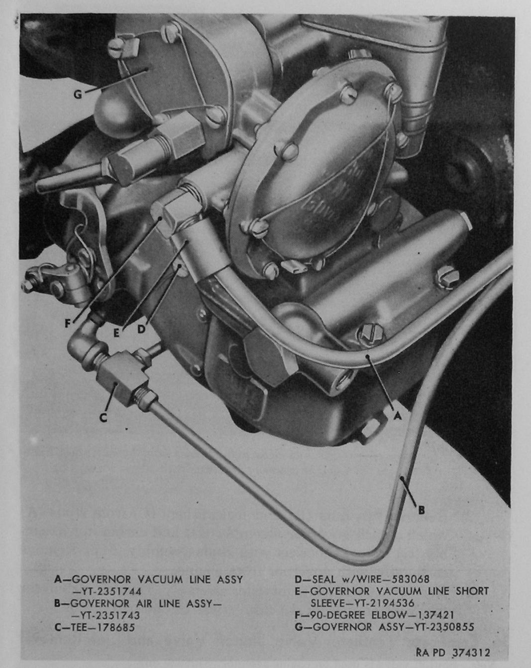
Figure 38. Governor line connections at carburetor and governor—engine assembly 8726920.
