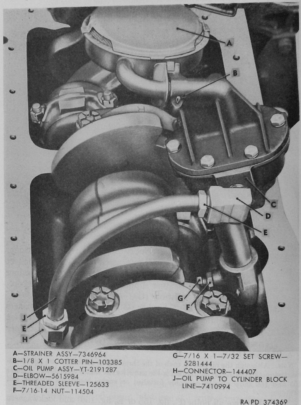
Figure 58. Oil pump and strainer assembly installed—engine assembly 8726920.
