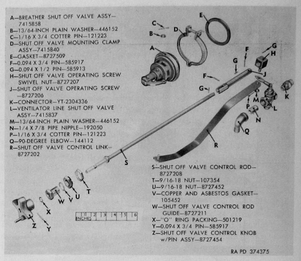
Figure 74. Breather valve and crankcase shutoff valve components—engine assembly 8726920.
