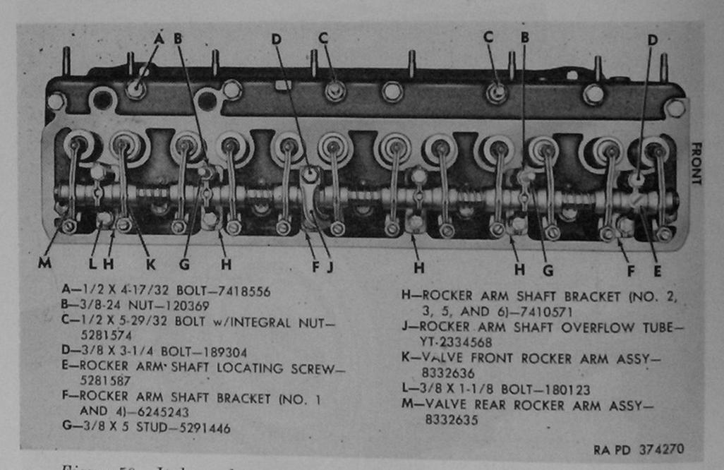
Figure 50. Valve rocker arm and shaft assembly installed on cylinder head.
