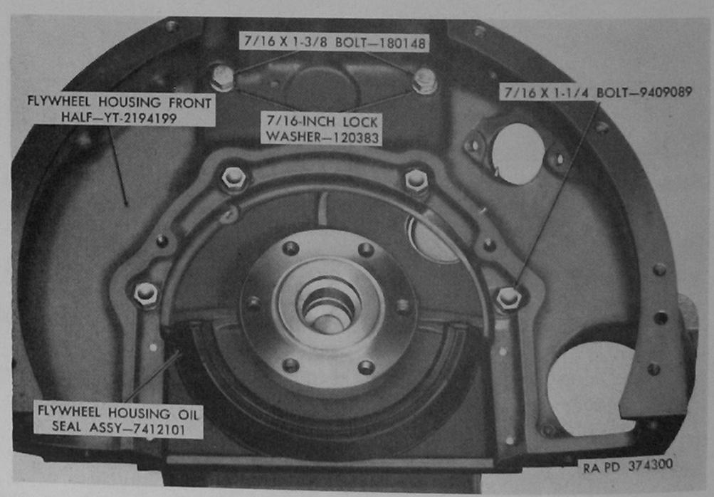
Figure 139. Flywheel housing front half installed—engine assemblies 7411599 and 8329440 shown.
