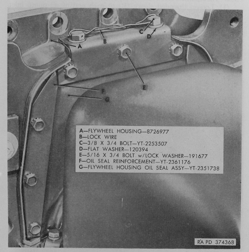
Figure 55. Flywheel housing oil seal assembly installed—engine assembly 8726920.
