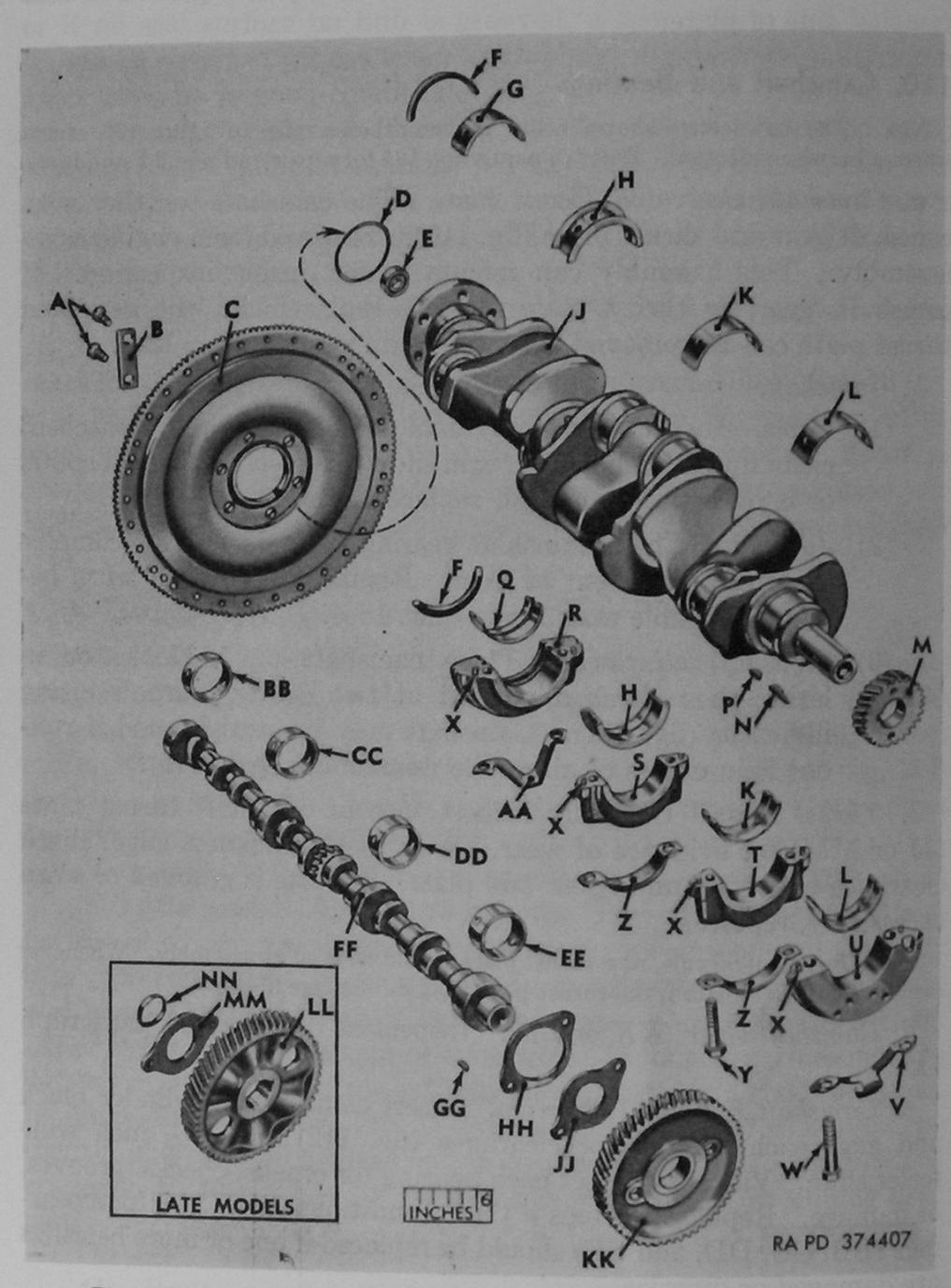
Figure 109. Crankshaft, camshaft, bearings, and timing gear components.
