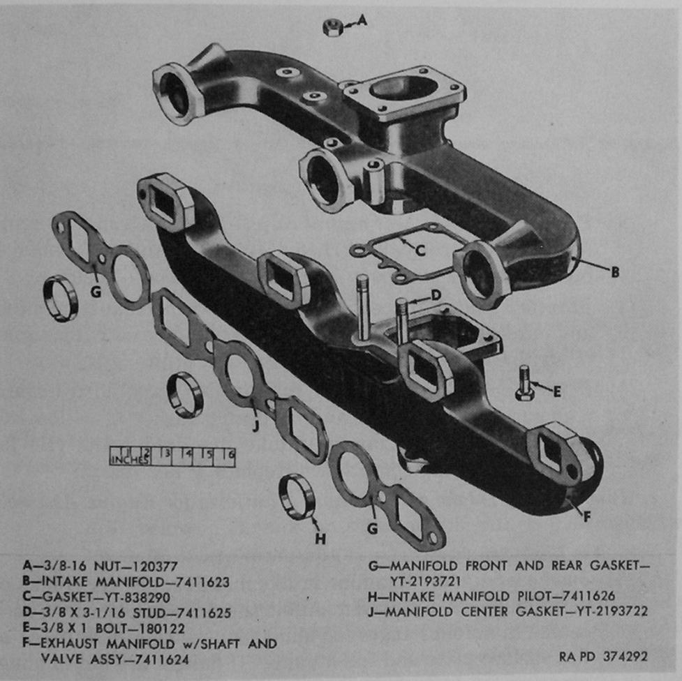
Figure 97. Intake and exhaust manifold components—engine assemblies 7411599 and 8329440.
