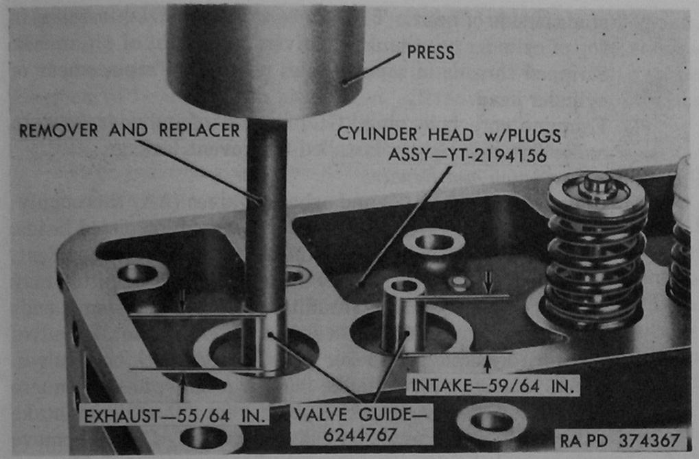
Figure 103. Installing valve guides in cylinder head using remover and replacer 5379773.
