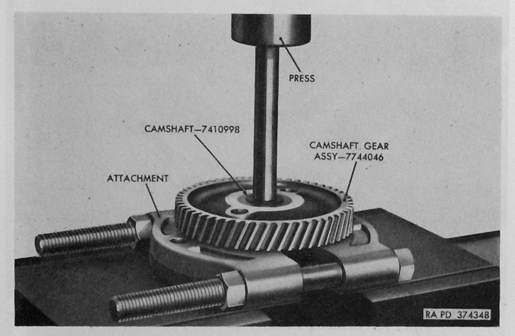
Figure 67. Removing camshaft gear from camshaft (early engine assembly 7411599 shown).
