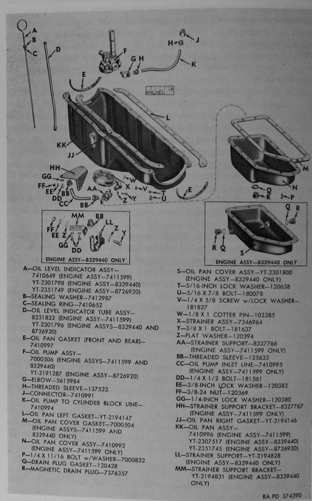
Figure 105. Engine oil pan, cover, and associated components.
