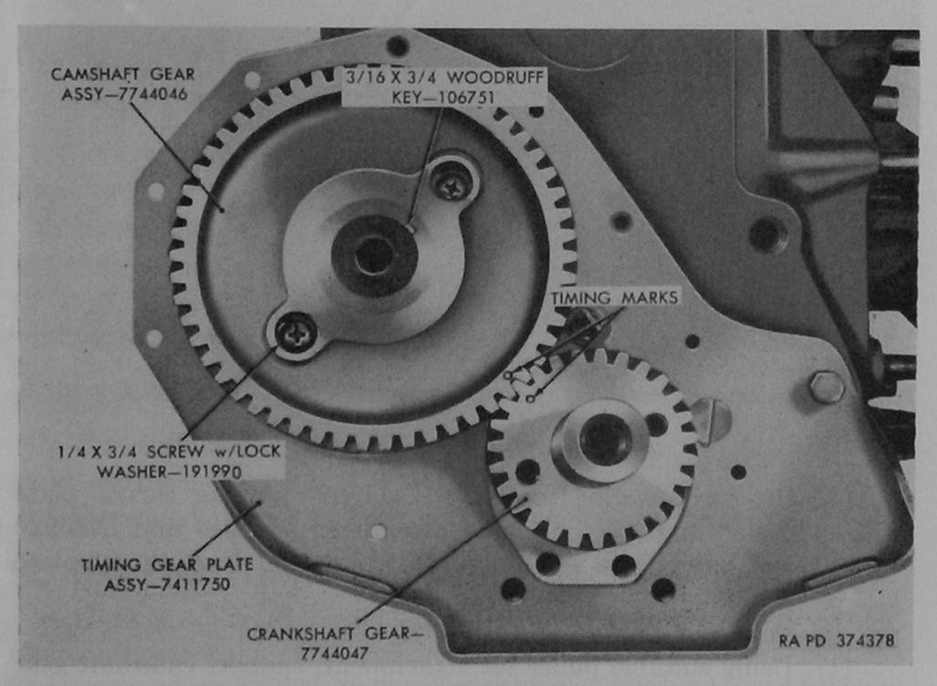
Figure 65. Timing gears with cover removed (early engine assembly 7411559 shown).
