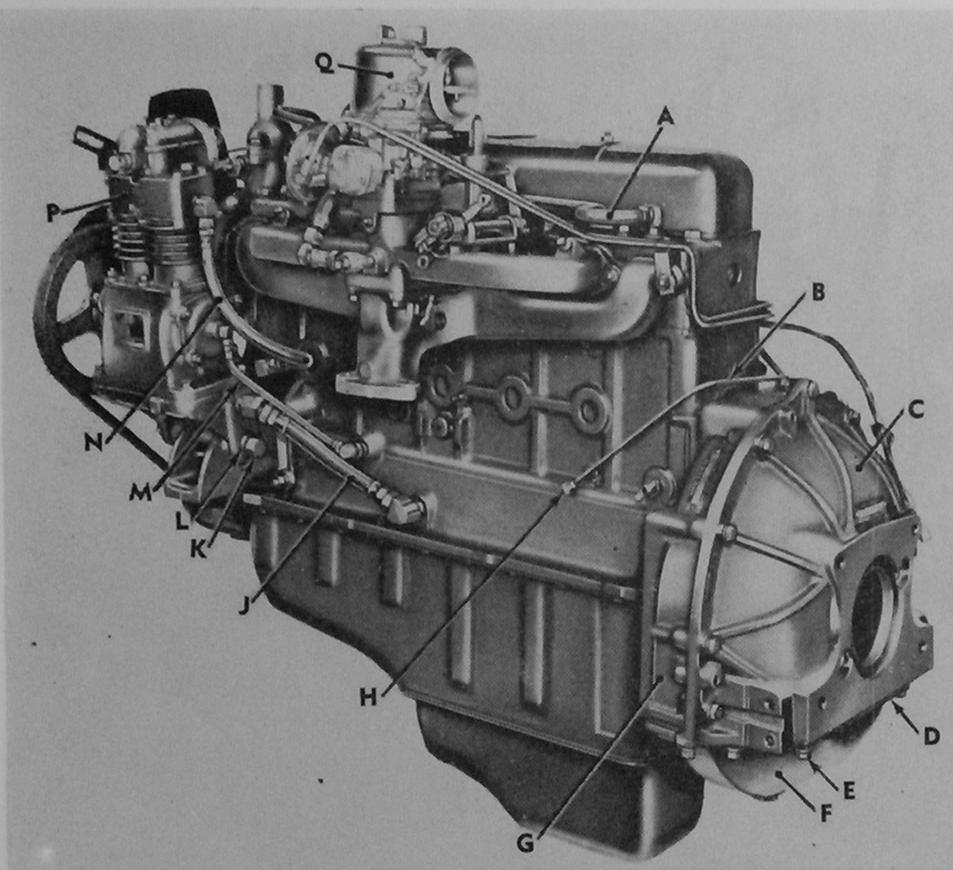
A-CYLINDER HEAD BYPASS WATER LINE ASSY-7411615
