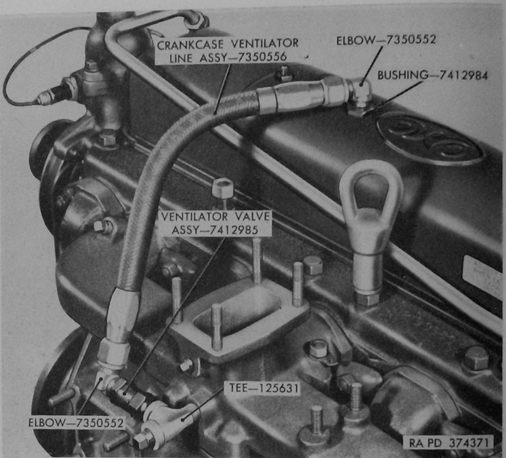
Figure 43. Crankcase ventilator line and valve installed—engine assemblies 7411599 and 8329440.
