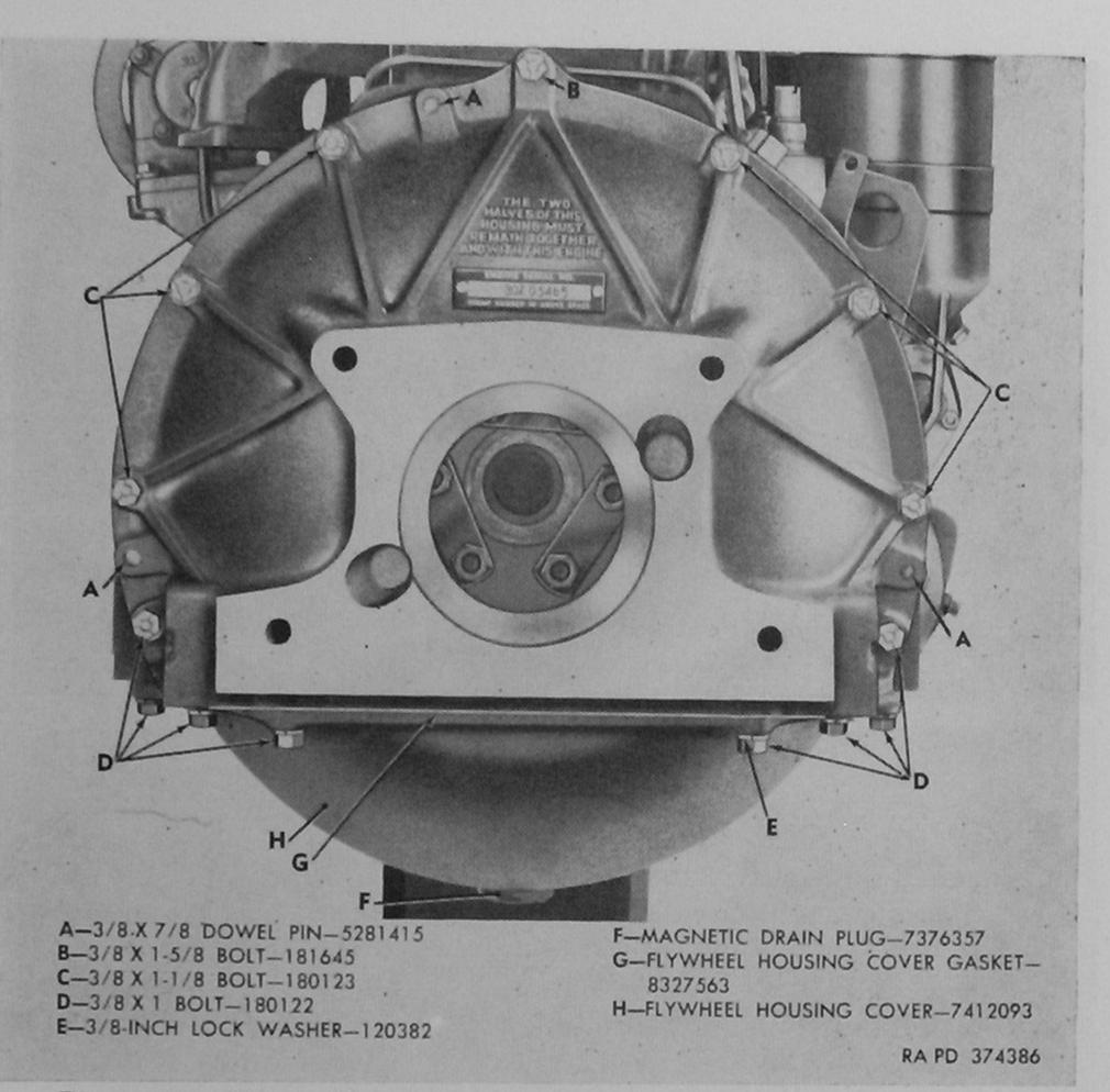
Figure 141. Flywheel housing rear half installed—engine assemblies 7411599 and 8329440.
