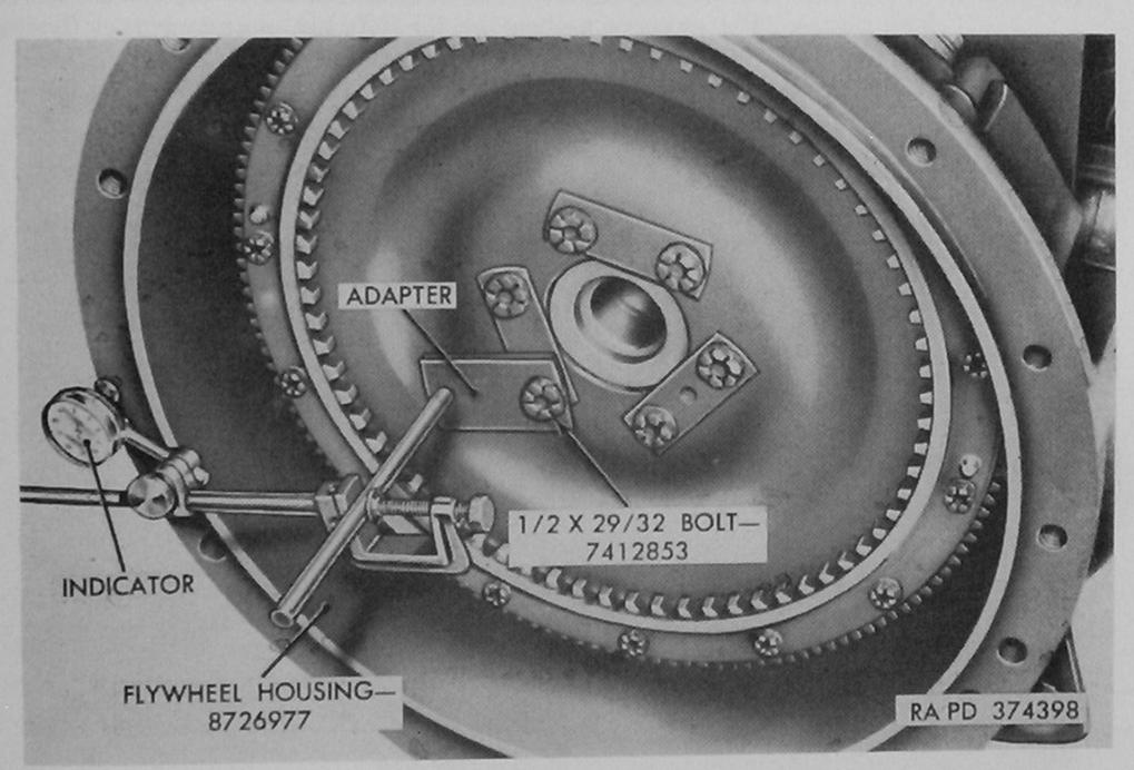
Figure 145. Checking squareness of rear face of flywheel housing—engine assembly 8726920.
