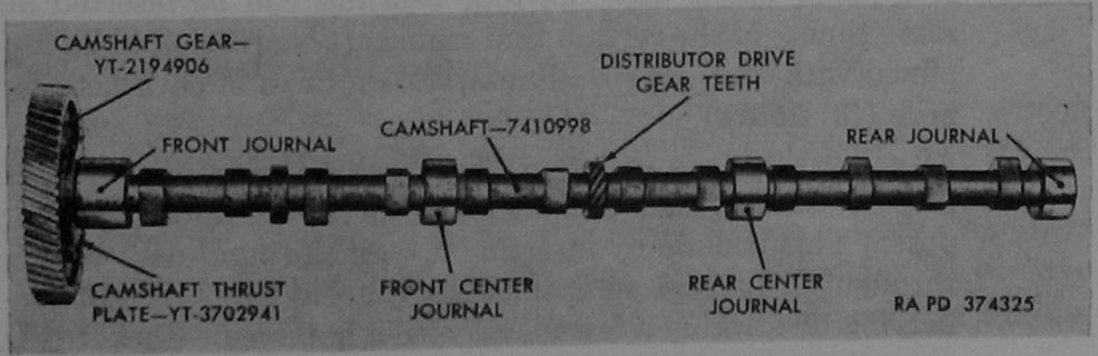
Figure 110. Camshaft, gear, and thrust plate.
