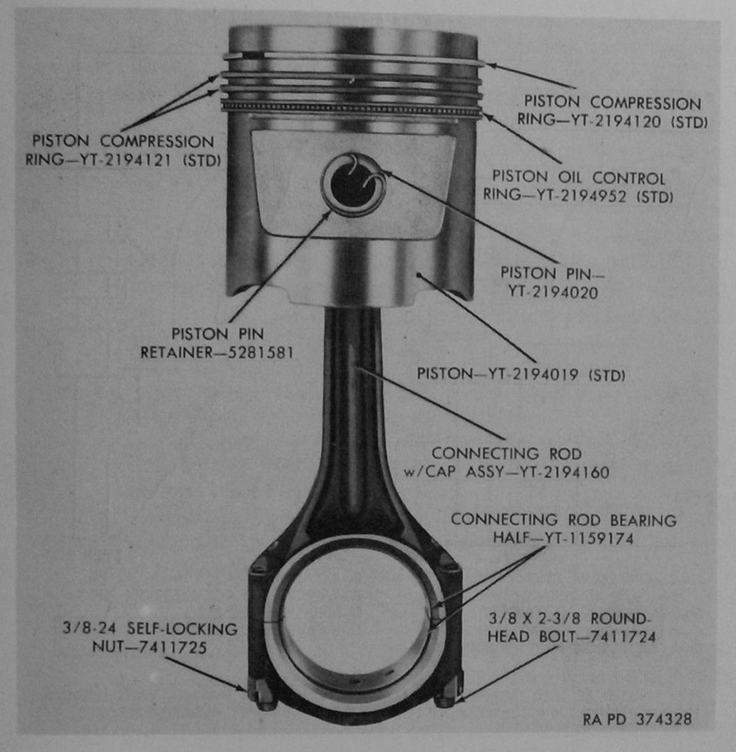
Figure 151. Piston and connecting rod assembly.
