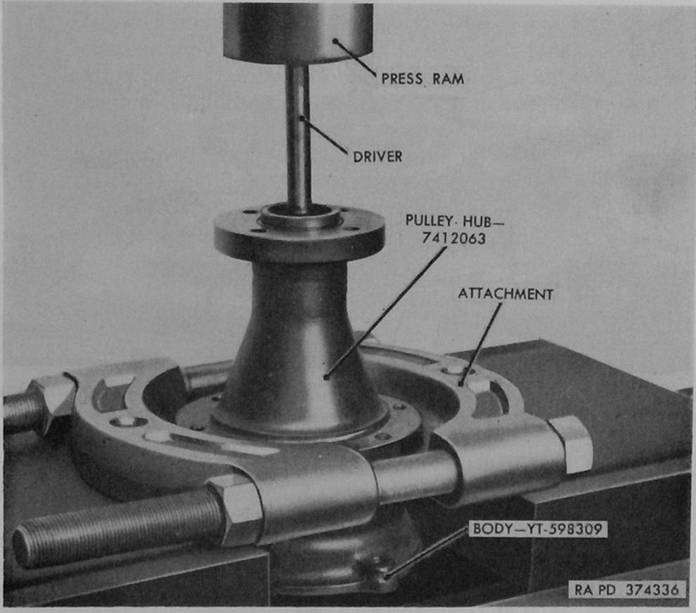
Figure 82. Removing water pump pulley hub—engine assembly 7411599.
