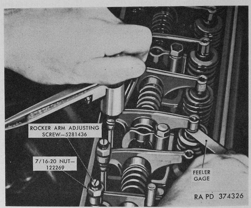
Figure 166. Adjusting valve clearance.
