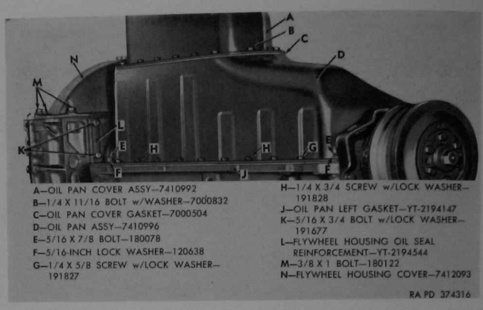
Figure 156. Oil pan and cover, and flywheel housing cover installed—engine assembly 7411599.
