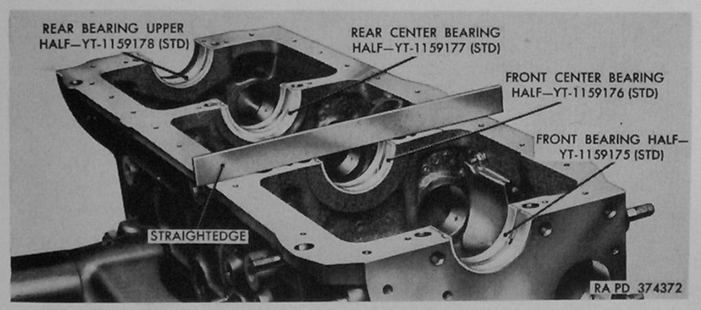
Figure 126. Checking for correct position of crankshaft bearing halves with straightedge.
