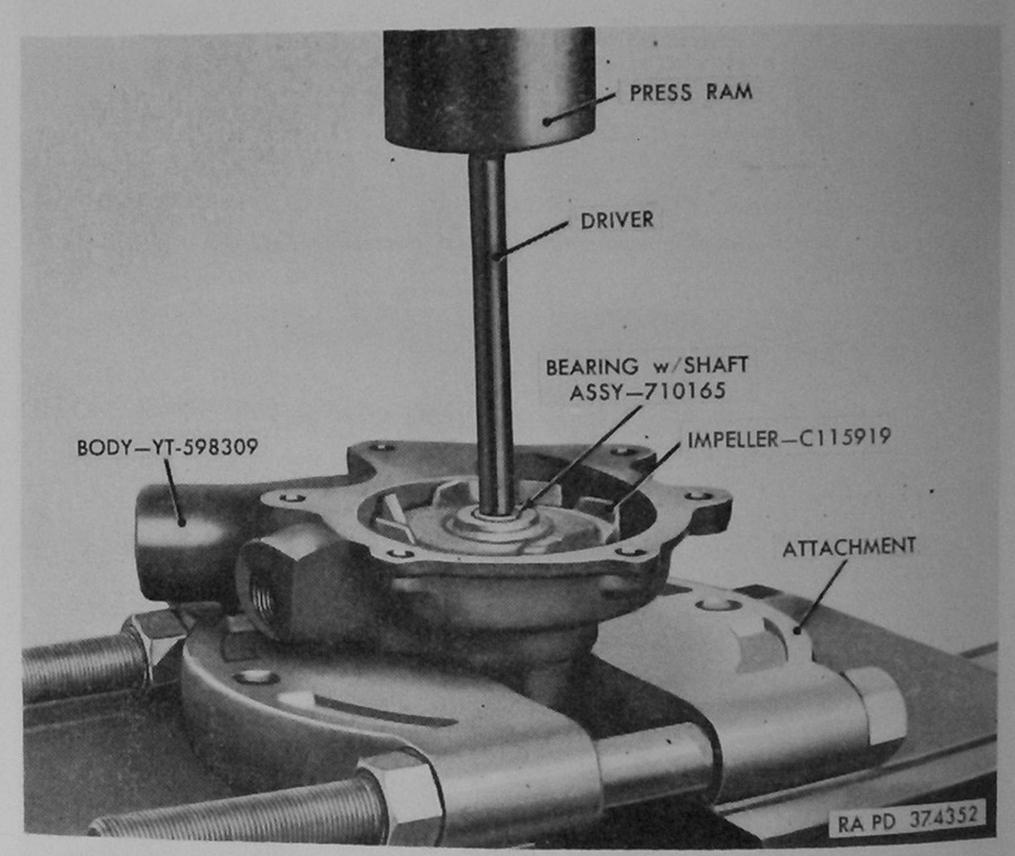
Figure 83. Pressing bearing with shaft assembly from water pump impeller—engine assemblies 7411599 and 8329440.
