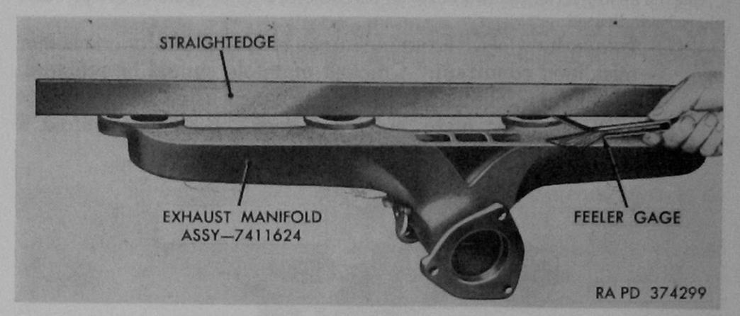
Figure 98. Checking alinement of manifold flanges—engine\_assemblies 7411599 and 8329440.
