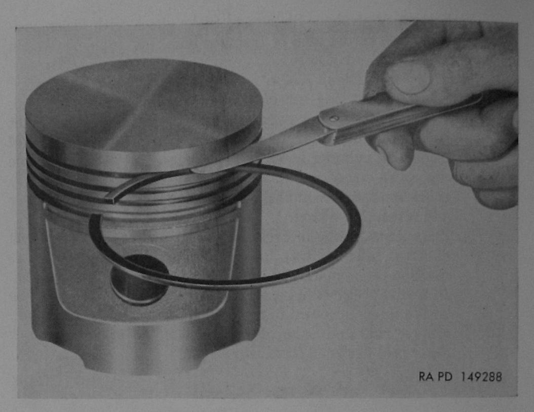
Figure 150. Checking piston ring to groove clearance.
