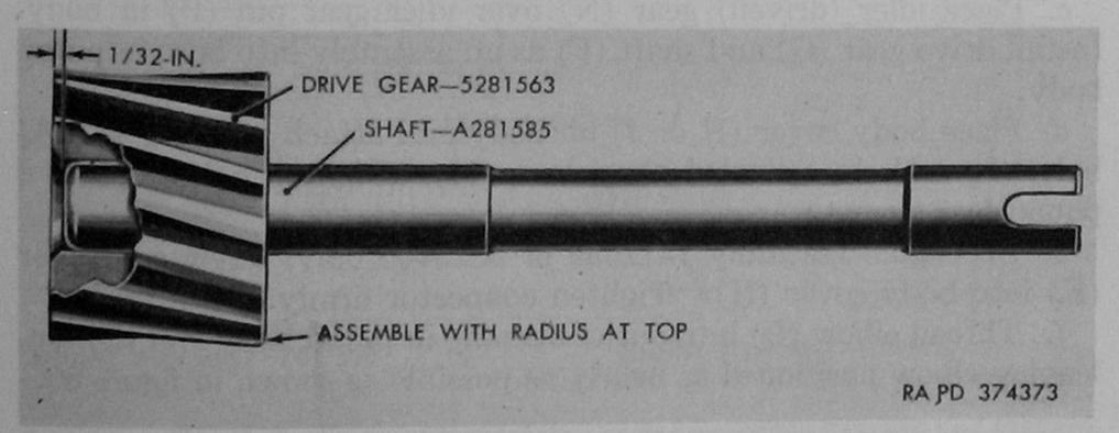
Figure 92. Oil pump shaft with drive gear assembled.
