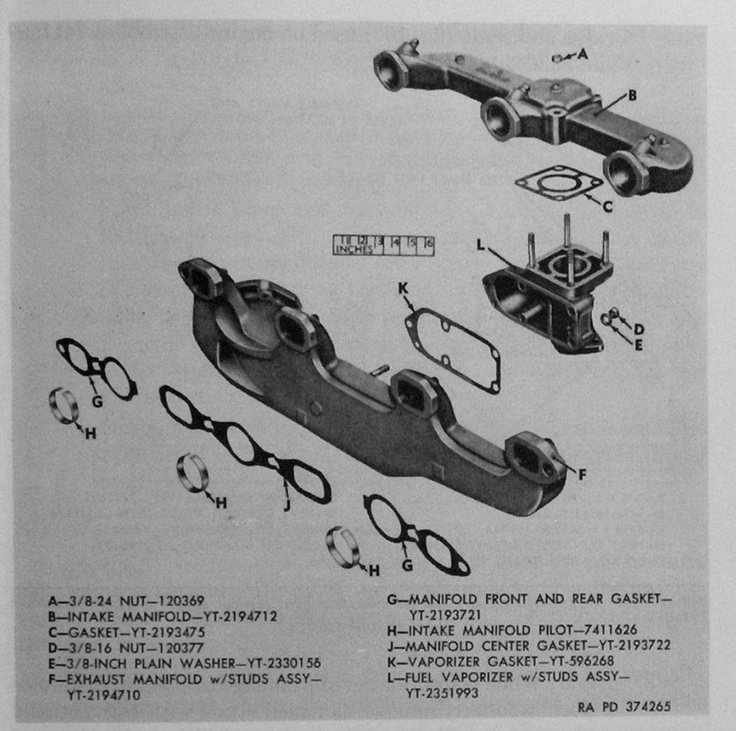
Figure 99. Intake and exhaust manifold components—engine assembly 8726920.
