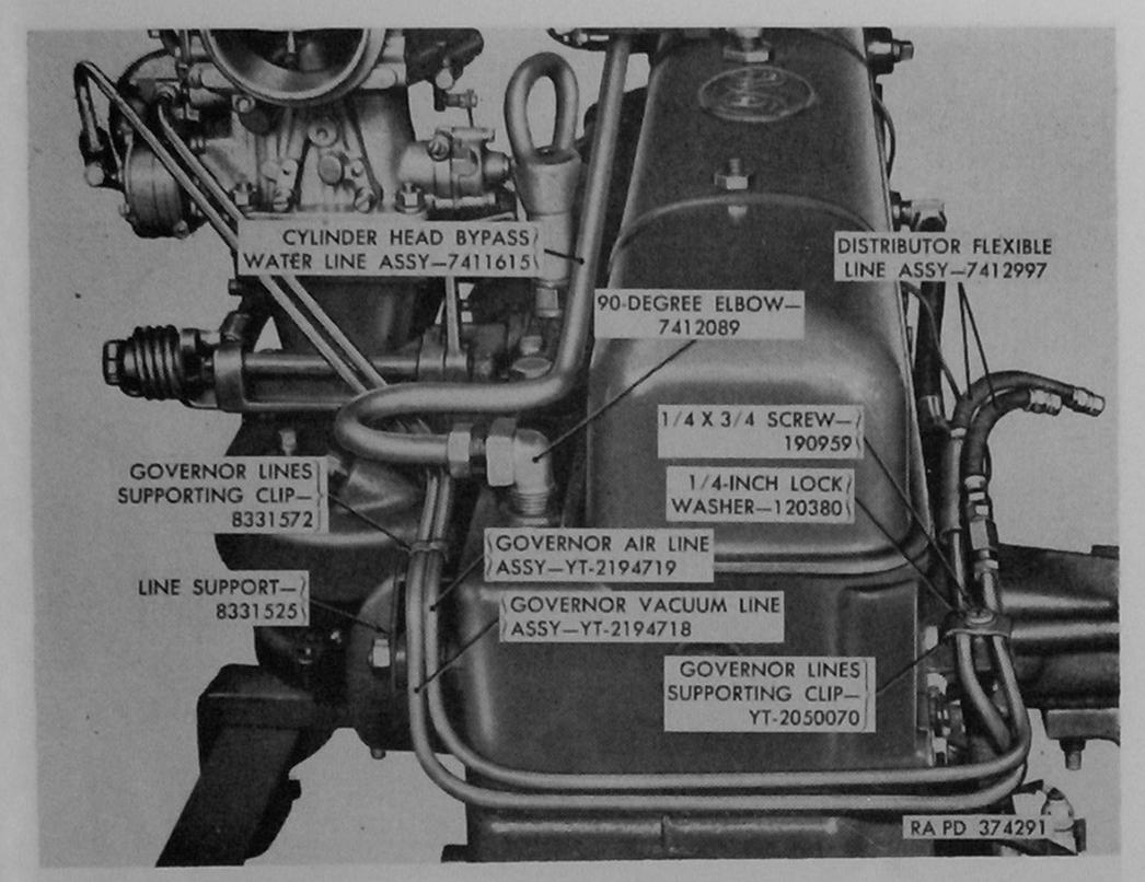
Figure 36. Location of governor line clips and cylinder head bypass water line—engine assembly 7411599.
