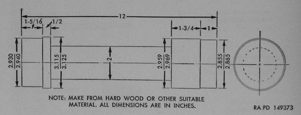
Figure 9. Improvised mandrel for installing crankshaft bearing oil seals.
