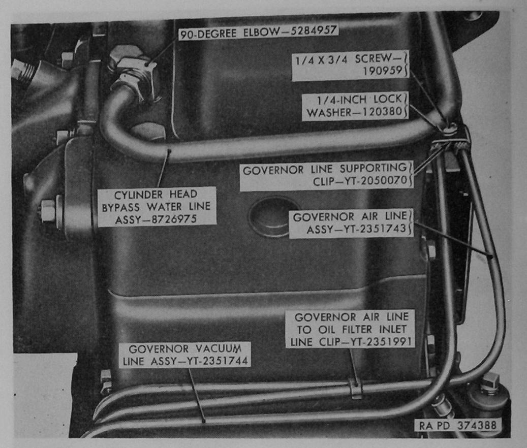
Figure 39. Location of governor line clips and cylinder head bypass water line—engine assembly 8726920.
