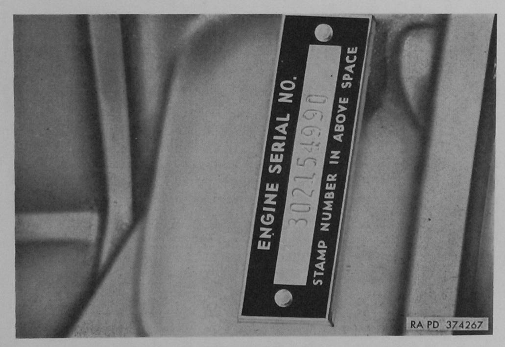
Figure 7. Location of engine serial number plate on flywheel housing—enging assembly 8726920.
