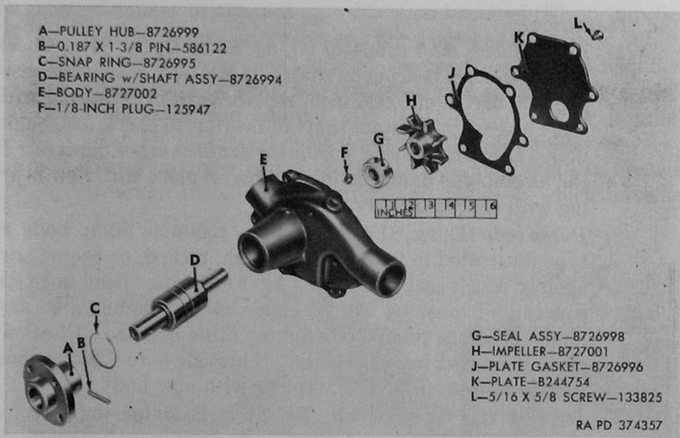
Figure 84. Water pump components—engine assembly 8726920.
