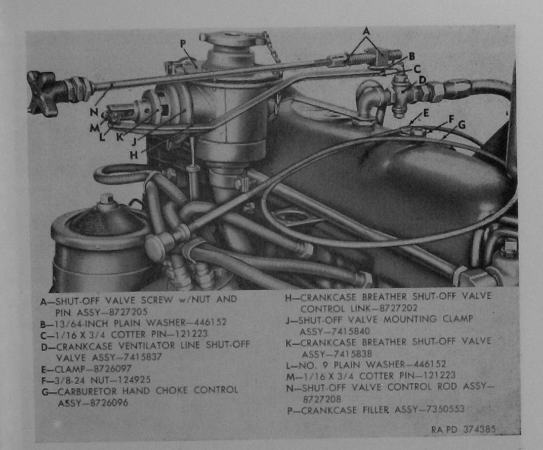
Figure 28. Breather valve, crankcase shutoff valve, and carburetor hand choke assembly installed—engine assembly 8726920.
