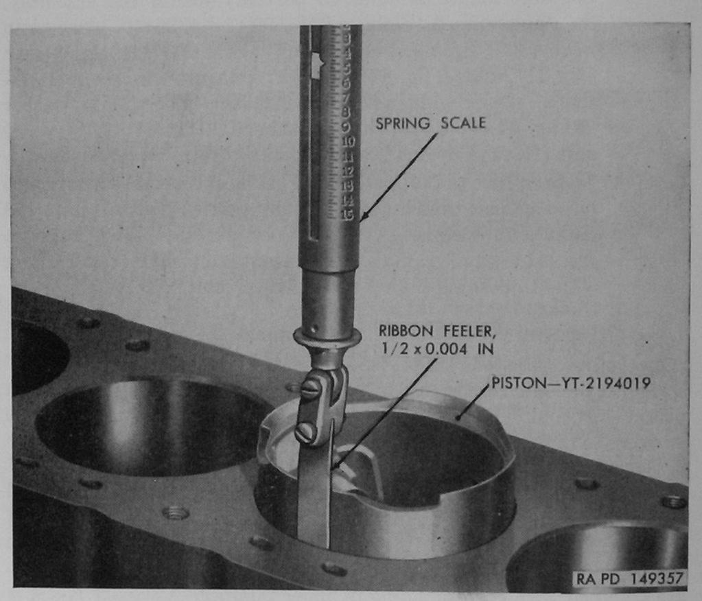
Figure 148. Method of checking piston fit in cylinder bore.
