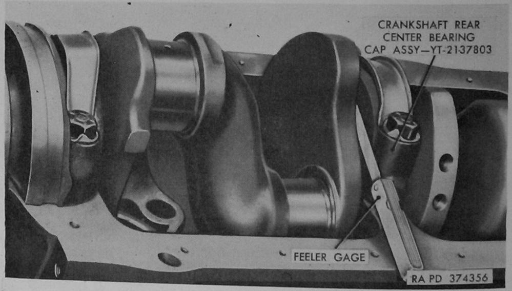
Figure 127. Measuring crankshaft end play.
