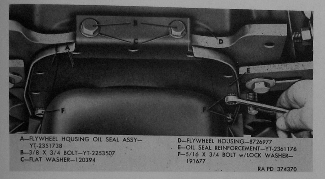
Figure 158. Installing flywheel housing oil seal assembly on engine assembly 8726920.
