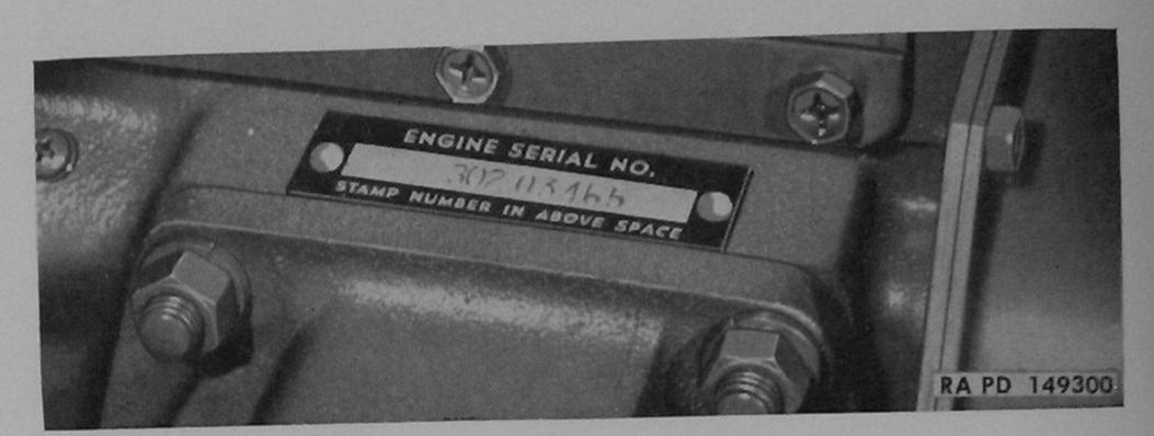
Figure 4. Location of engine serial number plate.
