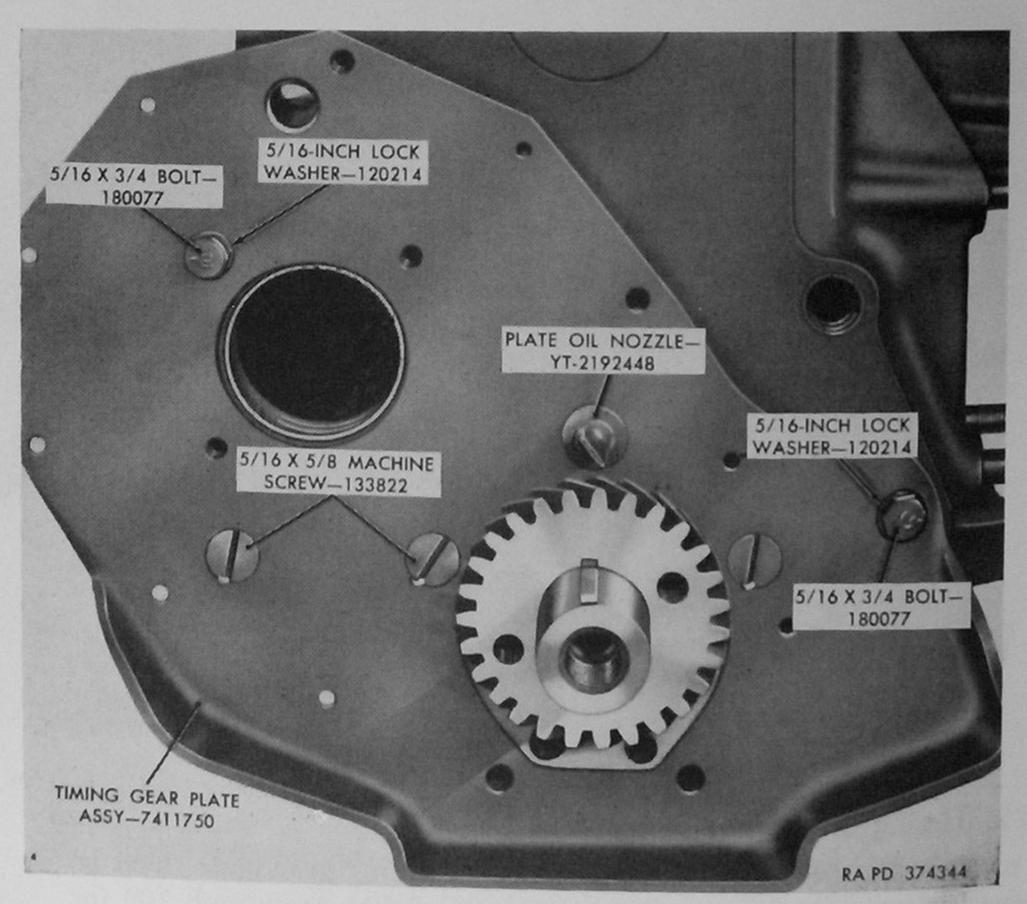
Figure 129. Timing gear cover plate installed on cylinder block.
