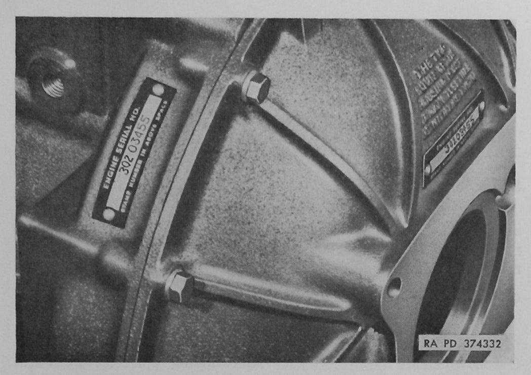
Figure 6. Location of engine serial number plates on flywheel housing halves—engine assemblies 7411599 and 8329440.
