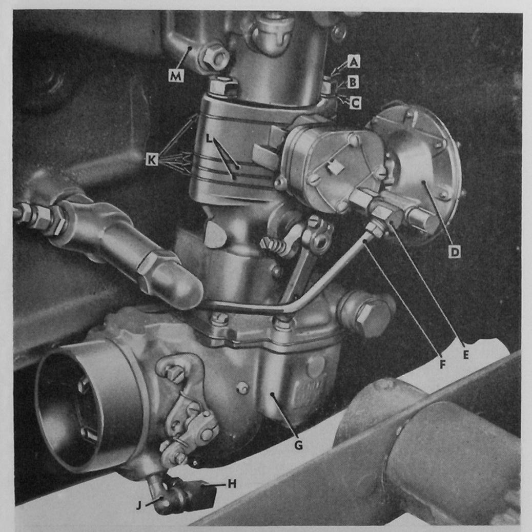
A-7/16 X 3-5/16 STUD-YT-063827 B-7/16-20 NUT-120370 C-7/16-INCH LOCK WASHER-120383
