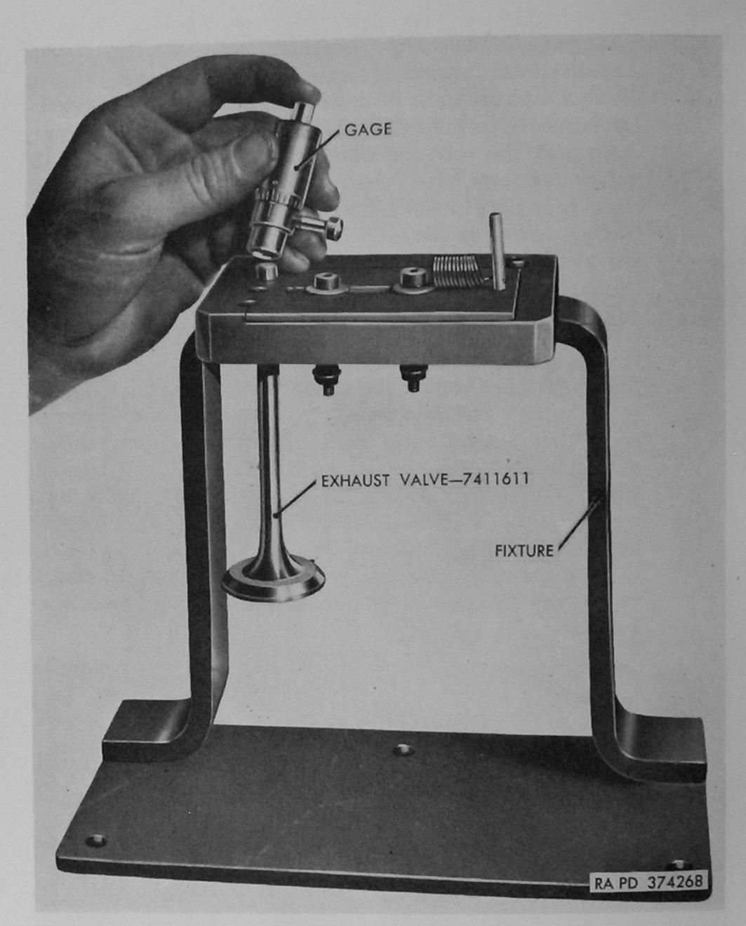
Figure 161. Use of fixture 7950911 with gage 7083104.
