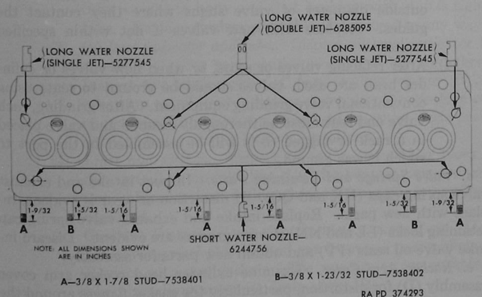
Figure 104. Cylinder head water nozzle identification (early engine assembly 7411599 only) and manifold stud driven height.
