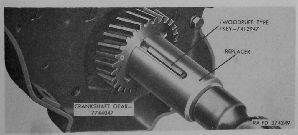
Figure 130. Installing gear on crankshaft using replacer 5379771.
