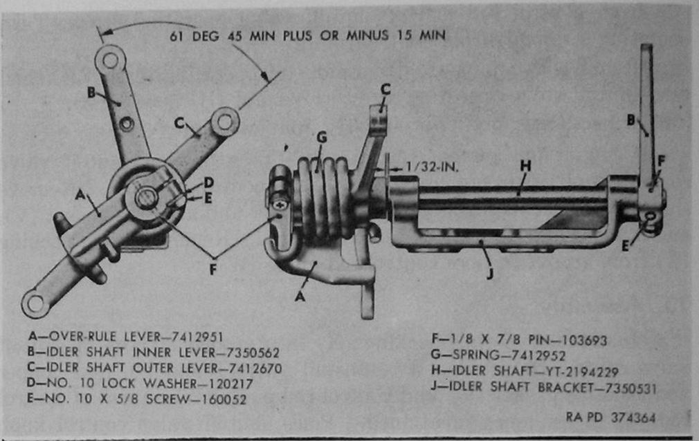
Figure 75. Carburetor throttle control bracket assembly—early engine assembly 7411599.
