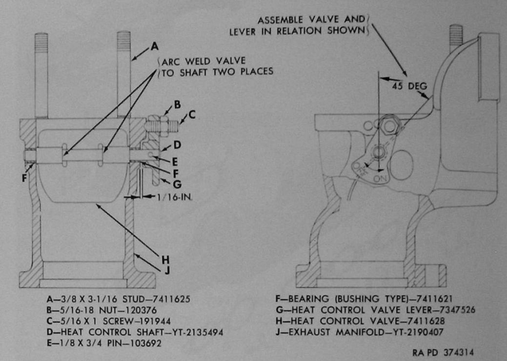
Figure 100. Sectional view of exhaust manifold heat control valve—engine assemblies 7411599 and 8329440.
