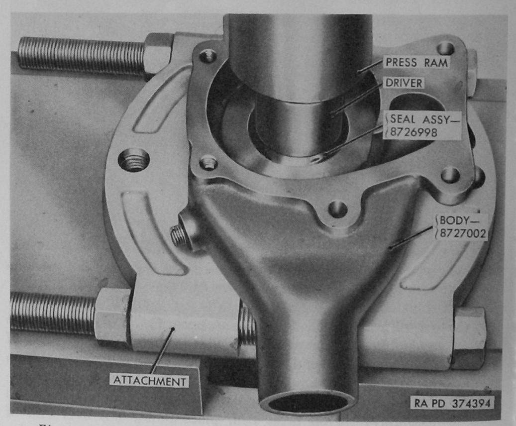
Figure 86. Installing water pump seal assembly—engine assembly 8726920.
