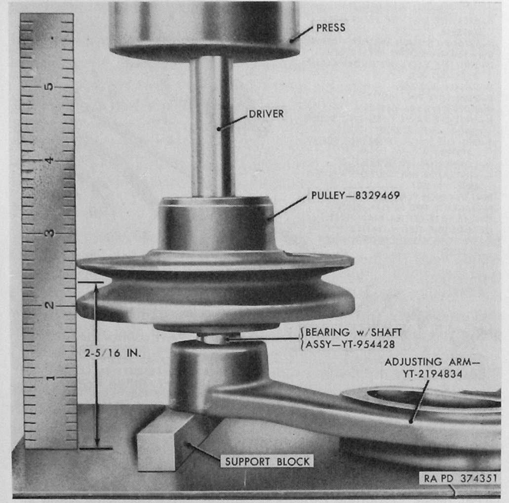
Figure 73. Pressing idler pulley and bearing with shaft assembly into adjusting armengine assembly 8329440.
