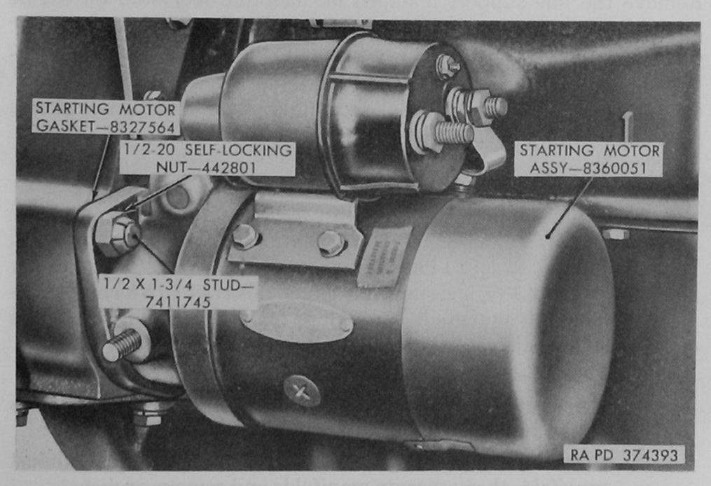
Figure 48. Starting motor assembly installed—engine assembly 8329440.
