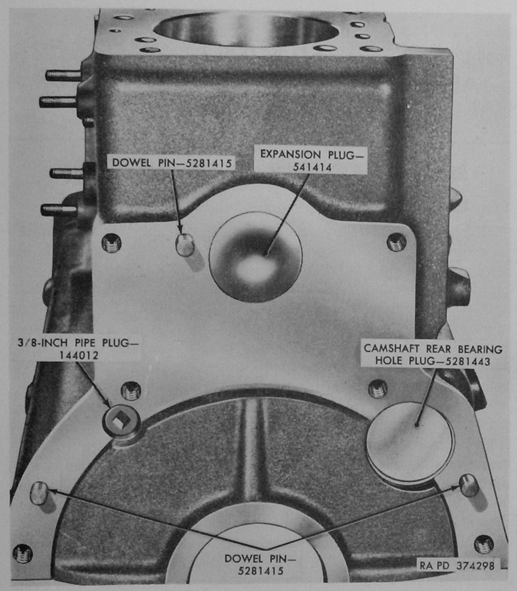
Figure 123. Rear view of cylinder block assembly (early model shown).
