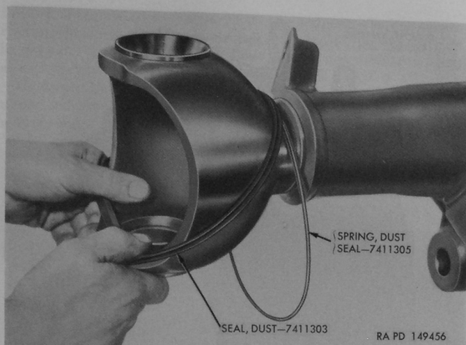
Figure 126. Housing outer dust seal and spring installation.
