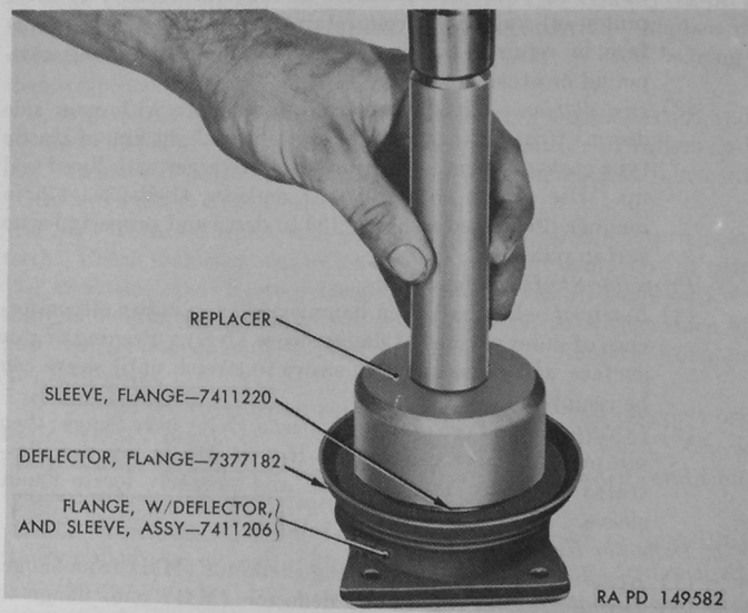
Figure 140. Flange sleeve installation with replacer 41-R-2395-515.
