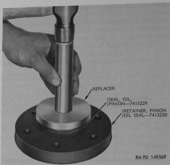
Figure 139. Drive pinion oil seal installation using replacer 41-R-2393-175.
