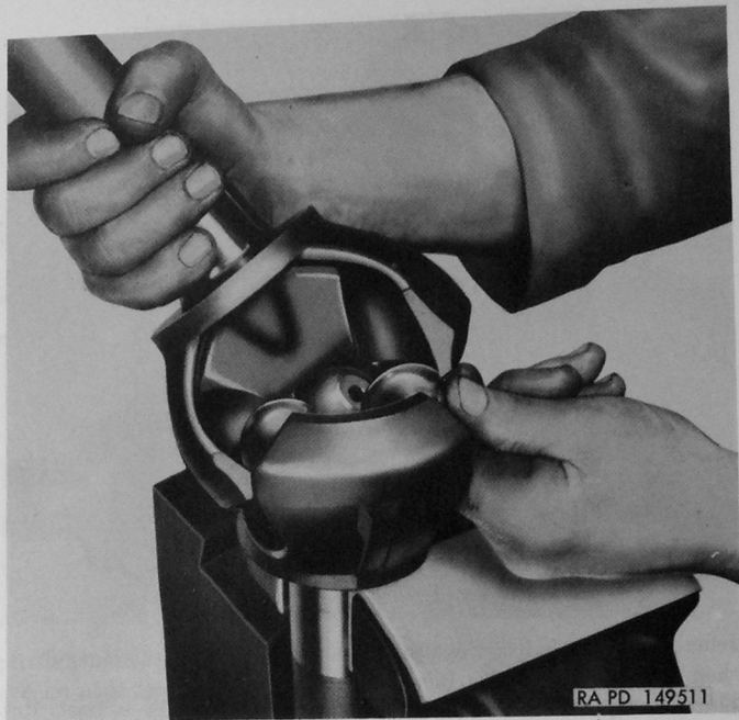
Figure 115. Universal joint outer balls removal or installation.
