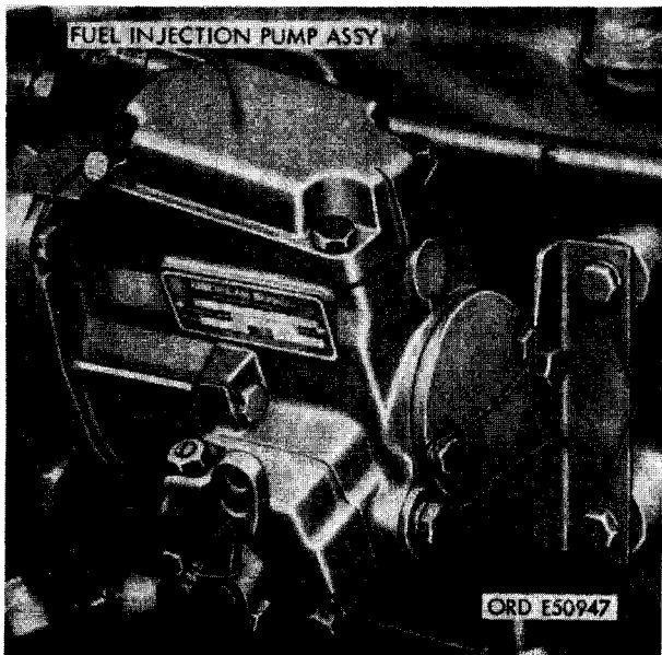
FIGURE 68. REMOVING OR INSTALLING FUEL INJECTION PUMP BRACKET (LATE MODEL ENGINES).
