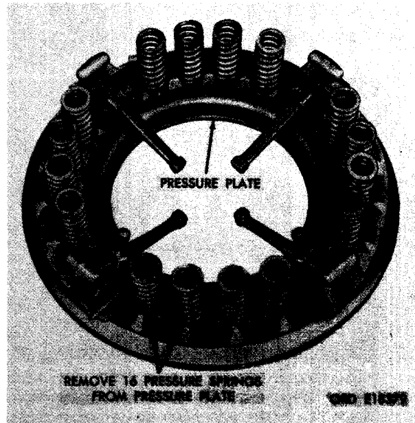
FIGURE 452. REMOVING OR INSTALLING PRESSURE SPRINGS FROM PRESSURE PLATE.
