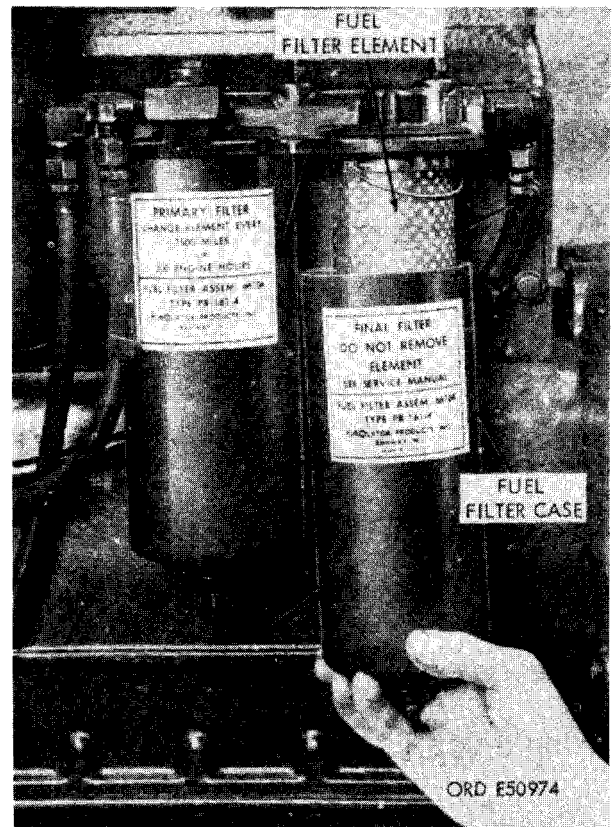
FIGURE 104. REMOVING OR INSTALLING FUEL FILTER ELEMENT AND FUEL FILTER CASE.
