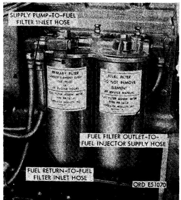
FIGURE 226. DISCONNECTING FUEL HOSES AT FUEL FILTER ASSEMBLY.
