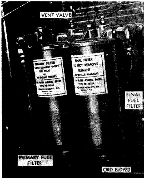
FIGURE 103. PRIMARY AND FINAL FUEL FILTERS - INSTALLED VIEW.
