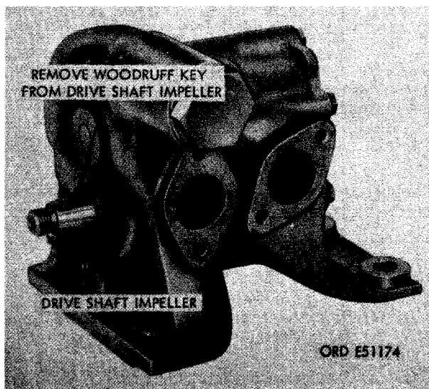
FIGURE 361. REMOVING OR INSTALLING DRIVE SHAFT IMPELLER WOODRUFF KEY.
