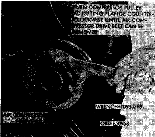
FIGURE 81. LOOSENING OR TIGHTENING COMPRESSOR PULLEY ADJUSTING FLANGE.
