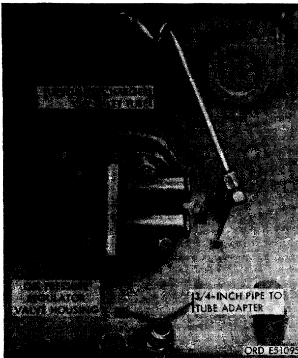
FIGURE 253. REMOVING TURBOSUPERCHARGER OIL INLET TUBE, FITTINGS, AND OIL PRESSURE REGULATOR VALVE HOUSING ATTACHING PARTS (EARLY MODEL ENGINES).
