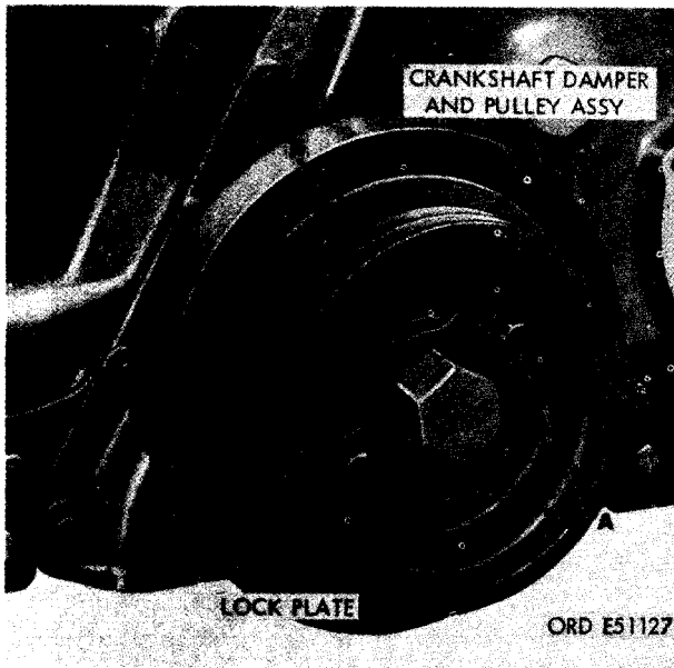
FIGURE 286. REMOVING OR INSTALLING CRANKSHAFT BOLT LOCK PLATE.
