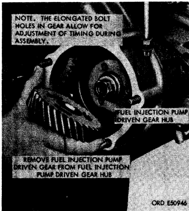
FIGURE 67. REMOVING OR INSTALLING FUEL INJECTION PUMP DRIVEN GEAR.
