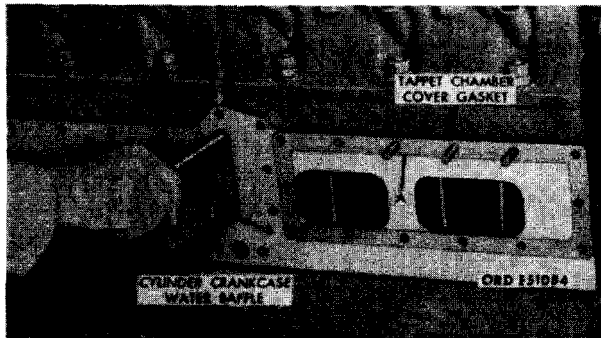
FIGURE 240. REMOVING OR INSTALLING CYLINDER AND CRANKCASE WATER BAFFLE.
