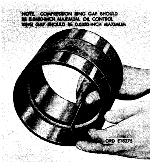
FIGURE 345. MEASURING PISTON RING GAP USING PISTON RING COMPRESSOR - 10899159.
