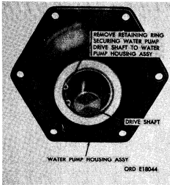
FIGURE 122. REMOVING OR INSTALLING WATER PUMP DRIVE SHAFT FROM WATER PUMP HOUSING ASSEMBLY.
