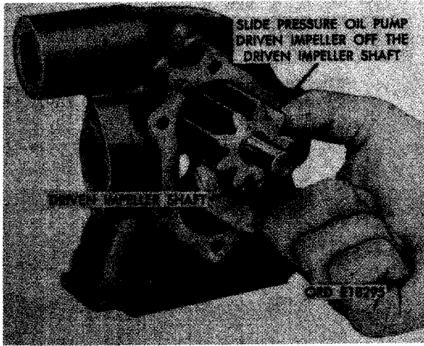
FIGURE 367. REMOVING OR INSTALLING PRESSURE OIL PUMP DRIVEN IMPELLER.
