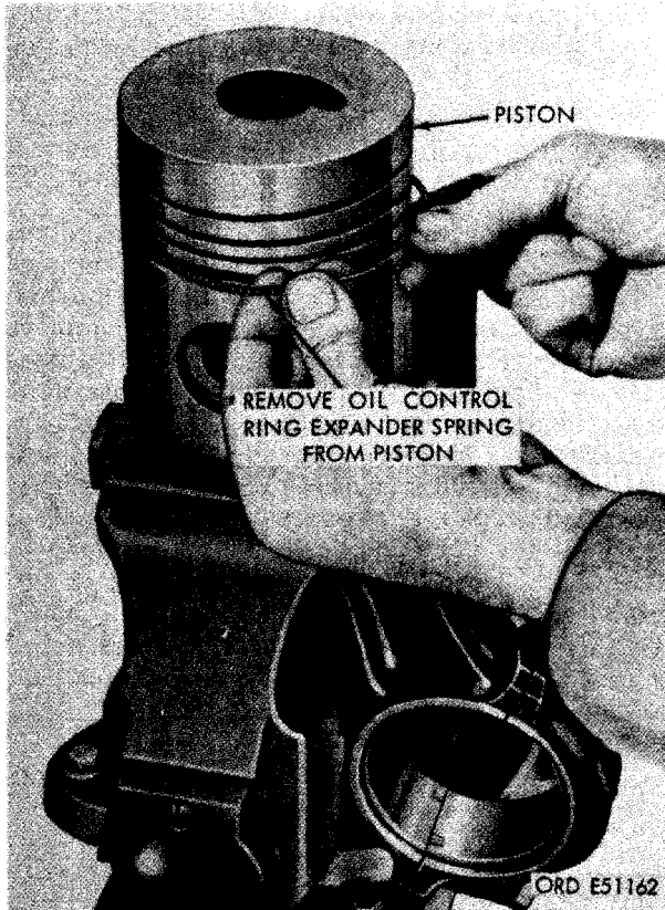
FIGURE 340. REMOVING OR INSTALLING OIL CONTROL EXPANDER SPRING.
