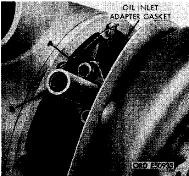
FIGURE 54. REMOVING OR INSTALLING TURBOSUPERCHARGER OIL INLET ADAPTER (EARLY MODEL ENGINES).
