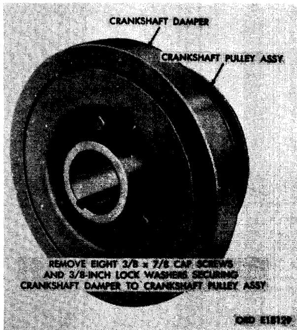
FIGURE 204. REMOVING OR INSTALLING CAP SCREWS AND LOCK WASHERS SECURING CRANKSHAFT DAMPER TO CRANKSHAFT PULLEY ASSEMBLY.
