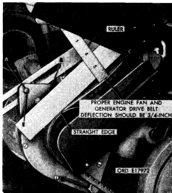
FIGURE 43. ADJUSTING ENGINE FAN AND GENERATOR DRIVE BELT DEFLECTION.
