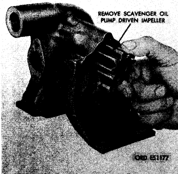
FIGURE 365. REMOVING OR INSTALLING SCAVENGER OIL PUMP DRIVEN IMPELLER.
