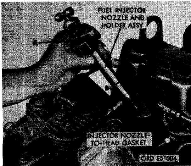
FIGURE 149. REMOVING OR INSTALLING FUEL INJECTOR NOZZLE AND HOLDER ASSEMBLY.
