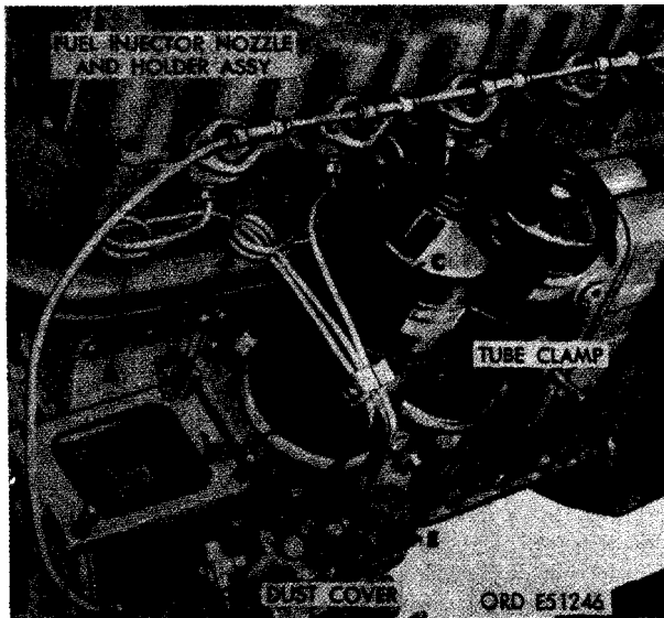
FIGURE 508. CONNECTING CYLINDER NO. 1, 2, AND 3 FUEL INJECTION TUBES.
