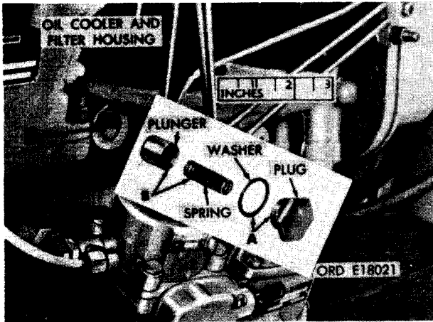
FIGURE 99. REMOVING, INSTALLING, AND INSPECTING OIL FILTER BYPASS VALVE.
