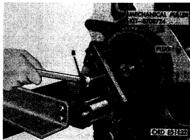
FIGURE 291. REMOVING CAMSHAFT GEAR USING MECHANICAL PULLER KIT - 8708724.
