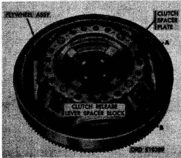
FIGURE 462. INSTALLING CLUTCH COVER ASSEMBLY AND SPACER PLATE IN FLYWHEEL.
