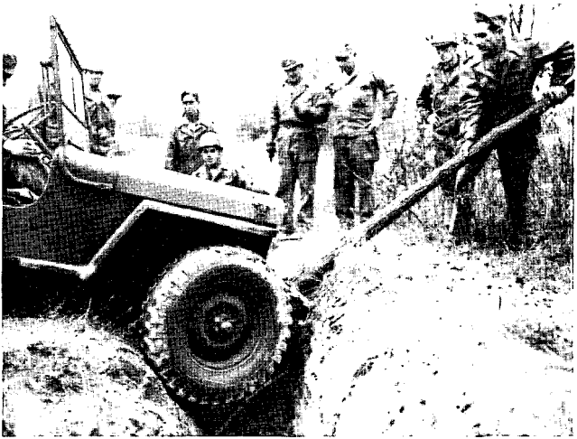
Figure 51. Pole used as a pry.
