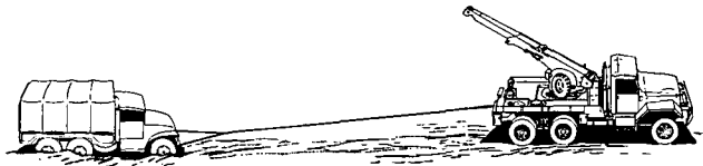
Figure 100. Recovering mired truck with a wrecker truck.
