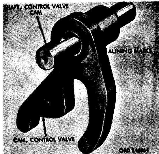
Figure 95. Control valve cam to shaft alining marks
