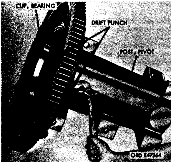
Figure 476. Removing bearing cup from base of pivot post
