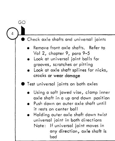
Are the axle shafts and universal joints OK?
