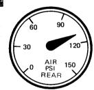
Registers air pressure (in psi) in the rear brake system. Normal operating range is 105-120 psi.
