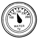
Registers engine coolant temperature in degrees Fahrenheit (normal range is 165°-195°F).
