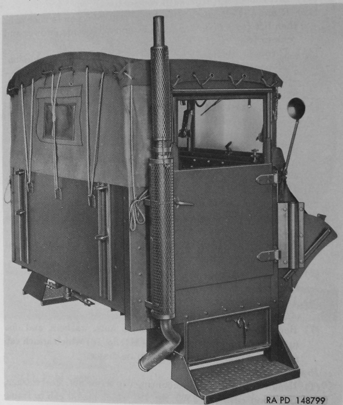
Figure 20. Cab assembly removed.
