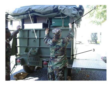
Remove corner ramp struts (1) and stow in back ramp.
