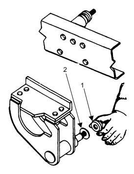
Resintall shock absorber (1), outer bushings (2), washers and nuts (3) to mounting hardware.
