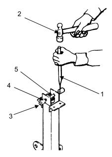
Remove bevel gear pin (1) from shaft (2).
