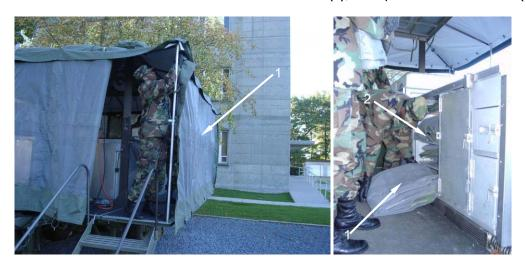
Remove overhead lights (1) and stow in area beneath burner racks (2).
