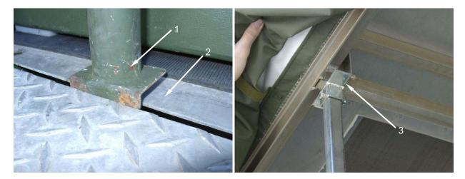
Before lowering the roof, ensure that nothing stowed inside the kitchen is higher than the top of the field ranges. With one person at each jack (1), raise both jacks slightly and disengage the corner post locking stops (2). Carefully lower both ends of the roof at the same time. Return roof lowering jacks (1) to storage by placing them upright in space on both sides of movable cabinet.
