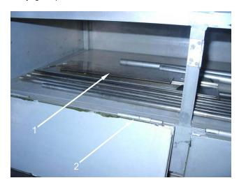
Stow optional empty lanterns, fuel can spouts, and fire extinguishers in movable cabinet assembly (1).
