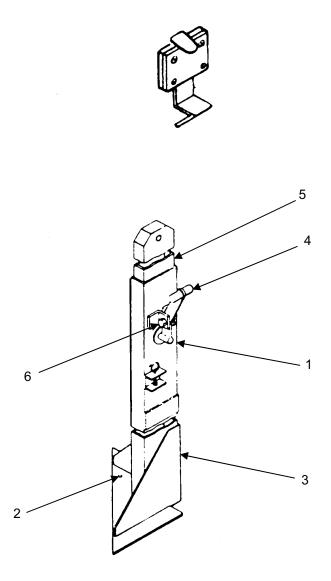
Remove nut, bolt and washer (1).
