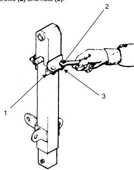
Reinstall base (1), screw and nut (2) on column.
