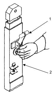
Reinstall nut, bolt and washer (1).
