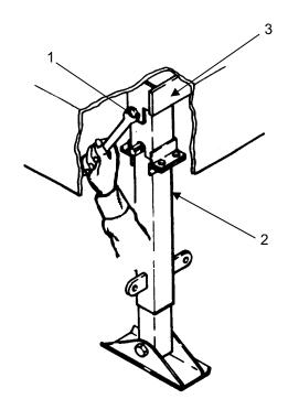
Remove nut, screw (1), and base (2) from column (3).
