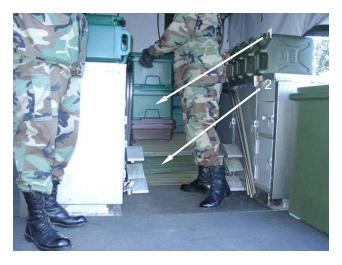
Move the ice chest (1) back into position at the end of the center aisle against the base of the ladders (2) and flush with the edge of the cabinets (3). Make sure that the handle (4) of the ice chest (1) is well behind the hole (5) used to stabilize the base of the roof jack so that the ice chest does not hinder the use of the roof jack in any way.
