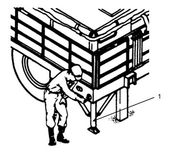
Remove quick-release pin (1) connecting jack brace (2) and leveling jack assembly (3).
