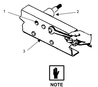
To prevent plate binding, tighten bolts evenly.
