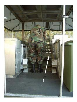
Position the moveable cabinet into the center aisle flush with the burner racks and food warmers.
