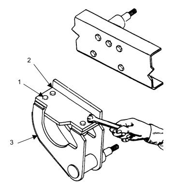
Remove five bolts, washers (1), and bracket assembly (2) from trailer frame (3).
