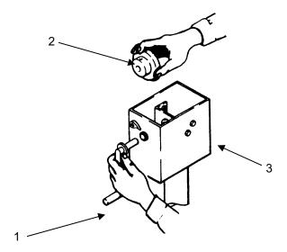
Reinstall spring pin (1) thru gear (2) and handle (3).
