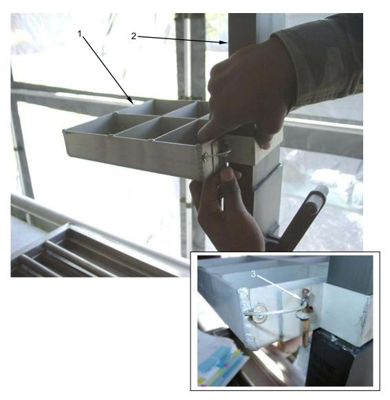
Install can opener adapter (1) in bracket (2) on top right-hand corner of storage cabinet (3). Install can opener (4) into can opener adapter (1).
