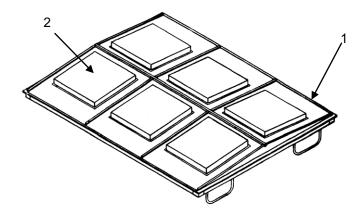
The roof assembly (1) for the MKT-90, MKT-95, and MKT-99 has a non-skid walkway (2), a rub pad (3), and side to side reinforcing cross beams and braces (4).
