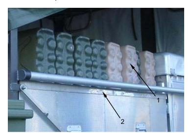
Stack twelve insulated food containers (1) on top of the ladders (2) in the center aisle.
