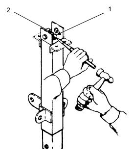
Reinstall shaft (1) and both bevel gears (2).
