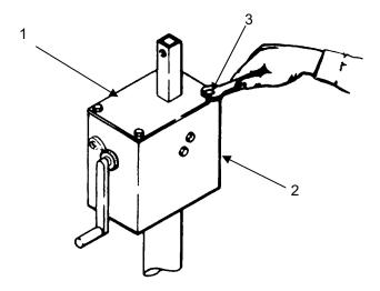
Reinstall end column (top bracket) (1) to column with screw, washer, and nut (2).
