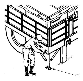
Remove quick-release pin (1) connecting jack brace (2) to leveling jack assembly (3).
