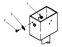
Removal/Reinstallation of leadscrew (1) from column (2).
