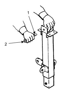
Remove pin and washer (1) from leadscrew (3).
