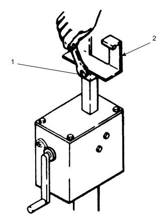
Remove four nuts, screws (1) and plate (2) from housing (3).
