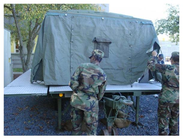
Push the slide-lock pins (1) into place, locking the corner ramp assemblies (2) to the end assembly (3). Repeat for the rear end ramp.
