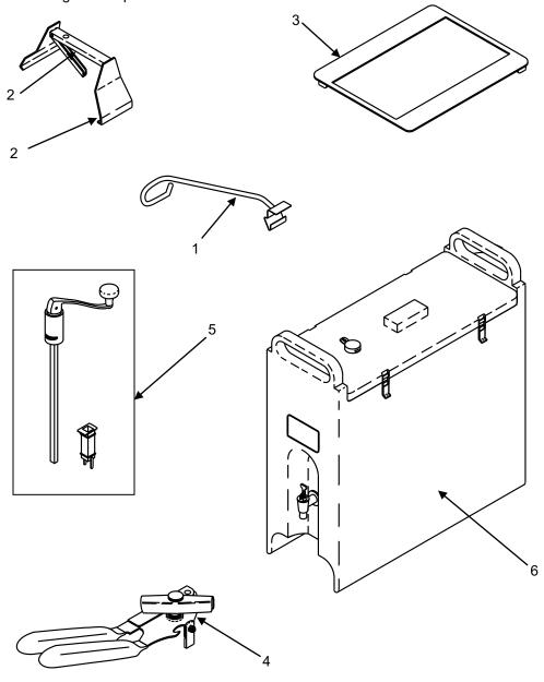
**MKT-I IMPROVEMENT KIT.** An improvement kit has been made available that will permit the Unit to replace and therefore upgrade many of the components included in older models of the Mobile Kitchen Trailer.
