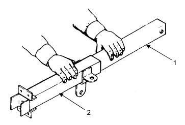
Reinstall pin and washer (1) on leadscrew (2).
