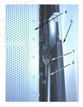
Route the strap (1) over the water containers (2) and engage one end of the strap on the bracket (3) on the floor beneath the drop leaf tables and attach the opposite end to similar bracket on the floor by the outer range cabinet. Tighten strap with ratcheting mechanism (4). Install second strap over liquid dispensers on opposite side of kitchen and secure strap.
