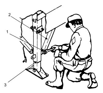
Remove nut, washer and screw (1) connecting leveling jack assembly (2) to platform assembly (3).
