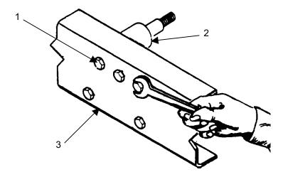
Reinstall five bolts, washers (1) and bracket assembly (2) to trailer frame (3).
