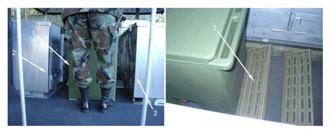
Stack remaining two ladders (1) on top of and in exactly the same position (i.e. base pads up) as the first ladder.
