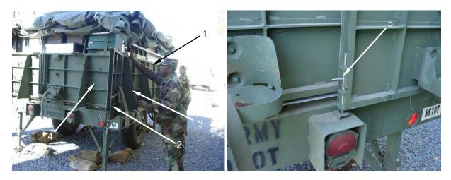
Place corner ramp struts (1) in holder (2) on rear end ramp (3).
