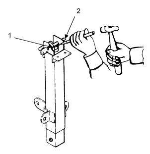
Reinstall pins and knobs on shaft.
