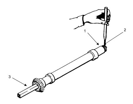
Reinstall gear shaft (1) into housing (2).
