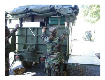
Secure front and rear end ramps (1) with eye bolt latches or z-bar (2). Fold in braces (3).
