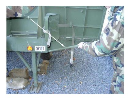
Raise side (1) and corner ramp (2) assemblies, fold in side ramp braces (3), fold corner ramps (2) around end ramps (4), and secure assemblies with slide lock pins (5).
