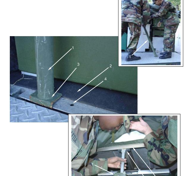
Place locking stops (1) into holes near bottom of the inside tube of posts (2) when roof is in raised position. Make sure that all four locking stops (1) are engaged. Collapse roof jacks (3) and stow in a secure place.
