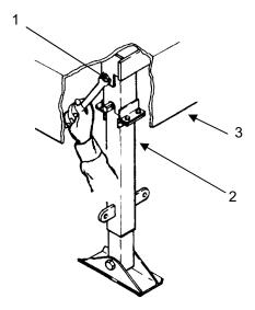
Reinstall screw, washer and nut (1) connecting stabilizer arm (2) to leveling jack assembly (3).
