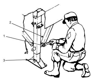
Remove nut, washer, and screw (1) connecting leveling jack assembly (2) to platform assembly (3).
