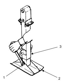
Remove nuts, screws (1) and housing (2).
