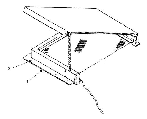
REPAIR ROOF VENT AND SCREEN ASSEMBLY KITCHENS WITH 6 ROOF VENT ASSEMBLIES
