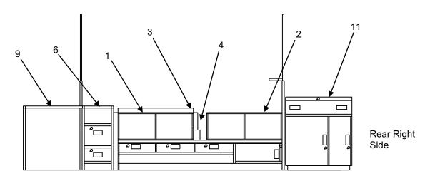
In the travel configuration, the roof canopy (1) is stowed and the travel cover (2) is secured around the exterior of the unit. Gasoline cans (3) are secured to the rear of the trailer (4). For the open configuration, the travel cover (2) is rolled and secured. The roof canopy (1) is attached to tent poles (5). For the foul weather configuration, the side walls are attached to the roof canopy (1) and secured to the trailer (4) for Kitchen tentage configurations (open, travel, or foul weather).
