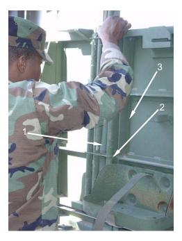
Secure the stowed equipment in the center aisle with aisle strap assembly (1).
