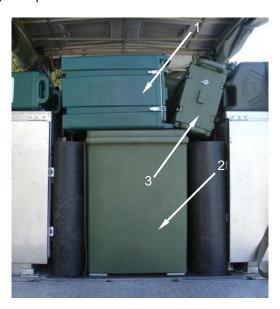
Pass one end of the cabinet strap (1) through the bracket (2) between the field ranges (3) and fixed cabinet (4).
