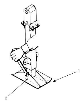
Reinstall screw, washer and nut (1) connecting leveling jack assembly (2) to platform assembly (3).
