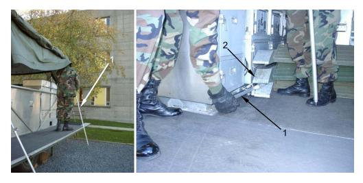
Stow ladder handrails (1) on the left and right side of the ladder (2) leaning against the fronts of the cabinets (3).
