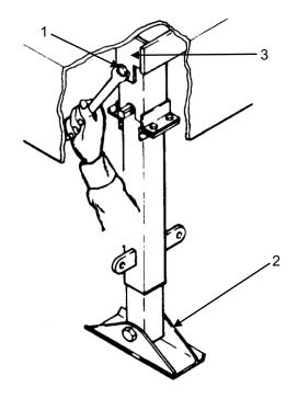
Reinstall screw, washer, and nut (1) connecting stabilizer arm (2) to leveling jack assembly (3).
