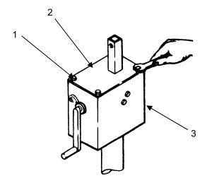
Remove spring pin (1) from gear (2) and handle (3).
