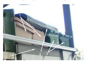
Stack the water containers (1) along the top of the cabinets (2) on the right side of the kitchen. Orient the tops of the water containers so that they face the center aisle.
