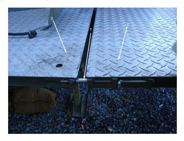
Soldiers may stand on ramp to continue with the next procedure. Position a soldier on either end of the ramp and roll the travel cover (1) under so that water will not collect in the fabric roll (2). Start at the bottom, fold the corners in and roll the cover (1) away from you until you reach the top. Secure the roll-up travel cover (1) with the straps (3) provided. Make sure all shock cords (4) are rolled inside of the covers. Repeat for the remaining three sides of the MKT.
