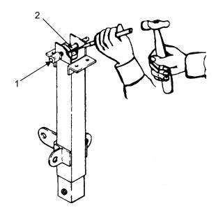
Remove shaft (1) and both bevel gears (2).
