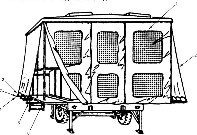
Open the screens (1) and the covers at the rear of the kitchen to allow use of the serving line entrance and exit, as well as the cook's access to the center aisle.
