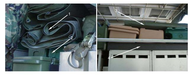
Place field tables (1) on top of the cold weather skirt (2) and insulated food containers in the center aisle.
