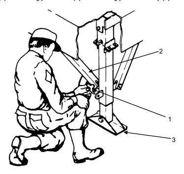
Remove nut, washer and screw (1) connecting stabilizer arm (2) to leveling jack assembly (3).
