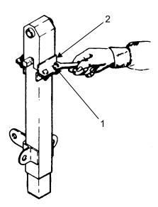
Using punch (1) and hammer (2), remove pin (3) and knob (4) from shaft (5).
