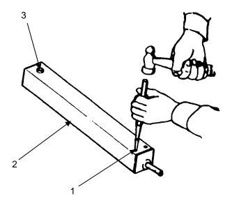
Reinstall nut (1) in column (2) with two pins (3).
