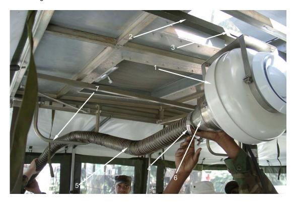
If the heater vent weldment (1) is not already installed, slide the heater vent weldment (1) under the cabinets (2) on the right side of the MKT so that the end of the weldment (1) that accepts the exhaust hose (3) is flush with the end of the cabinet (2).
