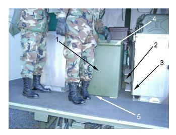
Place three liquid dispensers (1) on top of the ice chest (2) with the tops facing in toward the center aisle. Place one liquid dispenser (3) on top of the ice chest but off to the side.
