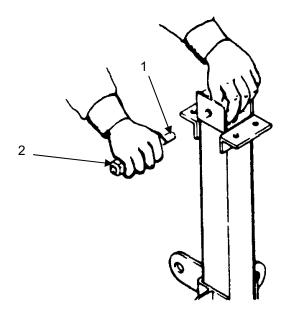
Reinstall bevel gear pin (1) in shaft (2).
