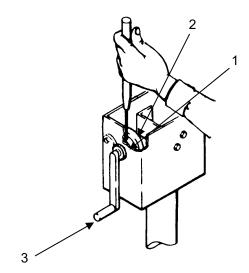
Reinstall plate (1) to housing (2) with four screws, washers and nuts (3).
