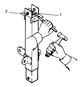
Remove support column assembly (1) from column (2) by sliding off.
