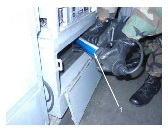
Loosen hose clamps and disconnect exhaust fan hose from heater weldment and from the hose adapter on the exhaust fan (1). Be sure to leave the heater weldment in place. Remove exhaust fan from roof and stow all components in storage area beneath burner racks (2).
