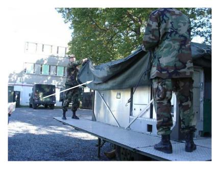
Unlock corner ramp slide lock pins (1).
