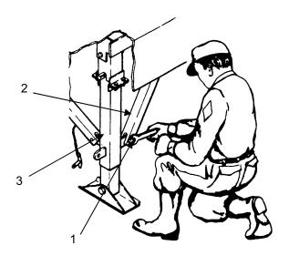
Reinstall quick-release pin (1) connecting jack brace to leveling jack assembly (2).
