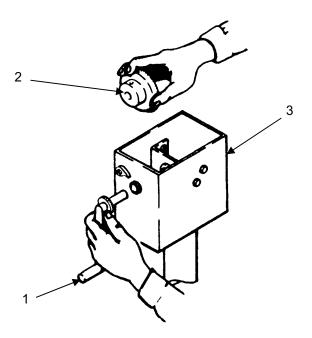
Remove four screws (1) and bracket (2) from housing (3).
