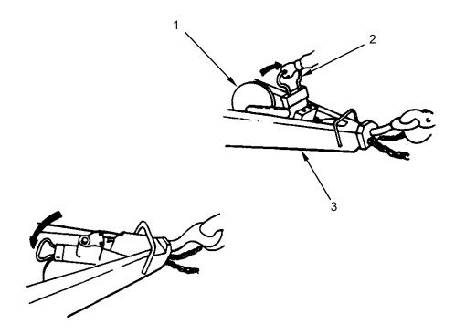
Disconnect the electrical power cord (1) and air brake hose (2). Set one of the manual brakes (3). Disconnect safety chains (4).
