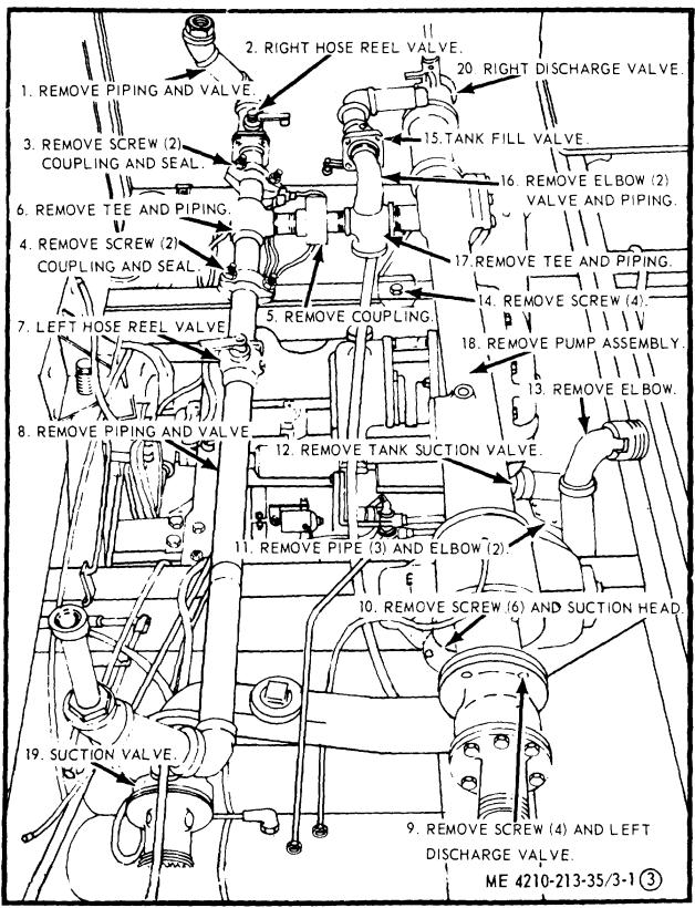
NOTE: REMOVE SUCTION AND RIGHT DISCHARGE VALVES IN A SIMILAR MANNER.
