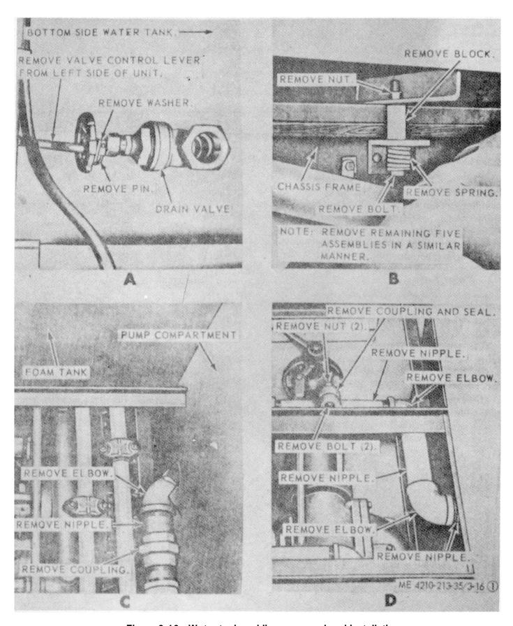
Figure 3-16. Water tank and lines, removal and installation.
