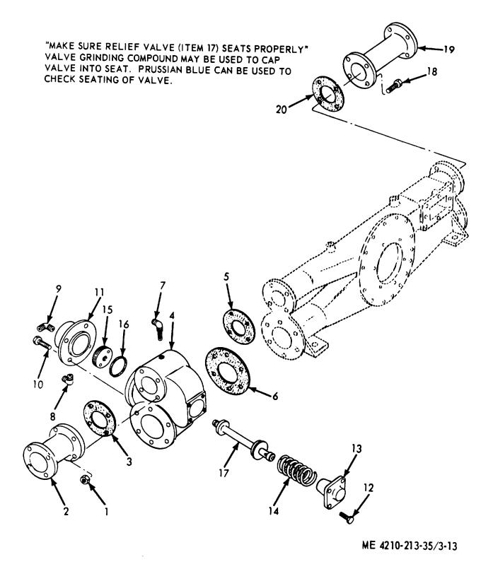
Figure 3-13. Relief valve and adapter, exploded view.
