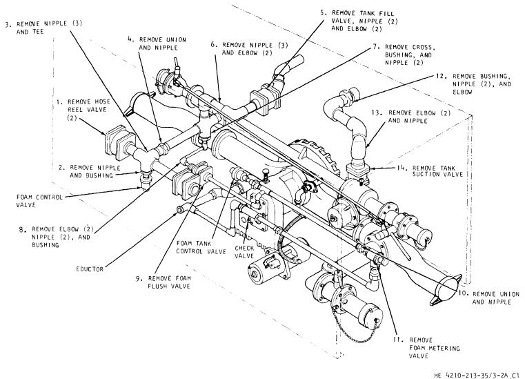
Figure 3-2A. Hose real valves, tank fill valve, tank suction valve, and foam metering valve removal and installation for model FT 500.
