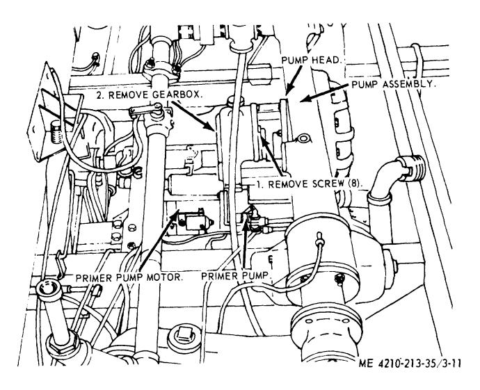
Figure 3-11. Pump gearbox, removal and installation.
