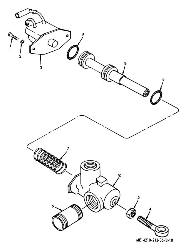
Figure 3-10. Primer valve, exploded view.
