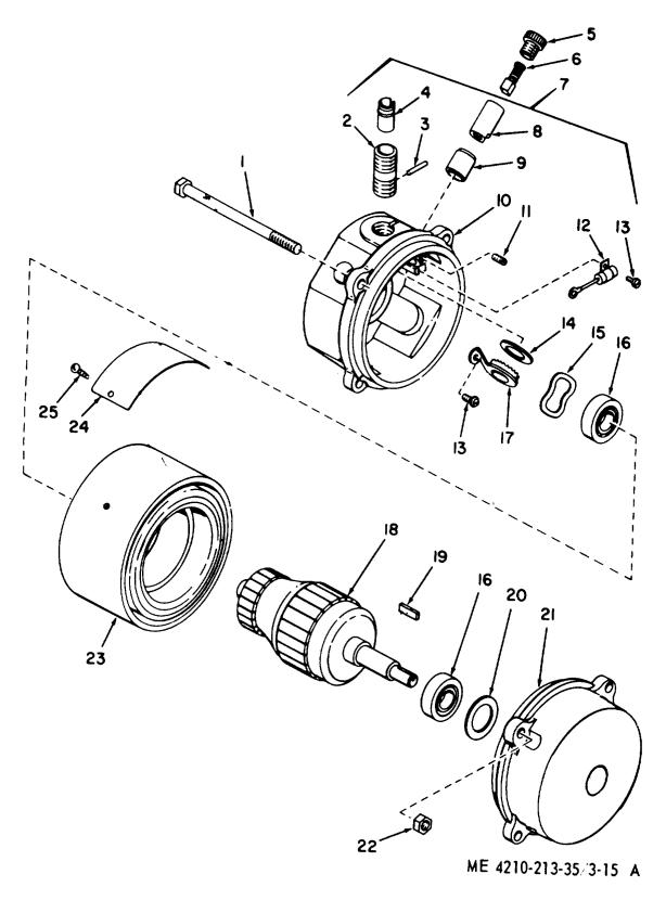
Figure 3-15A. Hose reel motor, exploded view.
