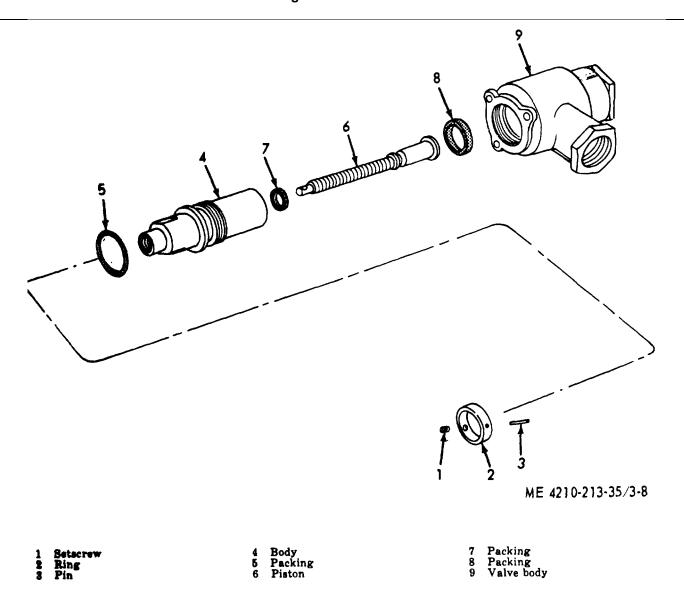
Figure 3-8. Foam metering valve, exploded view.
