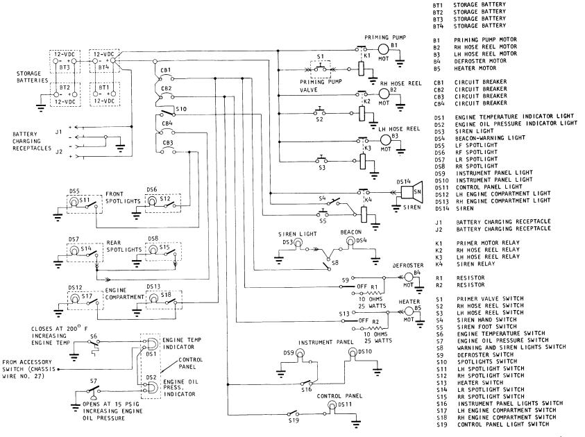
Figure 1-2. Wiring diagram for model FT-500.
