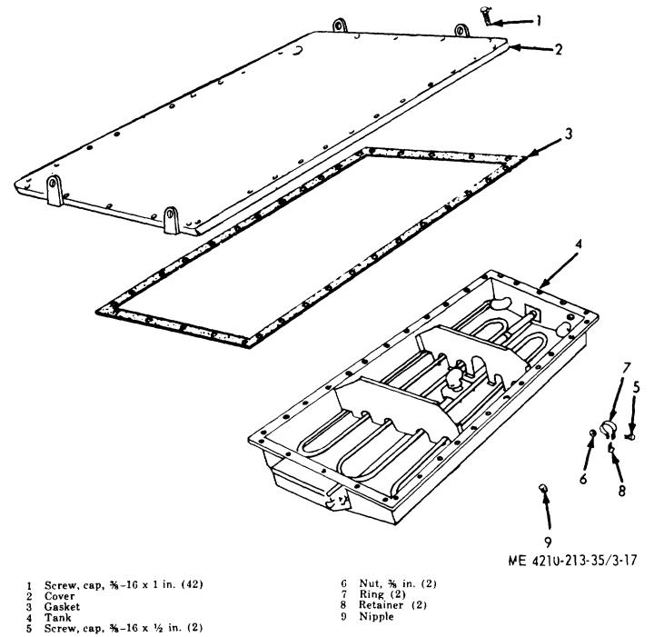
Figure 3-17. Water tank, exploded view.
