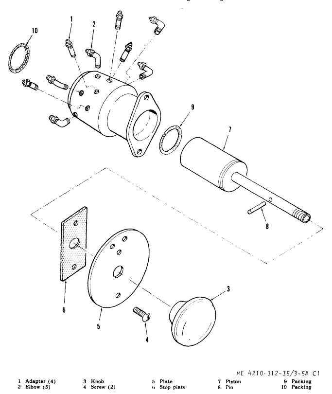
Figure 3-5A. Drain line valve for model FT-500, exploded view.
