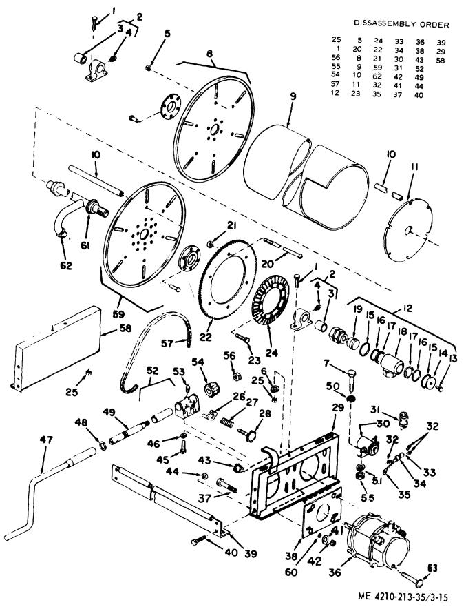
Figure 3-15. Hose reel assembly, exploded view.
