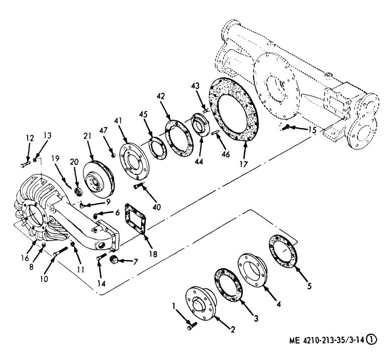
Figure 3-14. Pump head and body, exploded view.
