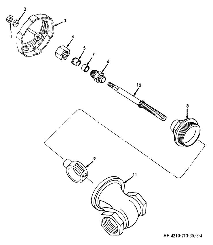
Figure 3-4. Water- tank drain valve, exploded view.
