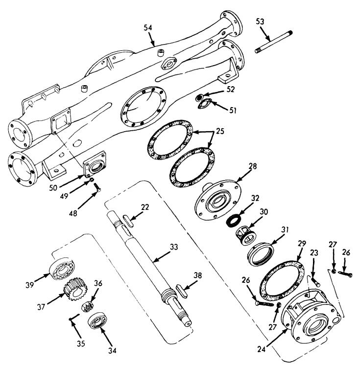
NOTE: REMOVE PARTS 24 THRU 39 ASSEMBLED, THEN DISASSEMBLE.
