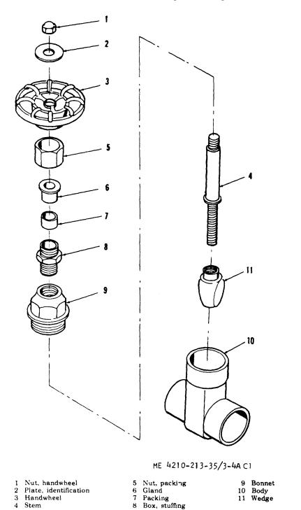
Figure 3-4A. Water tank drain valve for model FT-500, exploded view.
