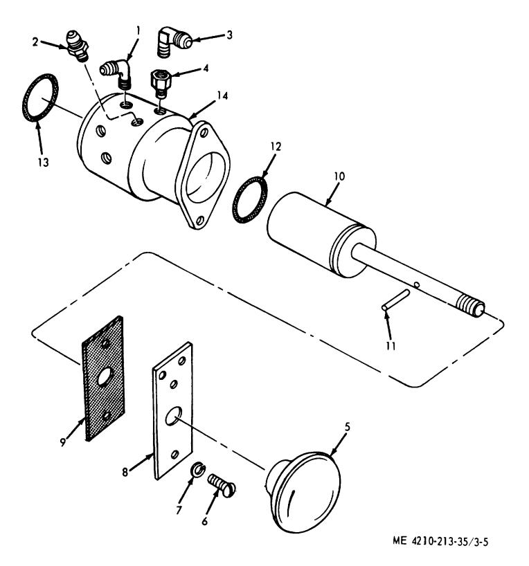
Figure 3-5. Drain line valve, exploded view.
