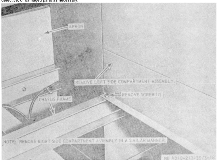
Figure 3-18. Special purpose body compartments, removal and installation.
