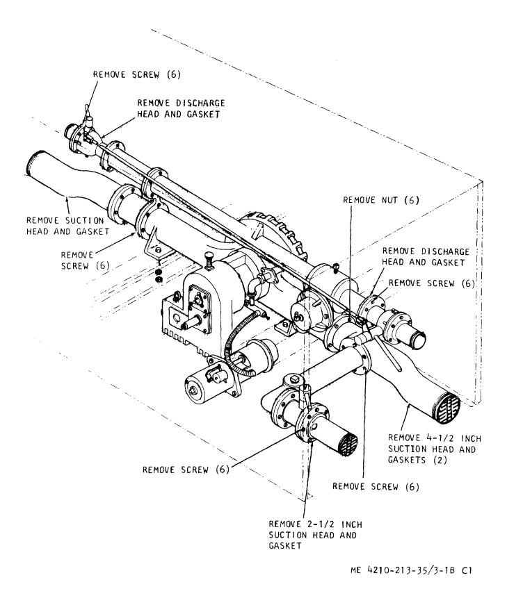
Figure 3-1B. Suction and discharge values, removal and installation for model FT-500.
