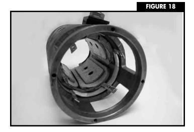
Press the CE housing flush with the field ring.
