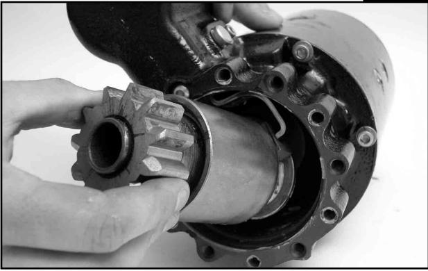
On MC MD and ME models, insert a finger in the shift housing and pull back the top of the shift lever, then perform the same sequence as above.
