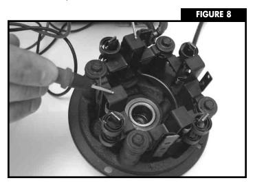
11. Brush Holder Assembly Ground Test
