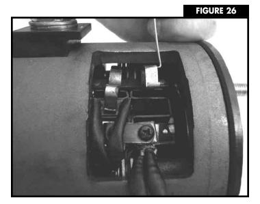
14.3 Wrap the brush opening band around the four brush openings in the position of the paint line, and secure with two #10-32 screws.
